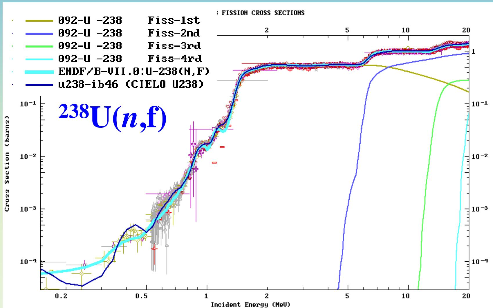
$^{238}\text{U}(n,f) - \text{ib46} = \text{ENDF-B/VII.1=STD}$
