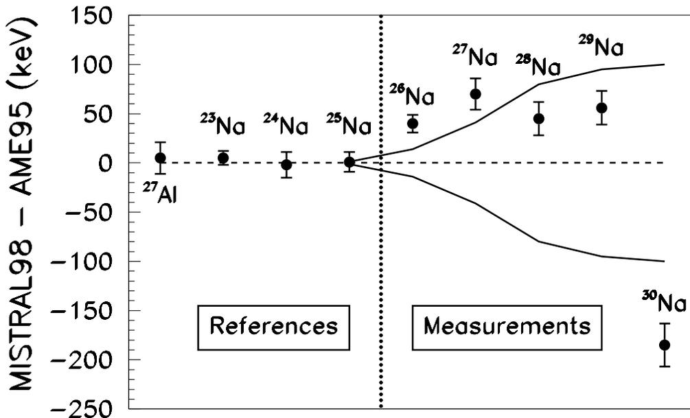
Fig. 1. The MISTRAL results compared to the AME'95 for <sup>27</sup>Al and for the sodium isotopes from  $A = 23$  to 30. The zero line represents the values from the mass table and the two continuous symmetrical lines represent the table uncertainties.
