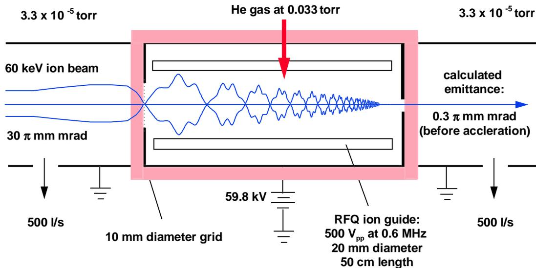
**FIGURE 1.** Schematic diagram of beam cooling system with optimized design parameters indicated.
