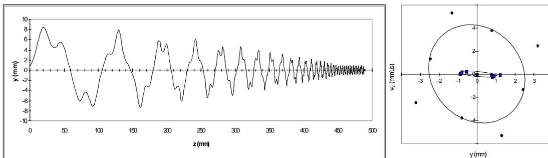
**Figure 3.** (left) Simulated trajectory of a single ion with an axial energy of 130 eV and a transverse energy of 8.5 eV subject to buffer gas cooling at 0.033 torr in a quadrupole ion guide. (right) Transverse phase space diagrams (for one dimension) of the ion beam before and after transit through the ion guide. The ratio of the corresponding emittance is a factor of 100. Ion guide operating parameters are as in figure 1.
