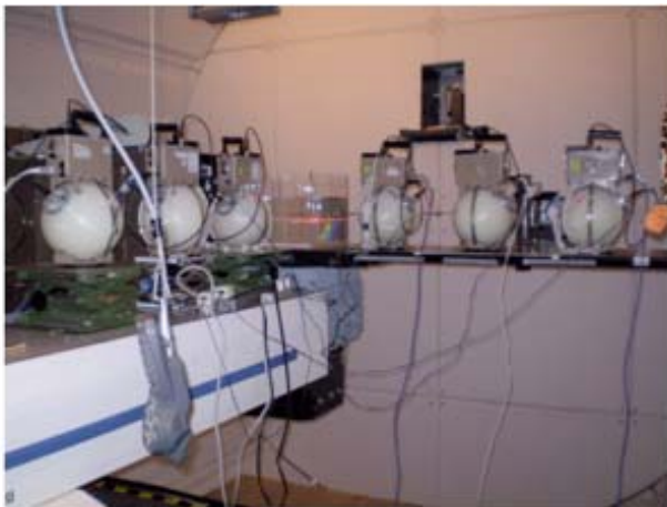
Fig. 8: Arrangement of the Bonner sphere detectors in the treatment rom. The beam nozzle is seen on the right side in the pictures.
