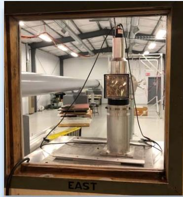
$\text{C}_6\text{D}_6$  Detector (45m)
