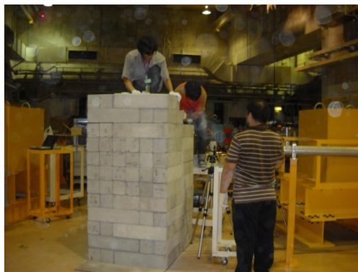
**Concrete shielding experiment** at heavy ion accelerator (HIMAC)
