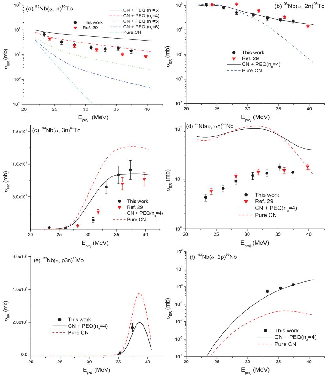
FIG. 1: (Colour online) Experimentally measured and theoretically calculated excitation functions for evaporation residues produced in the  $\alpha + {}^{93}\text{Nb}$  reaction using the code ALICE-91.
