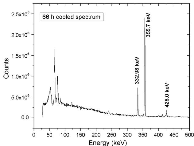
**Fig. 3** Typical  $\gamma$ -ray spectrum from the activated  $^{197}\text{Au}$  foil with 10 MeV bremsstrahlung beam
