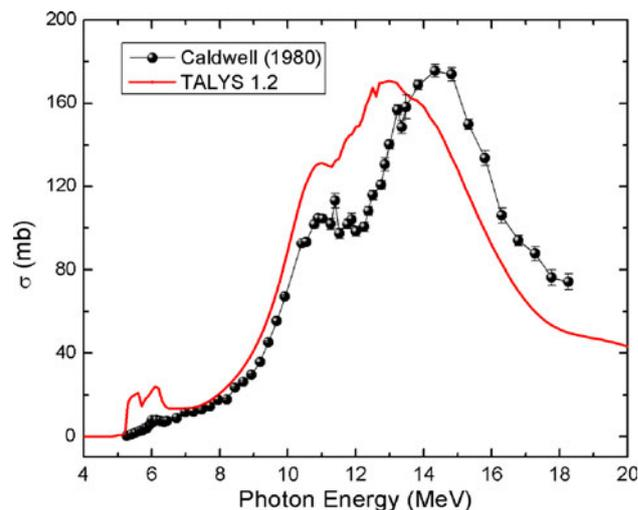
**Fig. 5** Plot of experimental and theoretical  $^{238}\text{U}(\gamma, f)$  reaction cross-section as a function of photon energy
