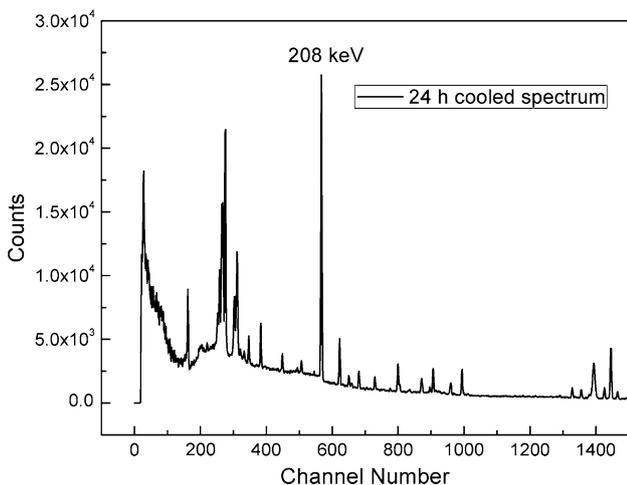
**Fig. 2** Typical  $\gamma$ -ray spectrum from the activated  $^{238}\text{U}$  foil with 10 MeV bremsstrahlung beam
