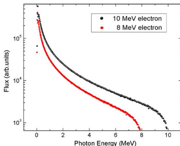
**Fig. 4** Bremsstrahlung spectrum obtained by impinging electrons of 8 and 10 MeV energies
