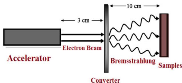
**Fig. 1** The experimental arrangement of irradiation
