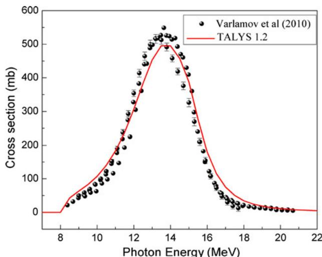
**Fig. 6** Plot of experimental and theoretical  $^{197}\text{Au}(\gamma, n)^{196}\text{Au}$  reaction cross-section as a function of photon energy
