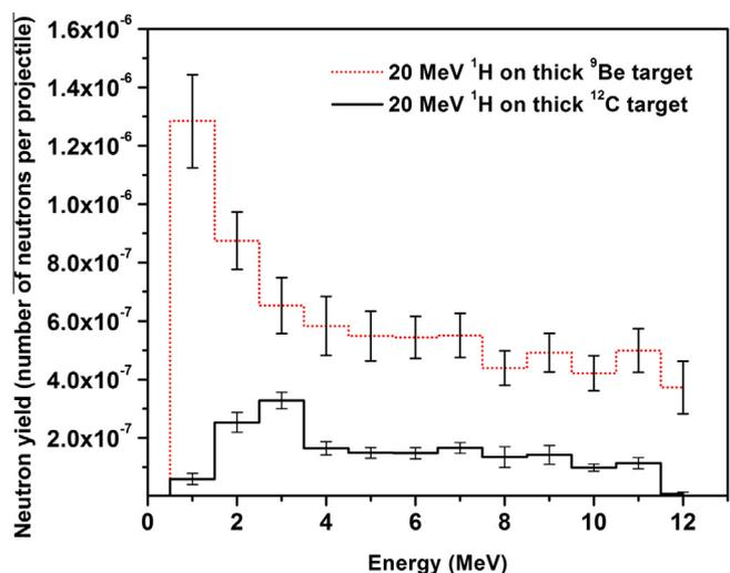
**Fig. 3.** Neutron spectral yield (total number of neutrons per projectile) for  $^1\text{H} + ^9\text{Be}$  and  $^1\text{H} + ^{12}\text{C}$  reactions at 20 MeV proton energy. The spectra are generated by measurement of track parameters in CR-39 detectors using the image analysing program autoTRAK\_n.
