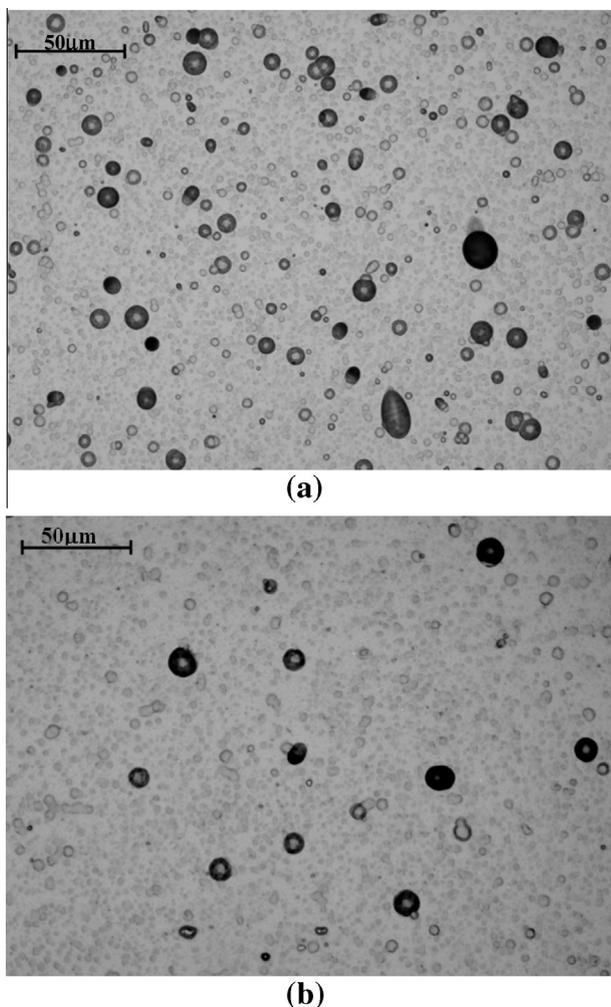
**Fig. 1.** Recoil tracks in CR-39 detectors due to neutrons emitting from (a)  $^1\text{H} + ^9\text{Be}$  and (b)  $^1\text{H} + ^{12}\text{C}$  reactions at 20 MeV proton energy. The tracks are developed by chemical etching (6.25 N NaOH, 70 °C, 9 h) and imaged at an optical magnification of 200 $\times$ .
