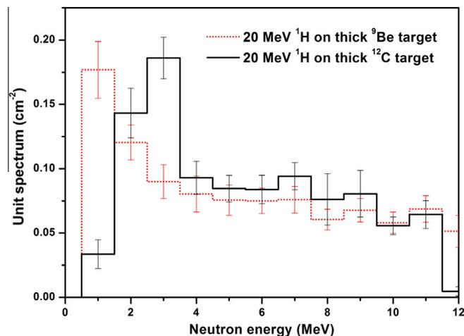
**Fig. 2.** The unit neutron spectra from  $^1\text{H} + ^9\text{Be}$  and  $^1\text{H} + ^{12}\text{C}$  reactions at 20 MeV proton energy, generated by measurement of track parameters in CR-39 detectors and using the image analysing program autoTRAK\_n for the analysis of 2-dimensional track images.
