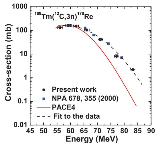
FIG. 1. (Color online) The experimentally measured and theoretically calculated EFs for reaction  $^{169}\text{Tm}(^{12}\text{C},3n)^{178}\text{Re}$  using Monte Carlo-based code PACE4. The measured cross sections for the residues  $^{178}\text{Re}$  by Chakrabarty *et al.* [12] are also shown for comparison.
