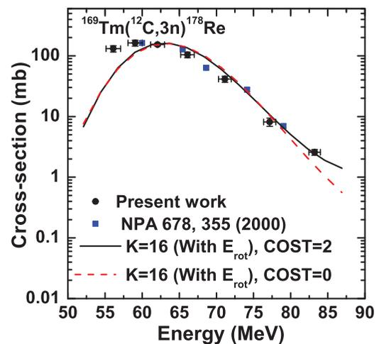
FIG. 5. (Color online) The experimentally measured and theoretically calculated EFs for reaction  $^{169}\text{Tm}(^{12}\text{C},3n)^{178}\text{Re}$  using code ALICE-91. The effects of different values of mean free multiplier COST = 0 and COST = 2 in ALICE-91 calculations are shown in this figure and discussed in the text. The measured cross sections for the residues  $^{178}\text{Re}$  by Chakrabarty *et al.* [12] are also shown for comparison.
