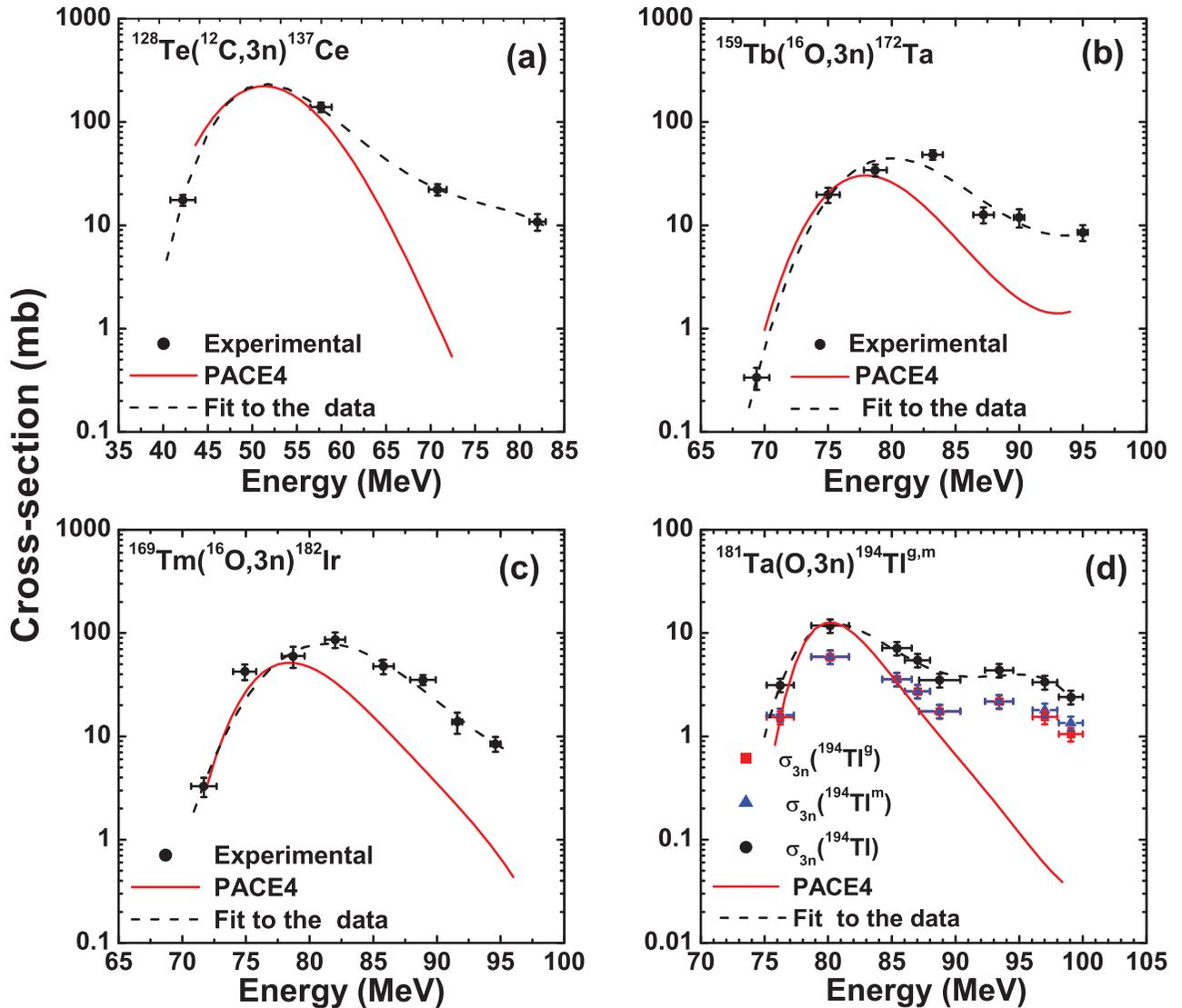
FIG. 2. (Color online) The experimentally measured and theoretically calculated EFs for reactions  $^{128}\text{Te}(^{12}\text{C},3n)^{137}\text{Ce}$ ,  $^{159}\text{Tb}(^{16}\text{O},3n)^{172}\text{Ta}$ ,  $^{169}\text{Tm}(^{16}\text{O},3n)^{182}\text{Ir}$ , and  $^{181}\text{Ta}(^{16}\text{O},3n)^{194}\text{Tl}$  using Monte Carlo-based code PACE4. The parameters used in this calculations are discussed in the text.
