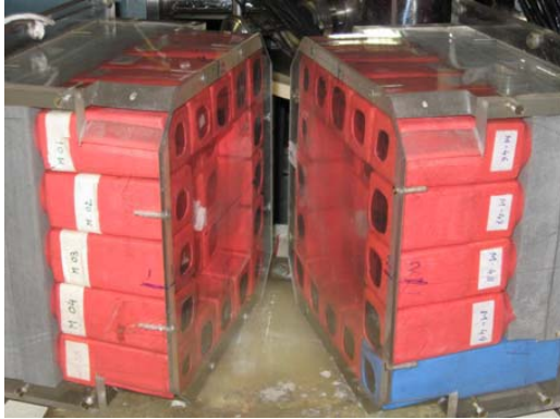
Fig. 1 : The TAGS set up at VECC using BaF2 scintillator detectors. The 50 detector elements were arranged in two halves each consisting of 25 detectors in the staggered castle type geometry. The two halves are shown in the figure separately.
