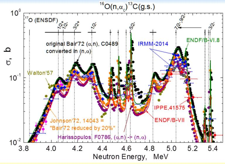
neutron measurements,  $^{16}O(n,\alpha)^{13}C$ , are less accurate and have worse resolution than alpha ones,  $^{13}C(\alpha,n)^{16}O$ , which can be converted in  $^{16}O(n,\alpha)^{13}C$  (below En = 5.6 MeV)
