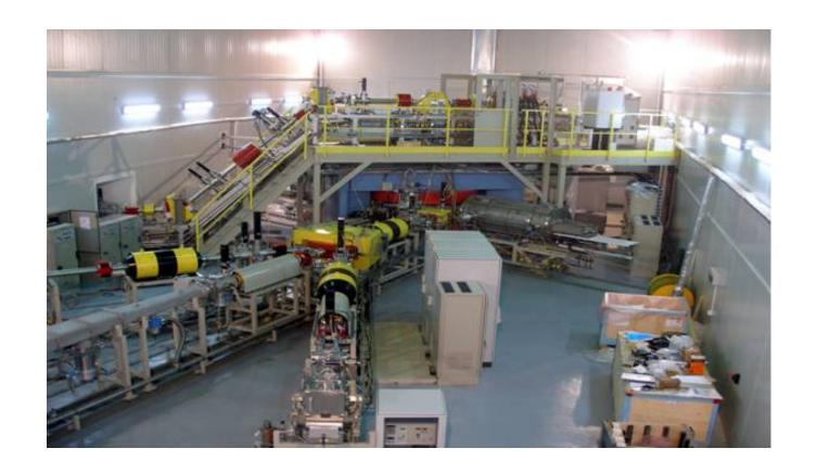
The one of the main components of cyclotron is source of multicharge of heavy ions on basis of electron-cyclotron resonance (ECR). It can work as a heavy ion injector in cyclotron for generating ion beams with high energy as well as on autonomous regime ensuring the experiments on beams with low energy.
