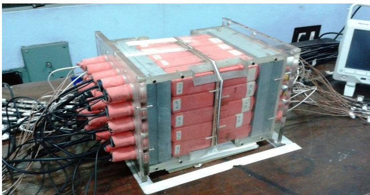
Fig.4.1.1: The TAGS setup used for the present measurement. The catcher foil is placed in the middle between the two halves
