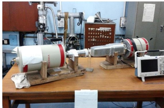
Fig.4.2.1: The HRS setup with single-crystal HPGe and clover HPGe detectors. The foil was placed in between the two detectors.
