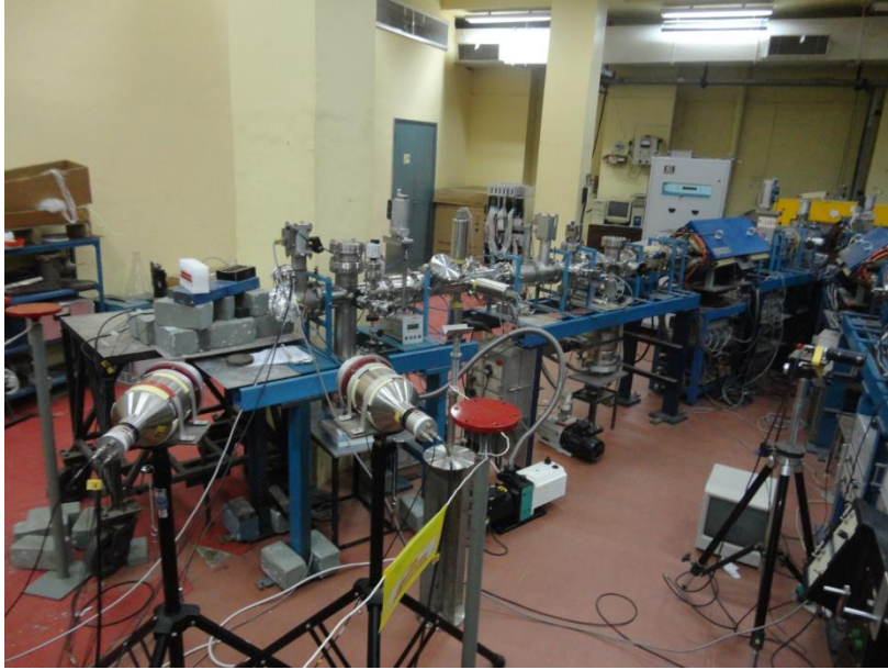
25 degree Hill-Side Beam Line being developed for inverse Kinematics {}^7\text{Li} beam on proton
