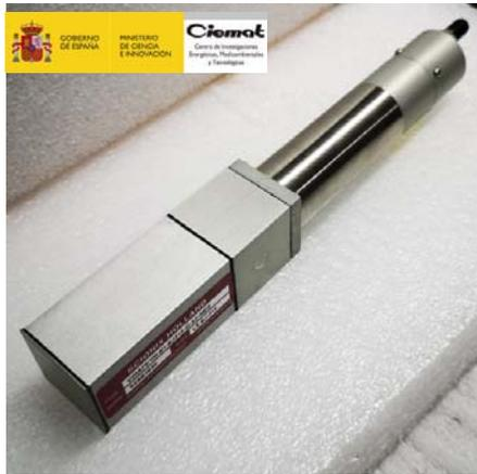
**sTED**  $\gamma$ -ray detector for very high counting rates (3 MBq) and suppression of the spallation flash (conditions at EAR2)
