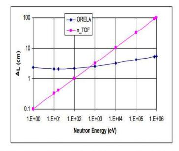
Due to moderation the neutron flight path is energy dependent.
