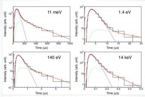
The resolution function was obtained by simulating neutron pulse shapes with a Monte-Carlo simulation code, PHITS.
