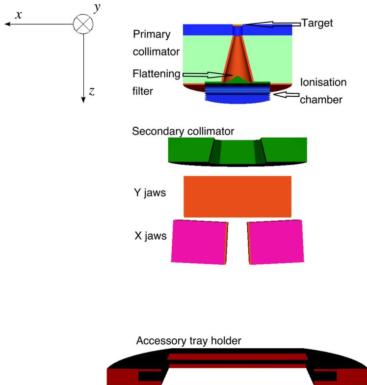
Figure 1. 3D image of the Varian Clinac 600 C in which a sector has been excluded in order to show the inner structure of the linac. The reference system is shown with the origin displaced to aid the eye visualise the direction of the three axes.
