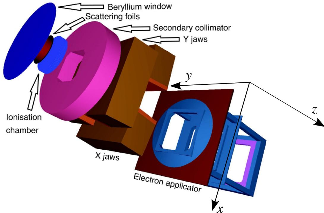
Figure 6. 3D image of the Varian Clinac 2100 C/D operating in electron mode at 6 MeV. The 15x15 cm<sup>2</sup> electron applicator is also shown. The reference system is shown with the origin displaced to aid the eye visualise the direction of the three axes.
