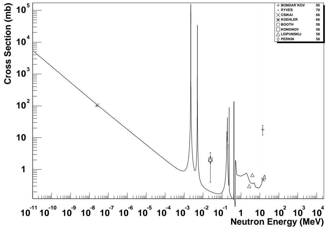
2.25     $^{30}\text{Si} (\text{n},\gamma) ^{31}\text{Si}$
