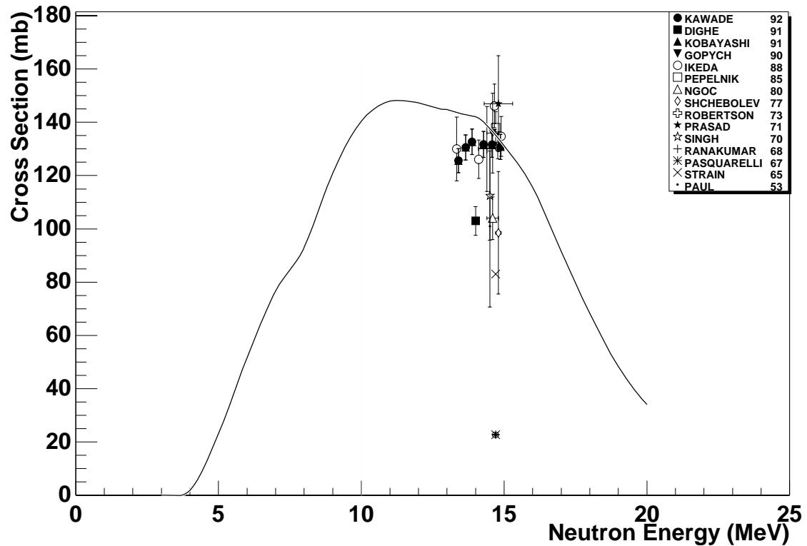
2.21      $^{29}\text{Si} (\text{n},\text{p}) ^{29}\text{Al}$
