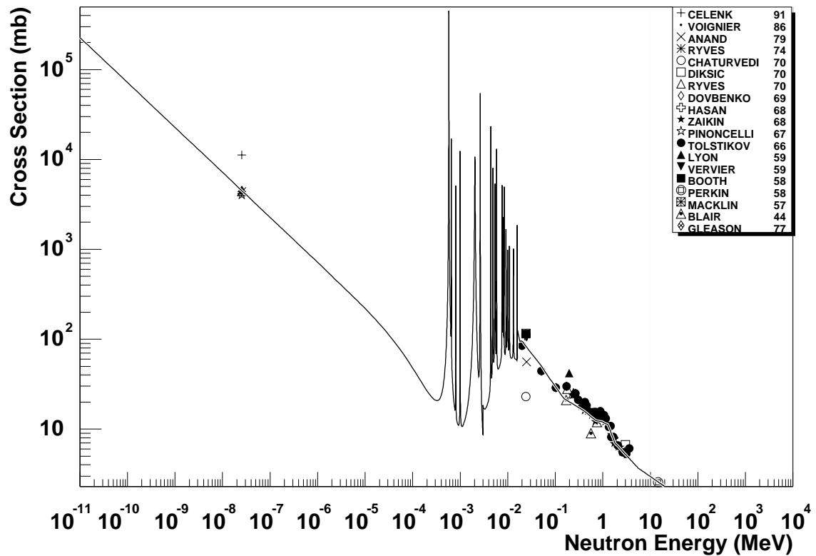
2.97      $^{63}\text{Cu} (n,\gamma) ^{64}\text{Cu}$
