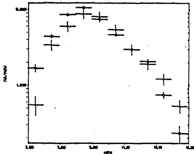
Fig. 1. The angle integrated α-emission cross-section for the <sup>56</sup>Fe(n,α) reaction
