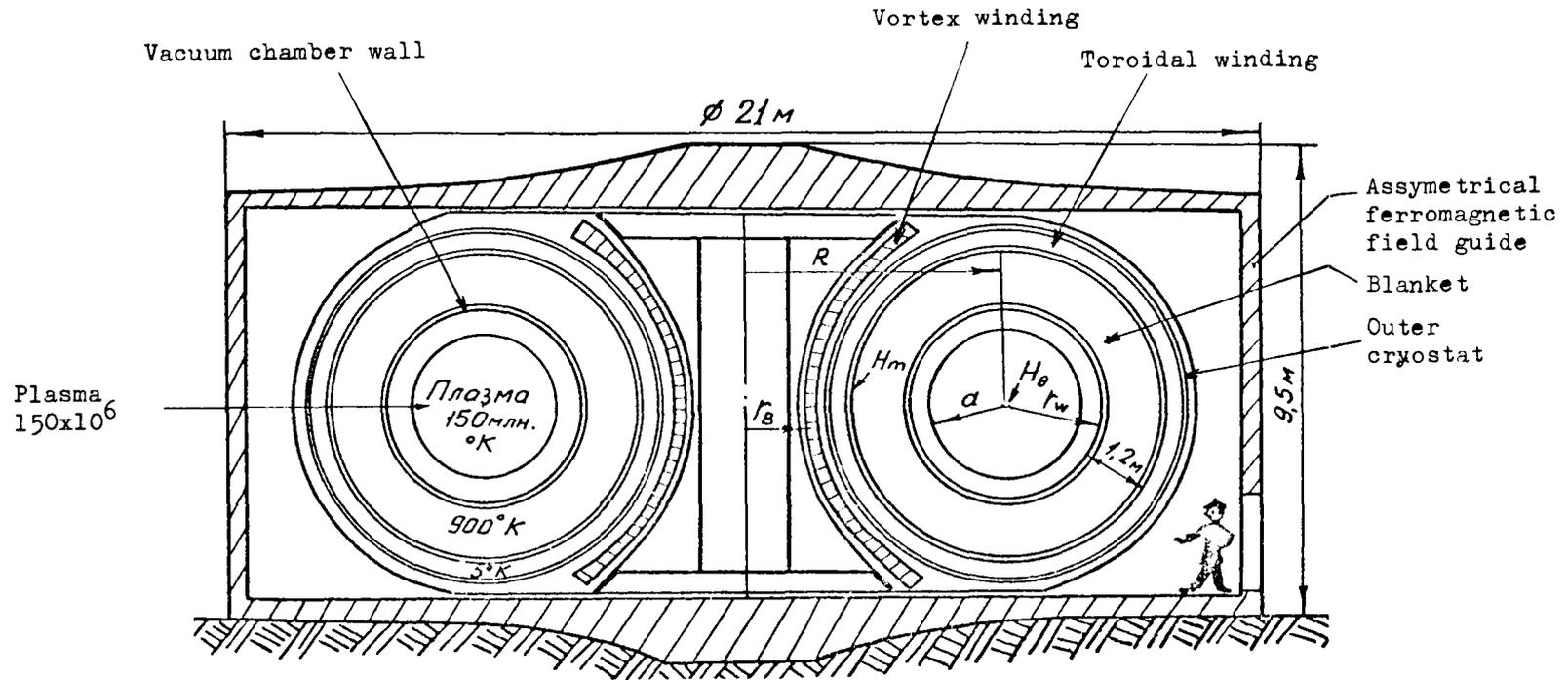
Fig. 1. Sectional view of the 2 million kW(e) Tokamak reactor
