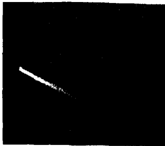
Figure 3 The display outputs of the pulse shape discriminator equipment, the horizontal axis being proportional to the pulse height and vertical axis to the pulse shape discrimination. (a) the total pulse output from a ^{252}\text{Cf} fission source (b) and (c) the neutron and gamma ray output channels gated by all the required biases.
