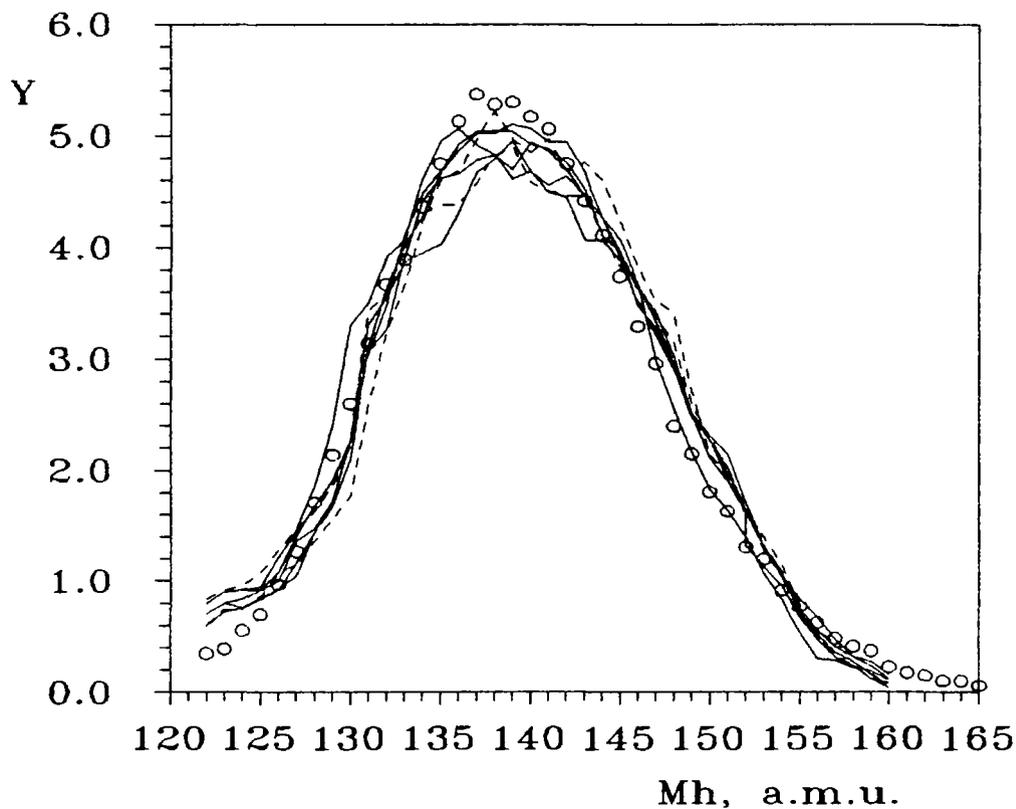
Fig.1. Set of FF mass-distributions of  $^{243}\text{Am}$  for different  $E_n$ .
