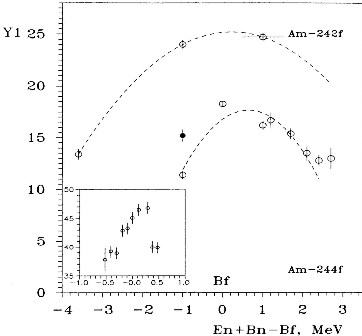
Fig.4. Energy dependence of Standard-I contribution (in % normalized to 100) to the mass spectrum of  $^{242}\text{Am}$  and  $^{244}\text{Am}$  fissile systems. Data for  $^{241}\text{Am}(d,pf)$  [7] were averaged over  $(d,pf)$ -excitation function in the region, indicated in [7]. The black sign - [1]. Insert shows  $Y_1$  for  $^{237}\text{Np}(n,f)$  [10] in the same variables as for mane figure. Barrier parameters were derived from [9].
