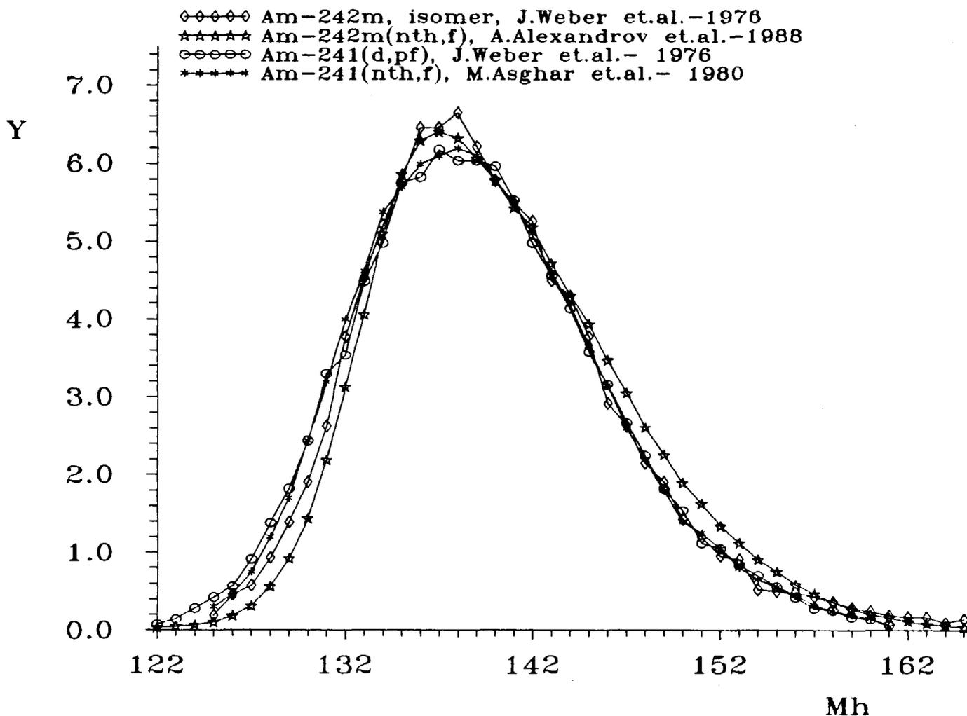
Fig.3. Fission fragment mass distributions for reactions:  $^{242m}\text{Am}(sf)$  [7],  $^{242m}\text{Am}(nth,f)$  [8],  $^{241}\text{Am}(d,pf)$  [7], and  $^{241}\text{Am}(nth,f)$  [2].
