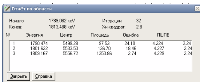
Fig. 3.25. Examples of automatic (a) and interactive (b) processing of a 2.6 GeV proton-irradiated ^{93}\text{Nb} spectral range, spectrum No. 10.
