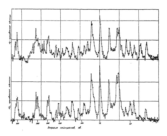
Fig. 3. Yields of secondary fission neutrons (N  $_f)$  and  $\gamma$  rays (N  $_\gamma)$  from sample
