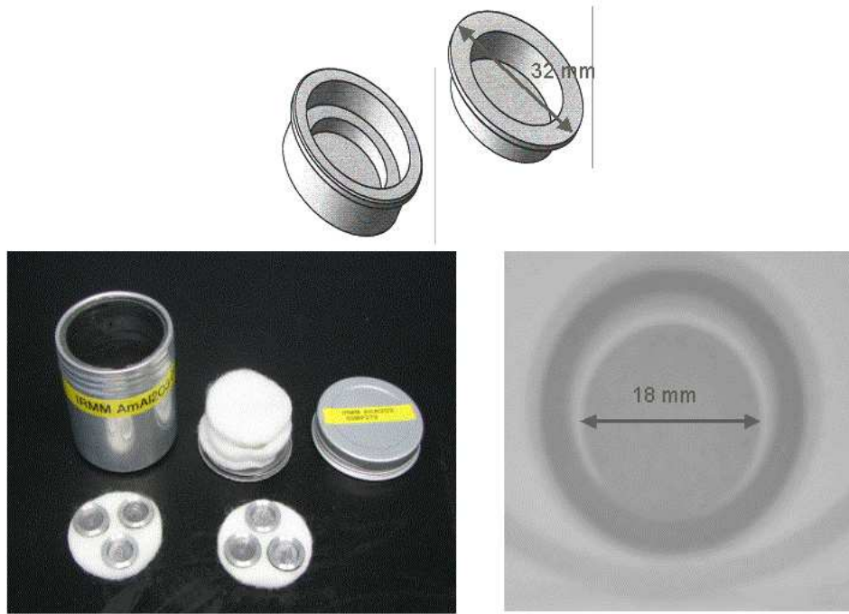
Figure 3.2: Americium samples and sample holders picture, scheme and X-ray radiograph.
