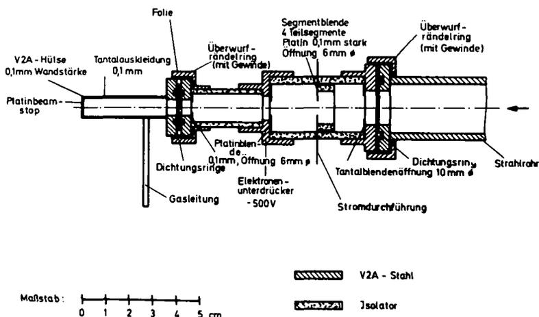
Fig. 1 Construction of the gas-target
