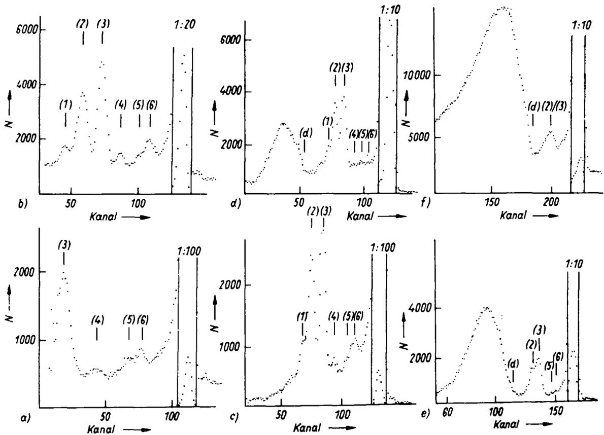
Fig. 2 Neutron time-of-flight spectra at different energies  $E_0$  ( $\theta_{\text{lab}} = 20^\circ$ ,  $p_{\text{gas}} = 1.3$  at, foil  $5.5 \mu\text{m Ta}$ ); position (d) represents the highest neutron energy from the deuteron break-up /7/. a)  $E_0 = 7$  MeV; b)  $E_0 = 8$  MeV; c)  $E_0 = 9$  MeV; d)  $E_0 = 10$  MeV; e)  $E_0 = 11$  MeV; f)  $E_0 = 12$  MeV.
