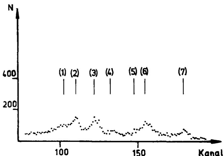
Fig. 3 Neutron time-of-flight spectrum from the target without deuterium gas; the deuteron bombarding energy corresponds to the DD-neutron energy of 8 MeV ( see fig.2,b); other conditions - as indicated on fig. 2. Number (7) gives the position of the DD-neutron peak.
