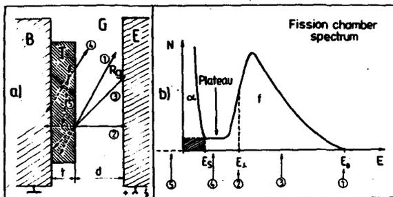
Fig.1: Various kinds of fission fragment tracks in a parallel plate fission chamber and its representation in the fission chamber spectrum (schematic view). The chamber is of a "differential" type, i.e. the target - electrode distance is smaller than the fission fragment ranges  $R_0$  in the chamber gas. Counting losses due to fragment  $\alpha$  absorption (track ⑤) as well as FC pulses in the plateau region (track ④) are caused by "flat" tracks (small inclination against the target surface).
