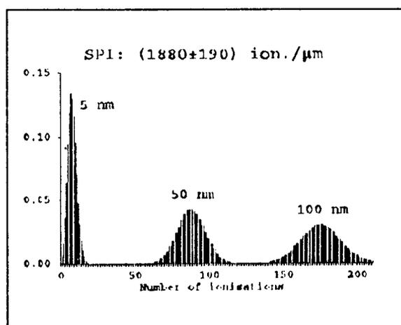
**Figure 8** Primary ionisation distributions for 4 MeV  $\alpha$ -particles for 5, 50 and 100 nm segments. SPI value by Perris and Zarris (1989).
