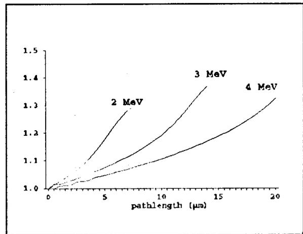
Figure 9 The ratio of the dose calculations with the energy loss correction to those based on LET for 2, 3 and 4 MeV  $\alpha$ -particles as a function of the pathlength.
