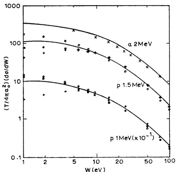
Figure 4 The model SDICS (see text) is presented (solid line) for 1MeV, 1.5MeV protons and 2MeV  $\alpha$ -particles, along with data ( $\bullet$ , Toburen and Wilson 1977;  $\times$ , Toburen et al 1980;  $+$ , Inokuti et al 1980;  $\circ$ , Rudd 1990).
