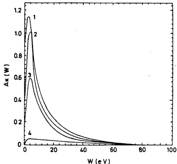
Figure 1. The terms  $A_k(W)$ ,  $k=1-4$ , of equation (2) as a function of the energy  $W$  of the ejected electron.
