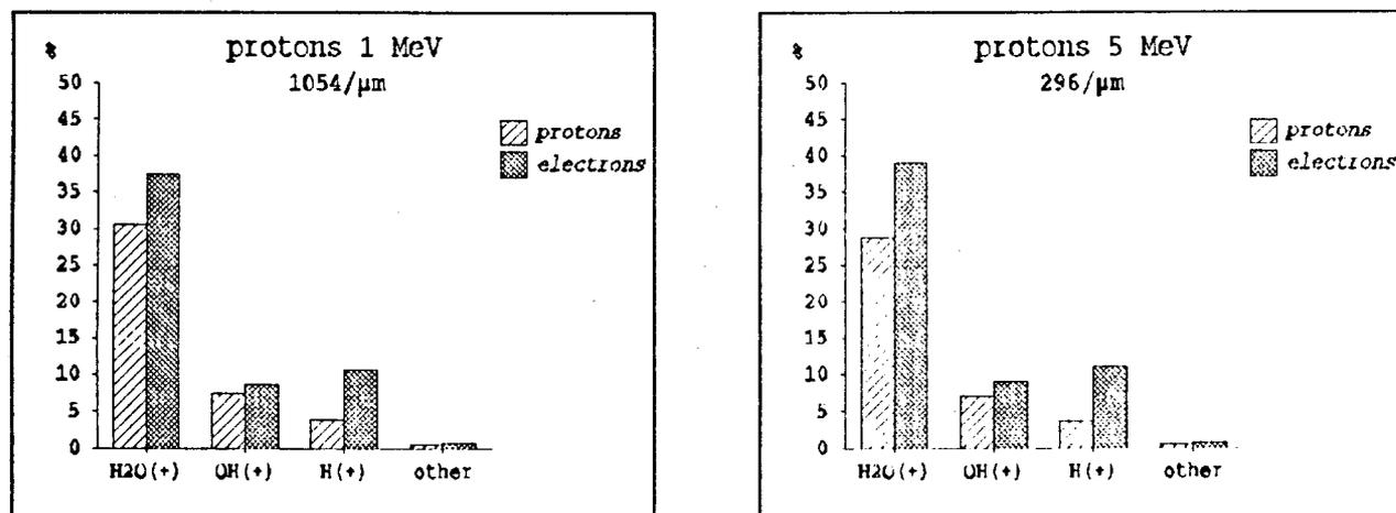
Figure 6. Primary chemical species formed by primary protons and the ejected electrons: 1 MeV protons (left), 5 MeV protons (right)
