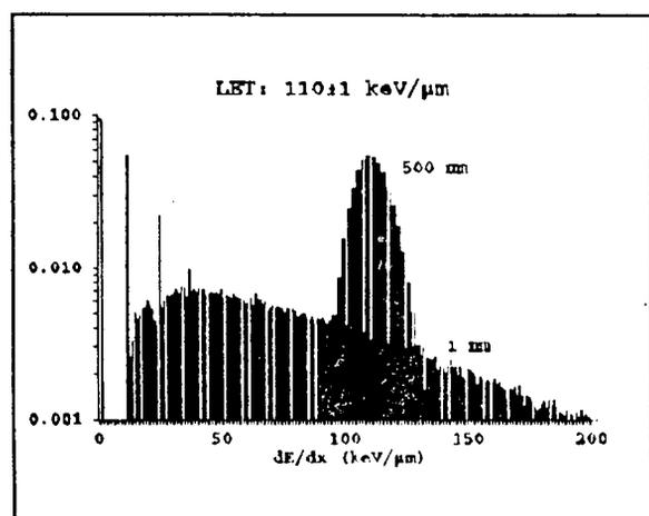
**Figure 7** Energy loss distributions ( $\text{keV}/\mu\text{m}$ ) for 4 MeV  $\alpha$ -particles for 1 and 500 nm segments. LET value by Thwaites (1981).
