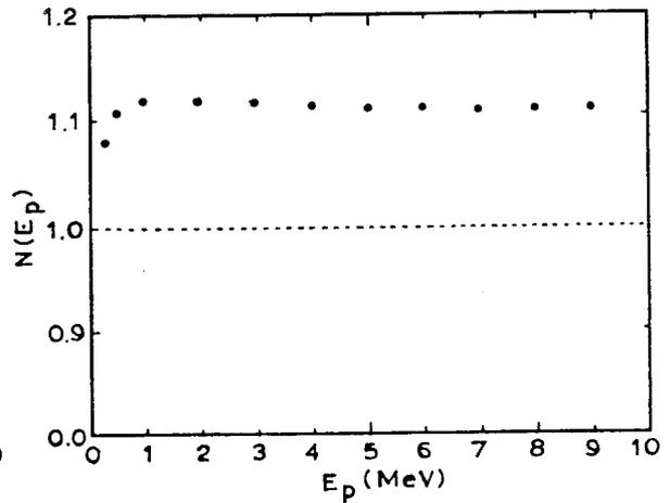
**Figure 3** Ratio  $N(E_p)$  of the experimental TICS to the integrated model calculations as a function of proton's energy  $E_p$ .
