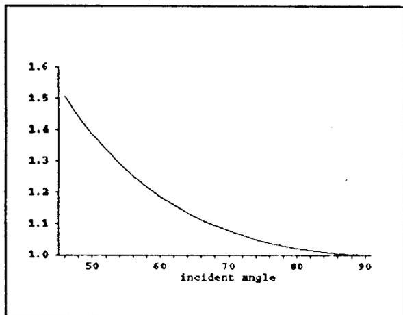
**Figure 10** Dose relative to perpendicular incidence as a function of incident angle for 4 MeV  $\alpha$ -particles on 8  $\mu$ m sample.
