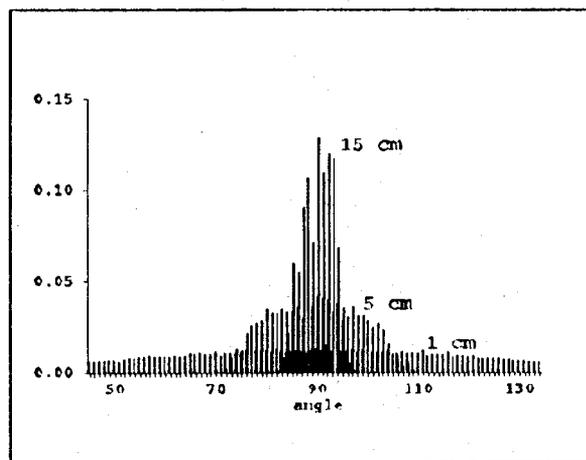
**Figure 11** Angular distribution of particles incident on a 0.4 cm radius sample placed on central axis of a surface source (1.5 cm radius) for 1, 5 and 15 cm source-sample distance.
