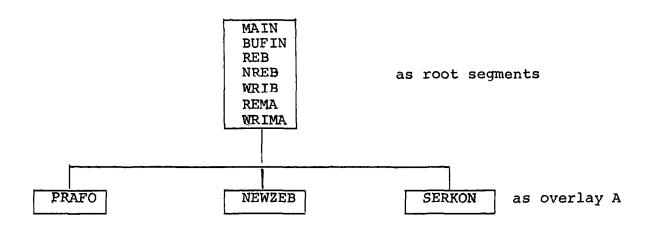
Note: PRAFO's for different evaluated files may be parallel in OVERLAY B. In this case their common routines such as, e.g. ARED, SLOV are in OVERLAY A.
