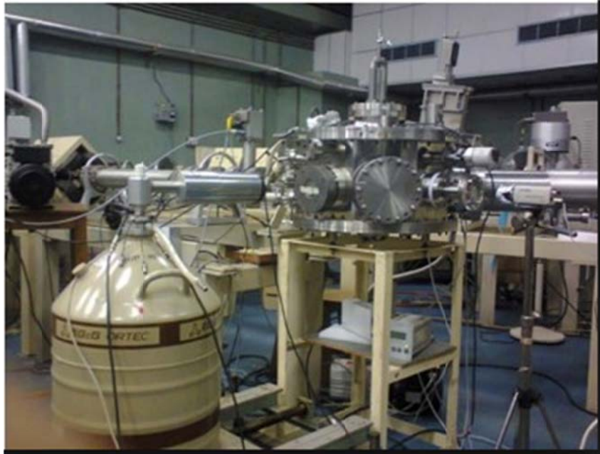
Figure 13: Scattering chamber and detectors at IOP, Bhubaneswar
