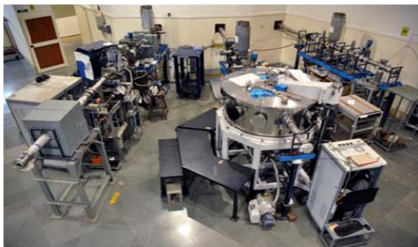
Figure 29: Hall 1 of Pelletron LINAC Facility showing general purpose scattering chamber, TIFR, Mumbai
