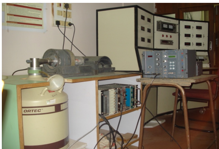
Figure 23: Control system of 14 MeV Neutron Generator along with HPGe detector and other electronic systems.
