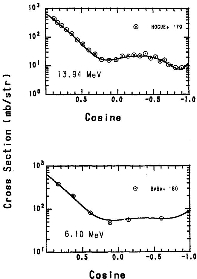
Fig. 6 Measured and evaluated elastic angular distributions.
