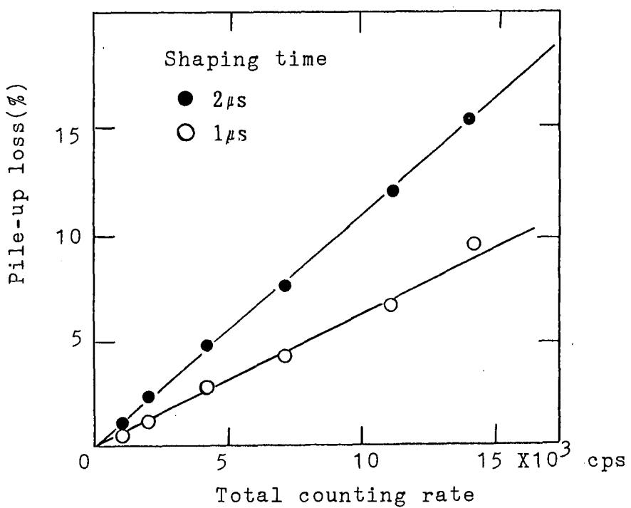
Fig. 12 Relation between pile-up loss and counting rate
