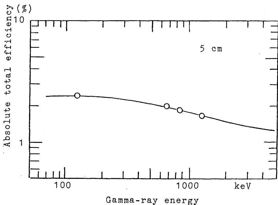
Fig. 11 Total detection efficiency of vertical HpGe detector
