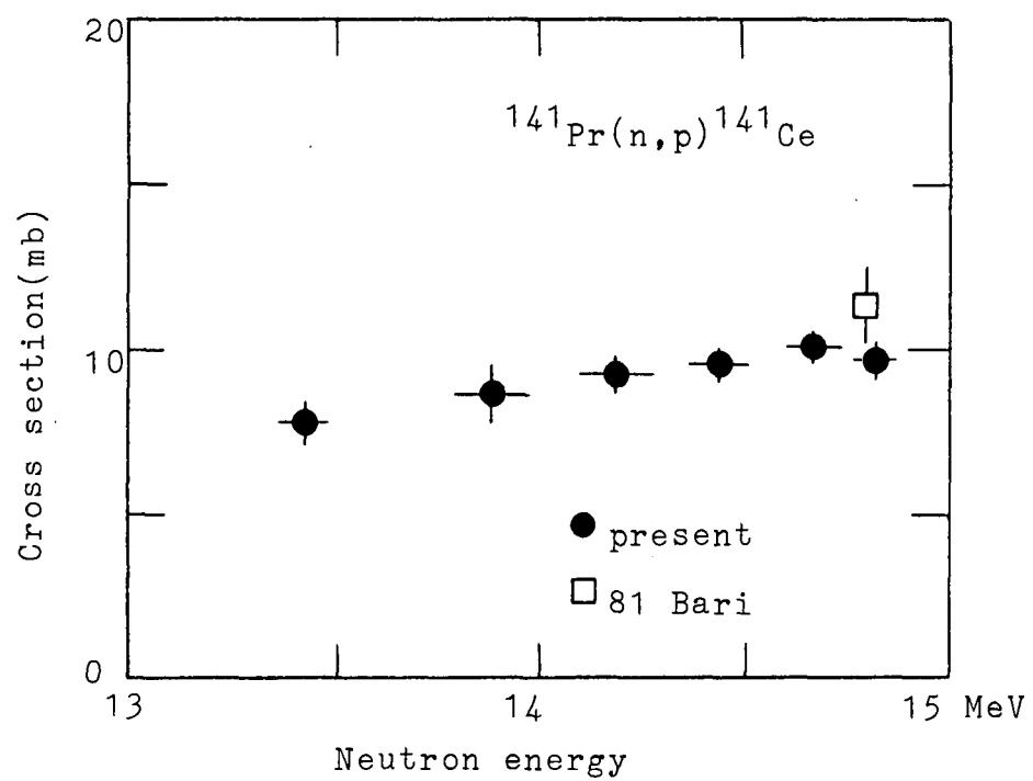
Fig. 15(b) Formation cross section of long-lived nuclei by 14 MeV neutron
