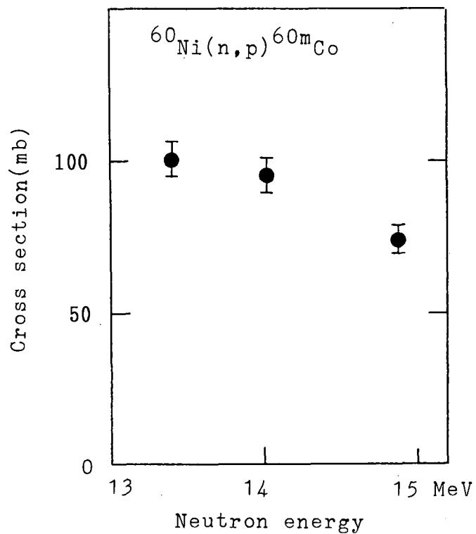
Fig. 14(c) Formation cross section of short-lived nuclei by 14 MeV neutron
