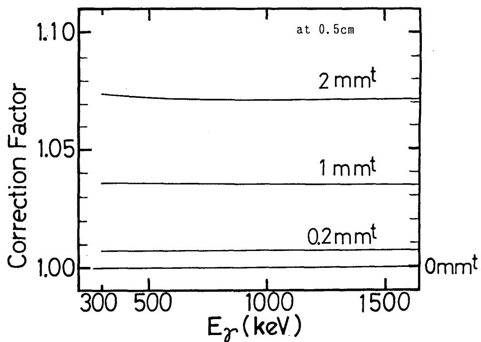
Fig. 13 Correction for the source thickness
