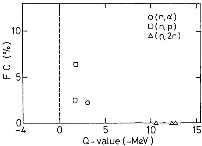
Fig. 9 Contribution of scattered neutron with energy less than 10 MeV
