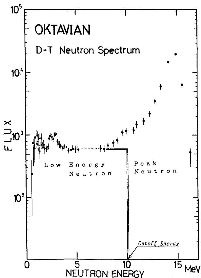
Fig. 8 Neutron spectrum at OKTAVIAN measured at the direction of  $70^\circ$  for the deuteron beam
