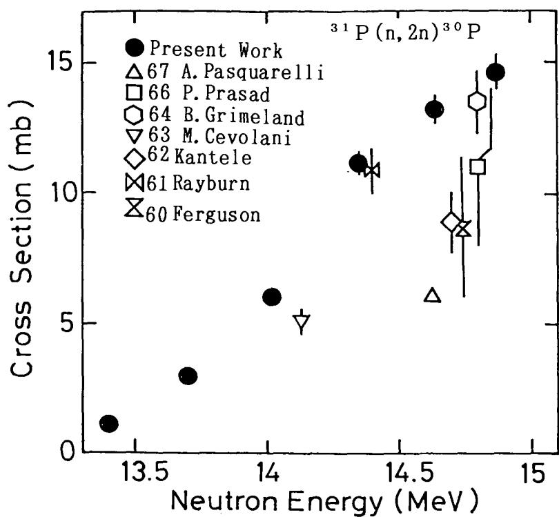
Fig. 14(a) Formation cross section of short-lived nuclei by 14 MeV neutron
