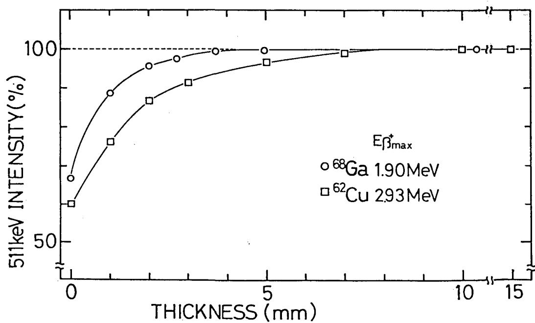
Fig. 5 Detection efficiency of the annihilation gamma-ray as functions of absorber thickness
