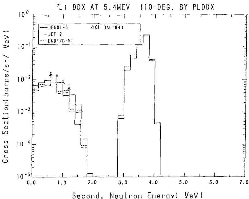
Fig. 4-4 The  ${}^7\text{Li}$  Double Differential Cross Section at 5.4 MeV,
