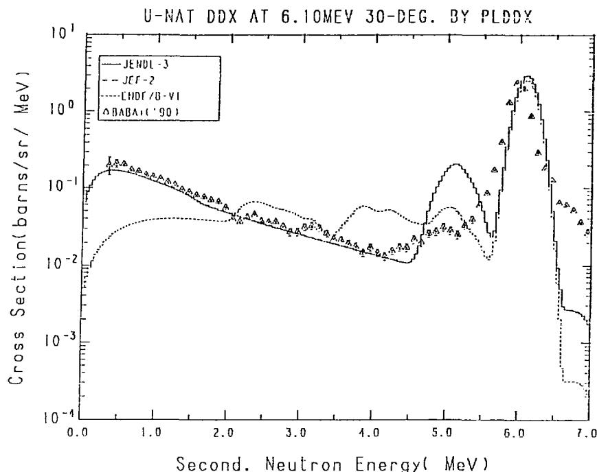
Fig. 54-1 The  $^{nat}\text{U}$  Double Differential Cross Section at 6.10 MeV,
