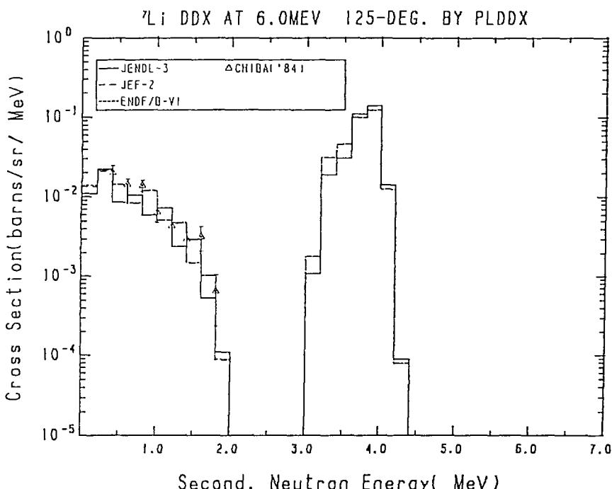
Fig. 5-4 The  $^7\text{Li}$  Double Differential Cross Section at 6.0 MeV,
