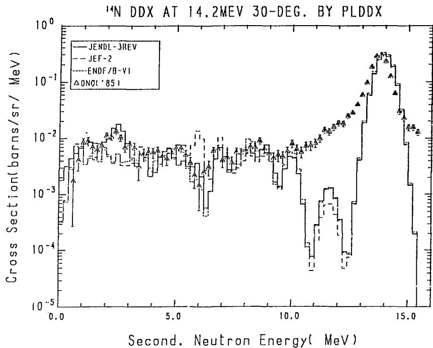
Fig. 13-1 The  $^{14}\text{N}$  Double Differential Cross Section at 14.2 MeV,
