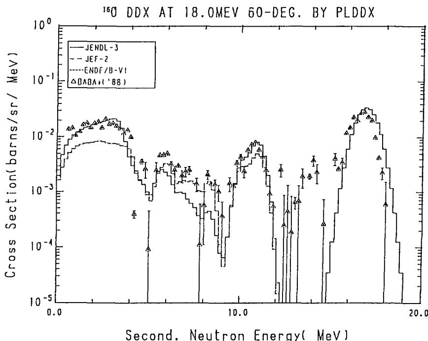
Fig. 16-2 The  $^{160}\text{O}$  Double Differential Cross Section at 18.0 MeV,
