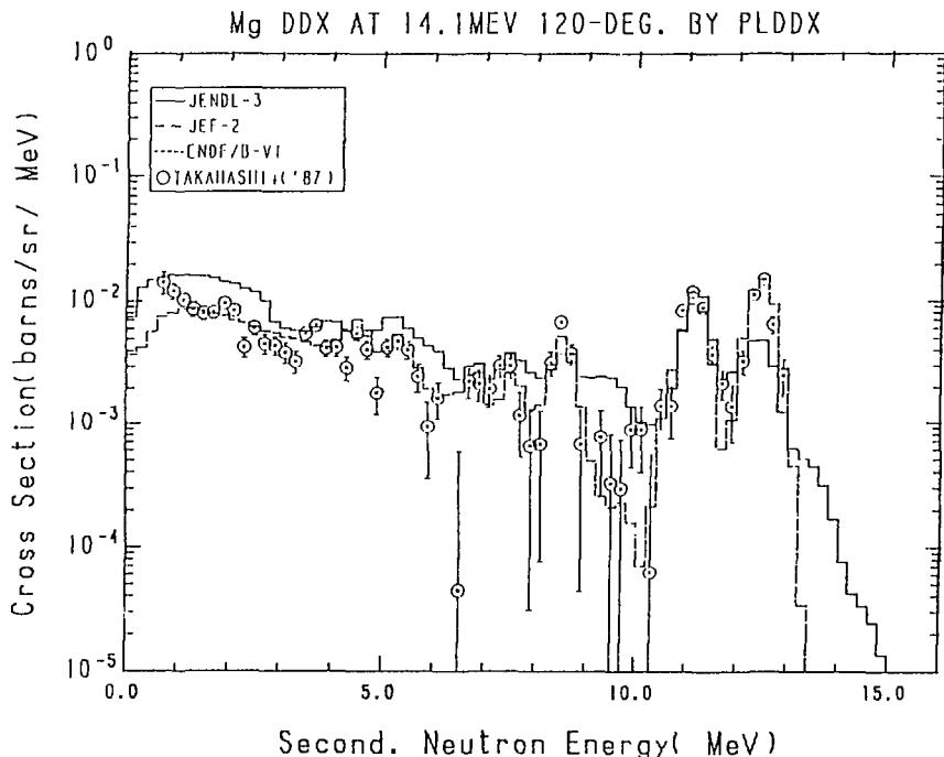
Fig. 19-4 The Magnesium Double Differential Cross Section at 14.1 MeV,
