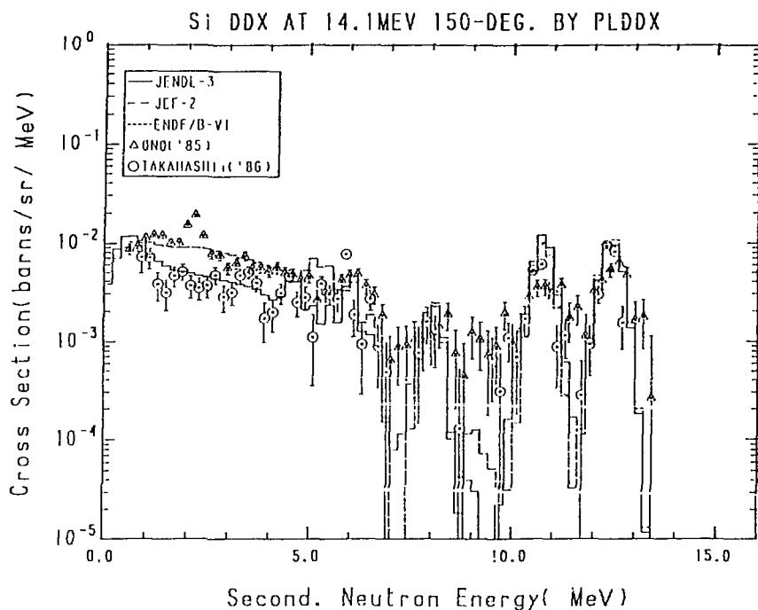
Fig. 22-5 The Silicon Double Differential Cross Section at 14.1 MeV,
