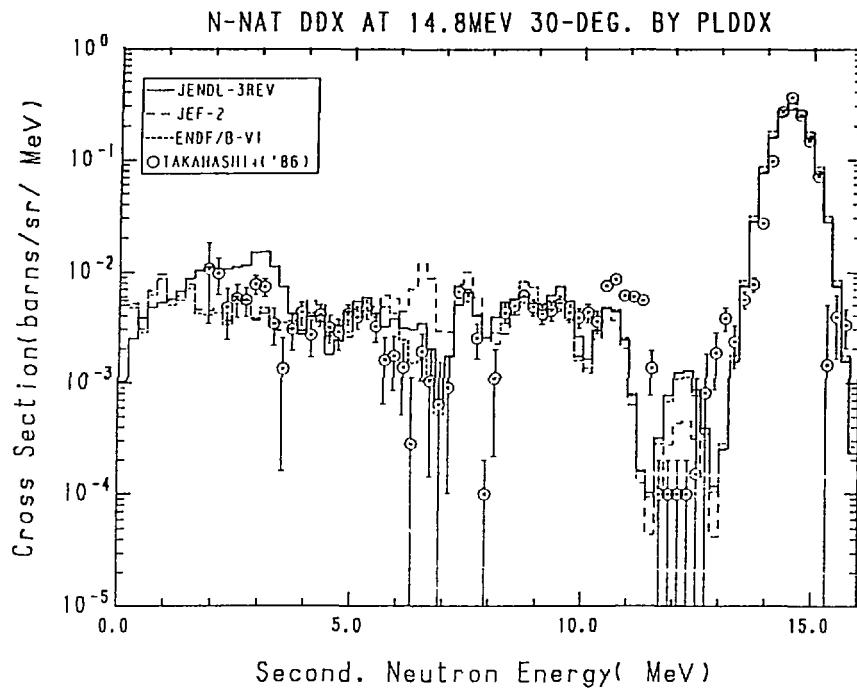
Fig. 14-1 The  $^{nat}N$  Double Differential Cross Section,
