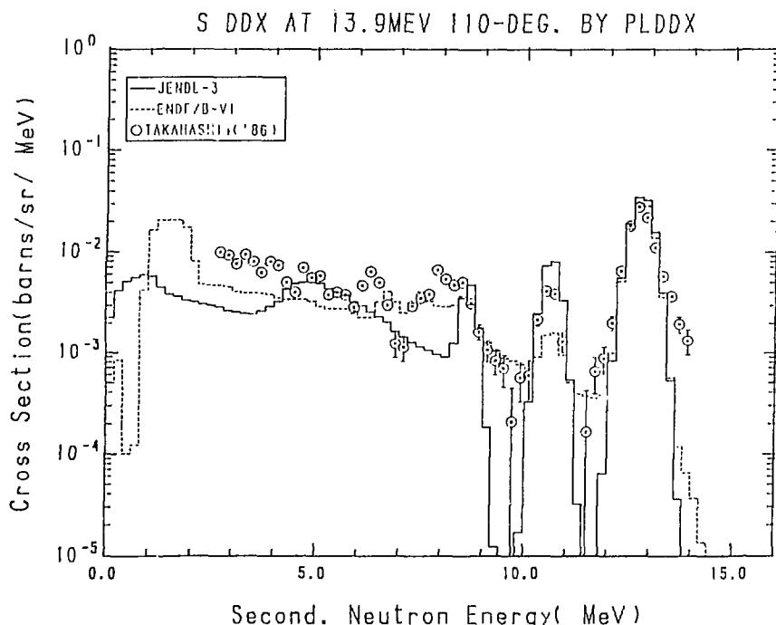
Fig. 23-4 The Sulphur Double Differential Cross Section,
