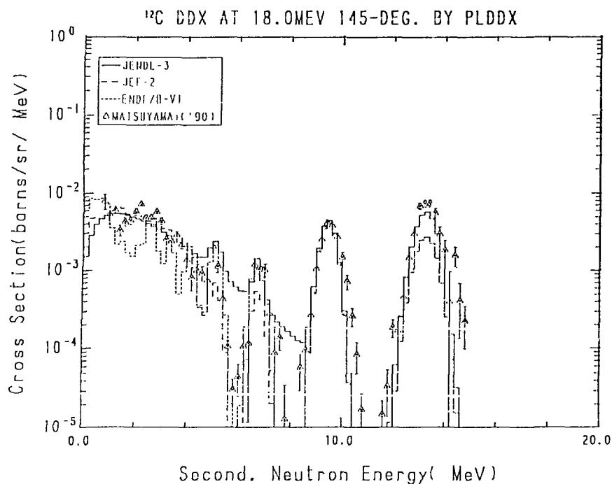
Fig. 12-5 The <sup>12</sup>C Double Differential Cross Section at 18.0 MeV,
