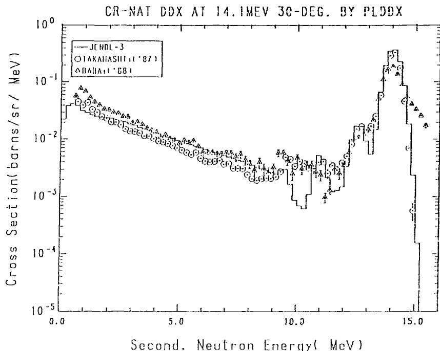
Fig. 27-1 The  $^{nat}\text{Cr}$  Double Differential Cross Section at 14.1 MeV,
