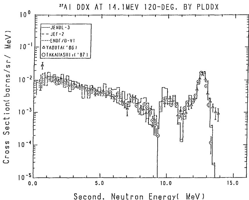
Fig. 20-4 The  $^{27}\text{Al}$  Double Differential Cross Section at 14.1 MeV,
