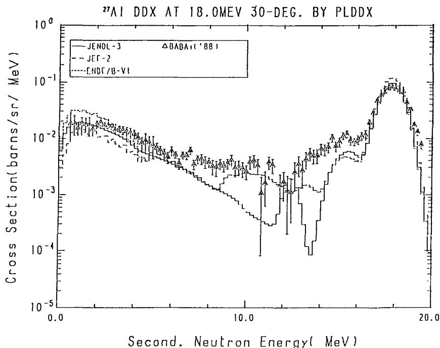
Fig. 21-1 The  $^{27}\text{Al}$  Double Differential Cross Section at 18.0 MeV,
