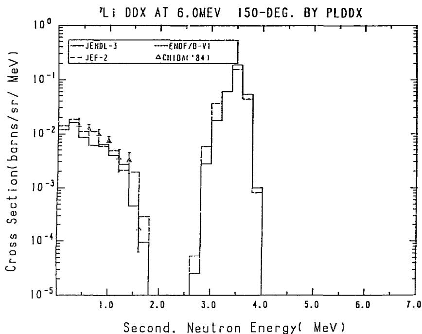
Fig. 5-5 The  $^{7\text{Li}}$  Double Differential Cross Section at 6.0 MeV,
