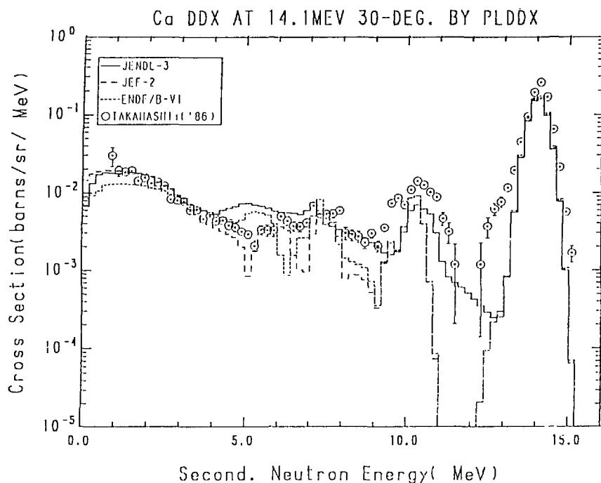
Fig. 24-1 The Calcium Double Differential Cross Section at 14.1 MeV,
