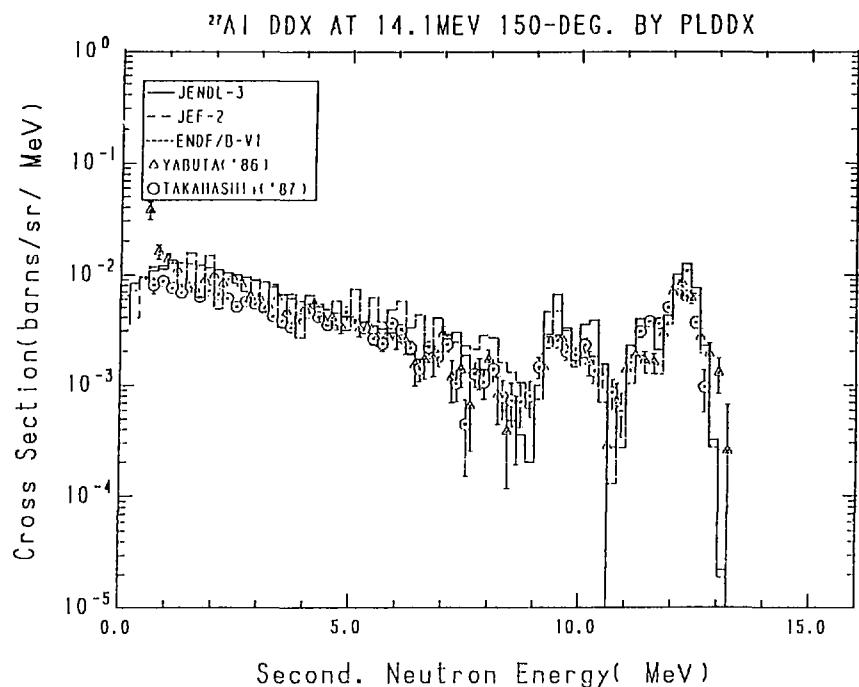
Fig. 20-5 The  $^{27}\text{Al}$  Double Differential Cross Section at 14.1 Mev,
