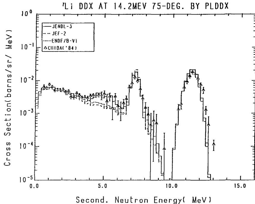
Fig. 6-3 The  $^7\text{Li}$  Double Differential Cross Section at 14.2 MeV,
