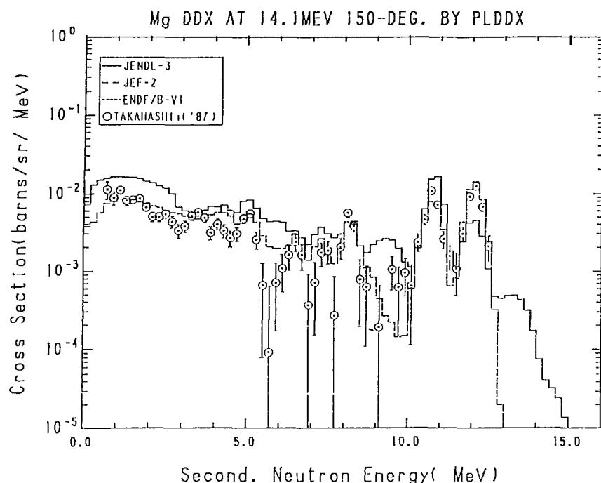
Fig. 19-5 The Magnesium Double Differential Cross Section at 14.1 MeV,
