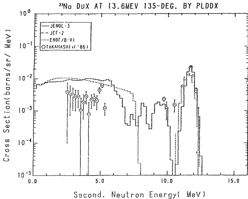
Fig. 18-5 The  $^{23}\text{Na}$  Double Differential Cross Section,
