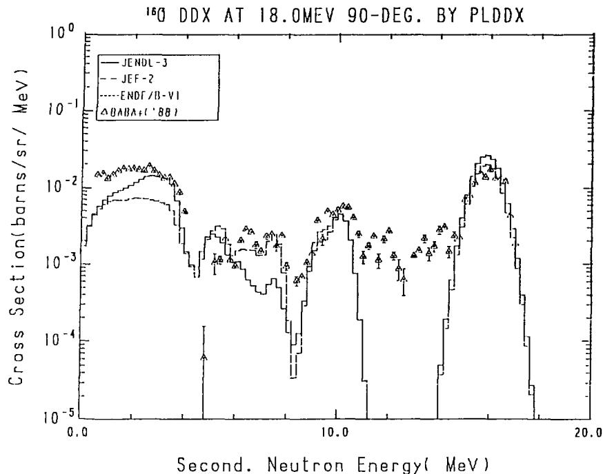
Fig. 16-3 The  $^{160}$  Double Differential Cross Section at 18.0 MeV,
