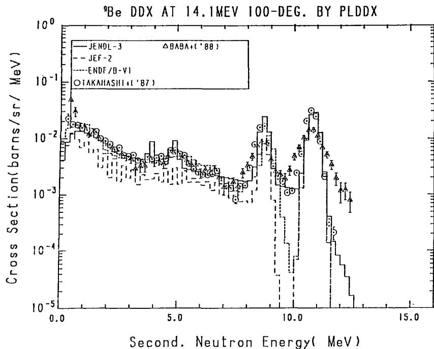
Fig. 8-3 The <sup>9</sup>Be Double Differential Cross Section at 14.1 MeV,
