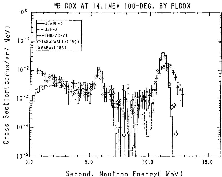
Fig. 9-3 The  $^{10}\text{B}$  Double Differential Cross Section at 14.1 MeV,
