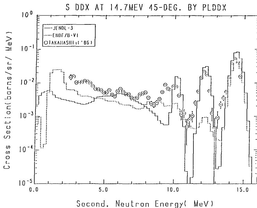
Fig. 23-1 The Sulphur Double Differential Cross Section,
