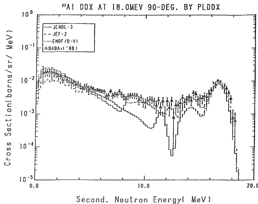
Fig. 21-3 The  $^{27}\text{Al}$  Double Differential Cross Section at 18.0 MeV,
