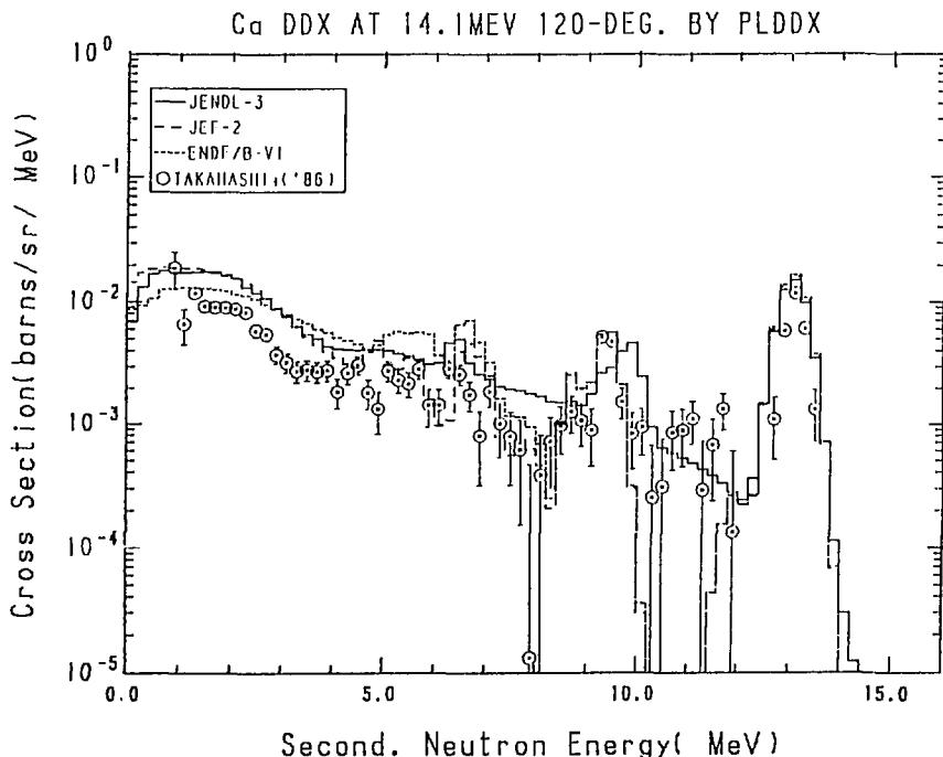
Fig. 24-4 The Calcium Double Differential Cross Section at 14.1 MeV,
