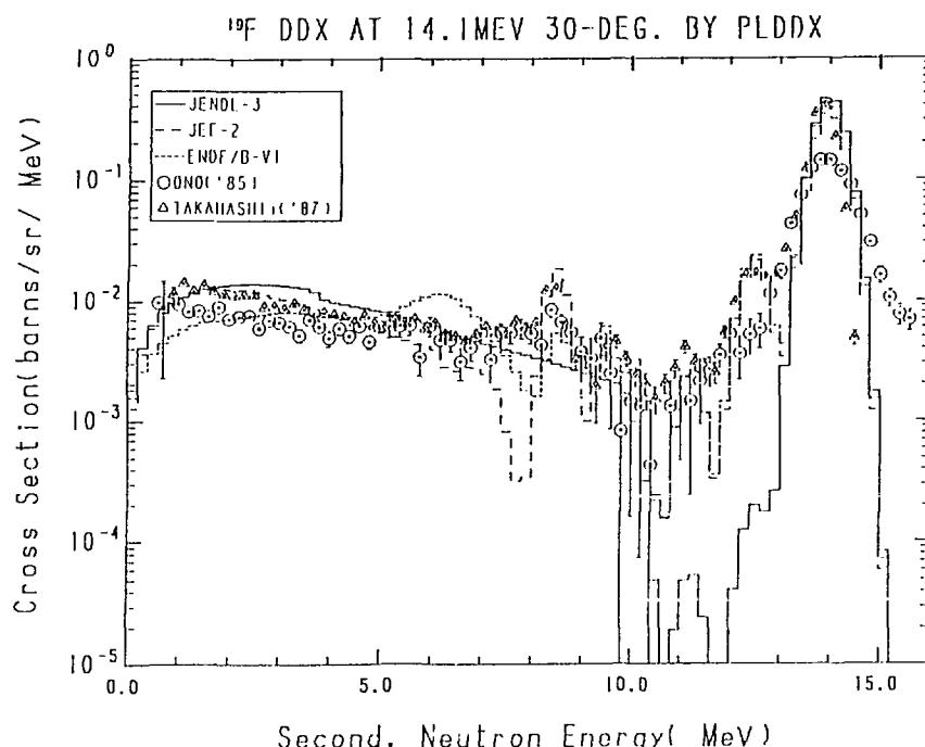
Fig. 17-1 The  $^{19}\text{F}$  Double Differential Cross Section at 14.1 MeV,
