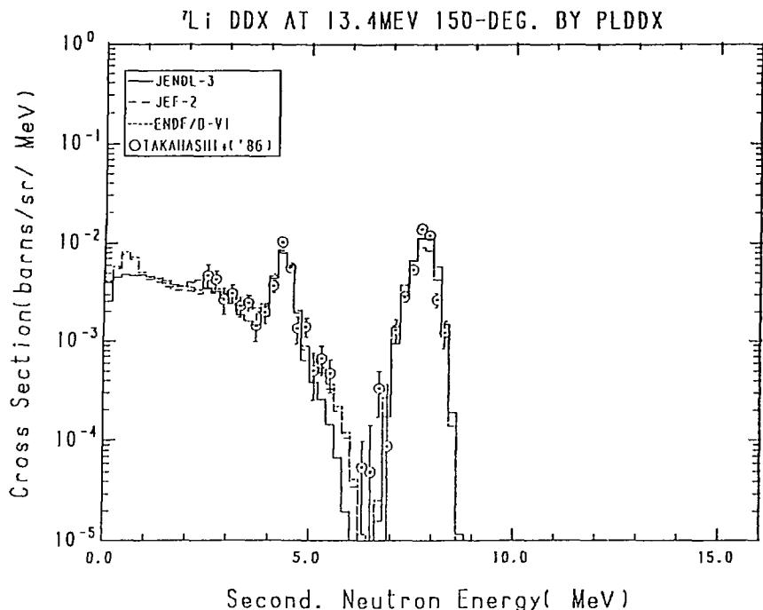
Fig. 7-5 The  ${}^7\text{Li}$  Double Differential Cross Section,
