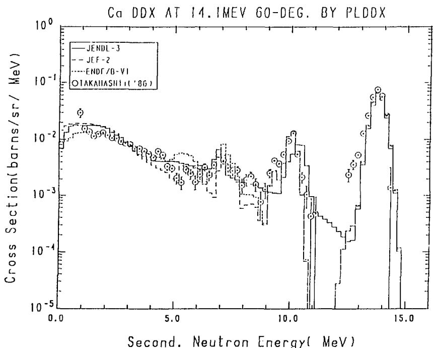
Fig. 24-2 The Calcium Double Differential Cross Section at 14.1 MeV,
