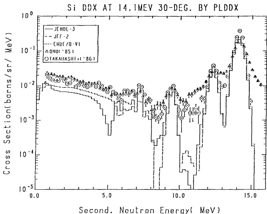
Fig. 22-1 The Silicon Double Differential Cross Section at 14.1 MeV,
