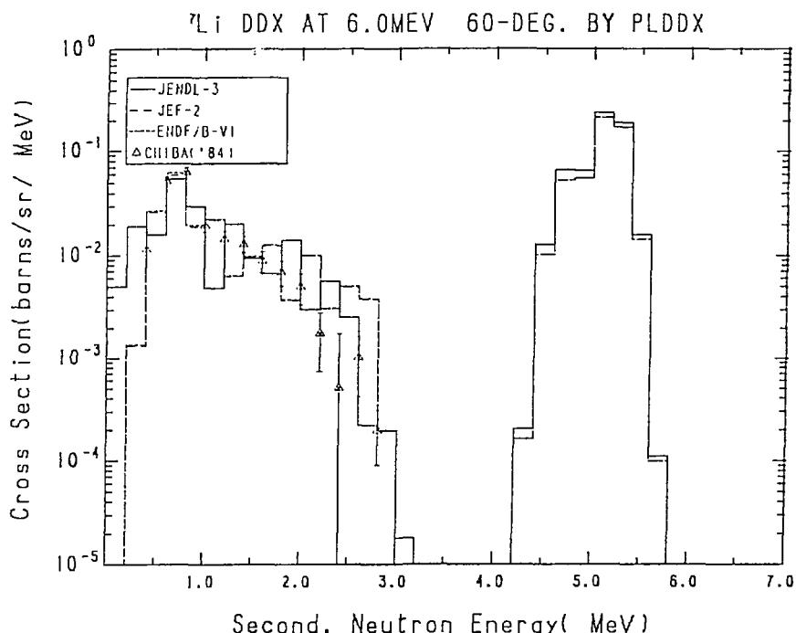
Fig. 5-2 The  ${}^7\text{Li}$  Double Differential Cross Section at 6.0 MeV,
