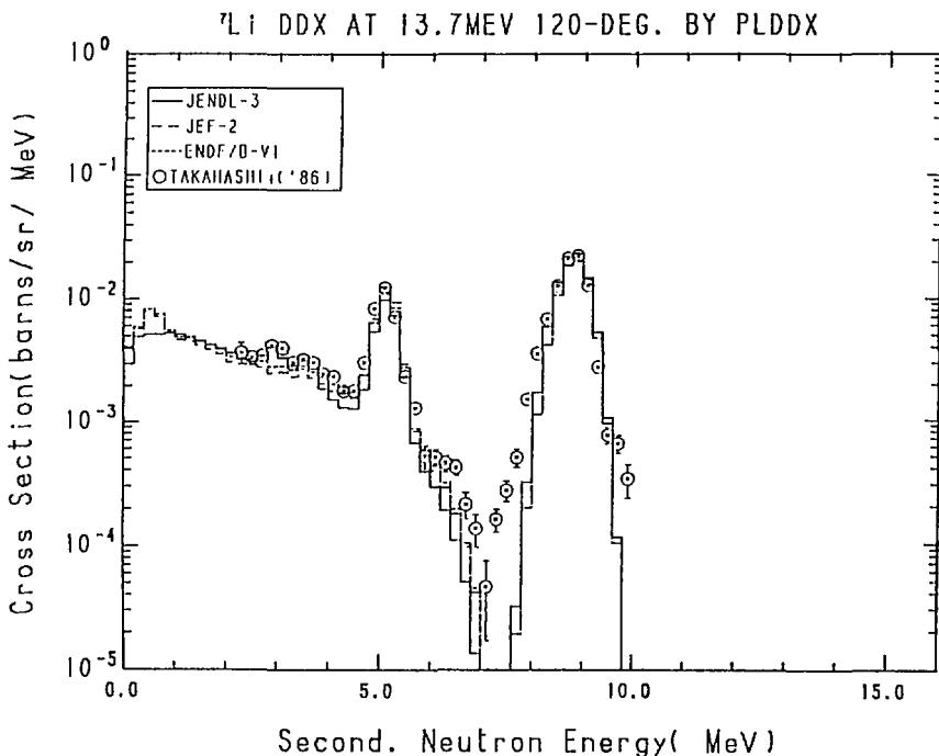
Fig. 7-4 The  $^7\text{Li}$  Double Differential Cross Section,
