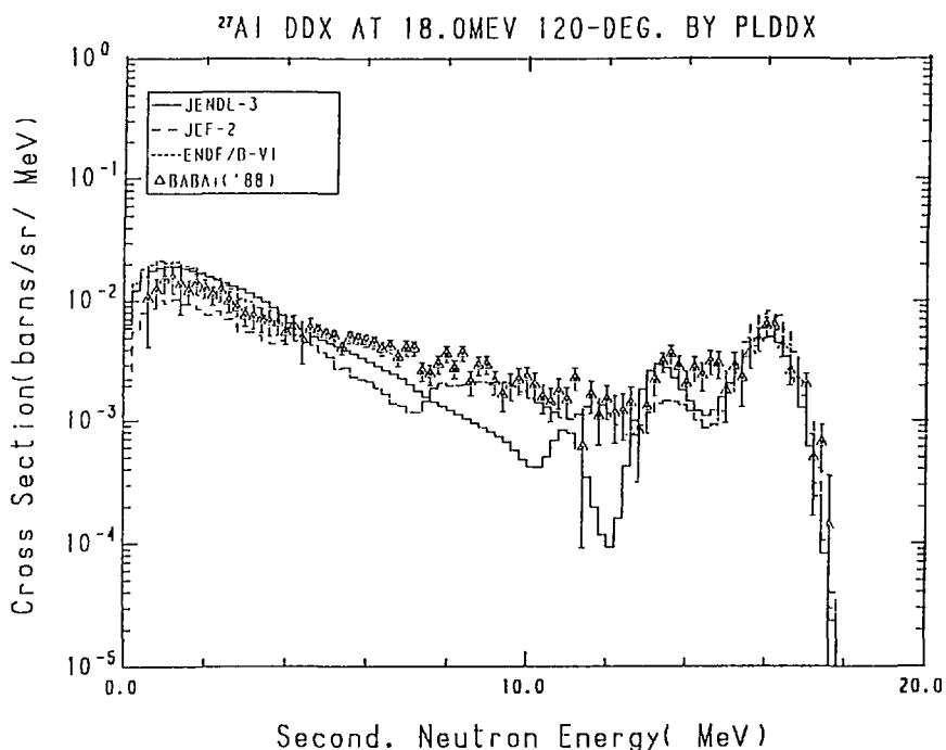
Fig. 21-4 The  $^{27}\text{Al}$  Double Differential Cross Section at 18.0 MeV,
