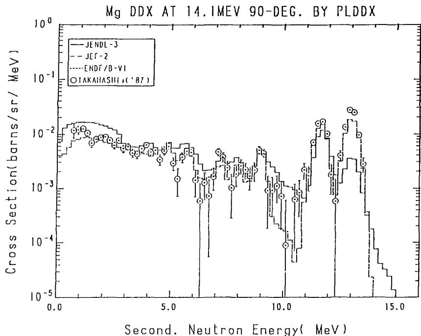
Fig. 19-3 The Magnesium Double Differential Cross Section at 14.1 MeV,
