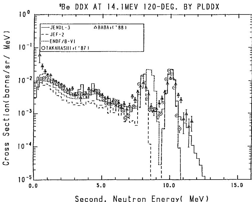
Fig. 8-4 The <sup>9</sup>Be Double Differential Cross Section at 14.1 MeV,
