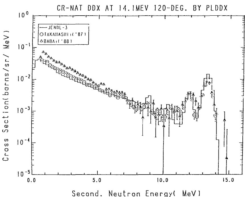
Fig. 27-4 The  $^{nat}\text{Cr}$  Double Differential Cross Section at 14.1 MeV,
