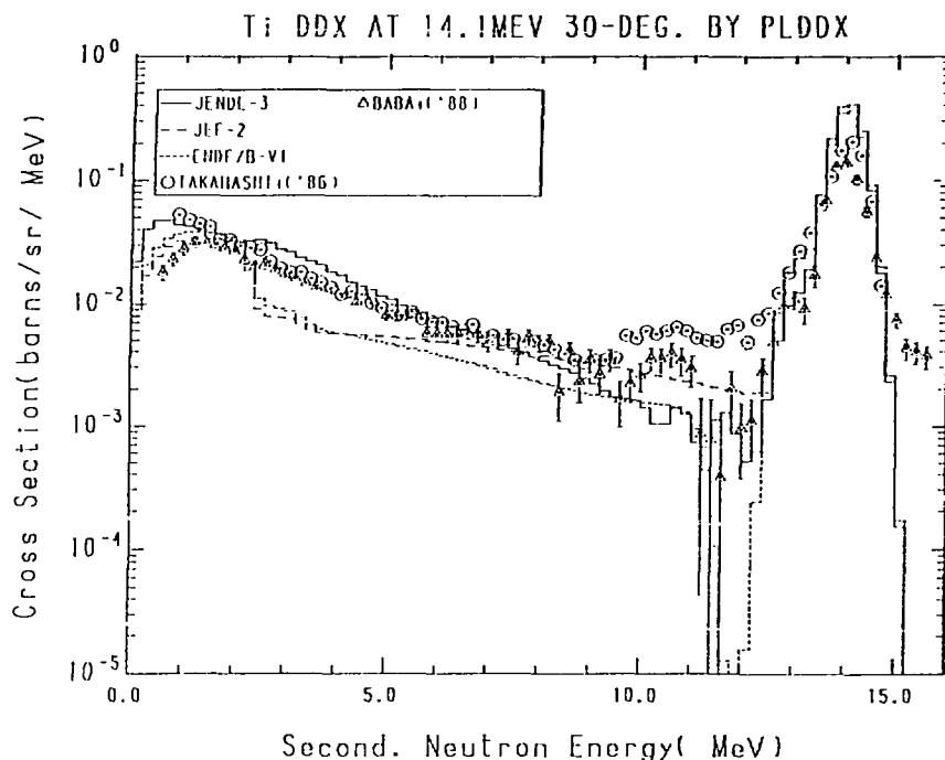
Fig. 25-1 The Titanium Double Differential Cross Section at 14.1 MeV,
