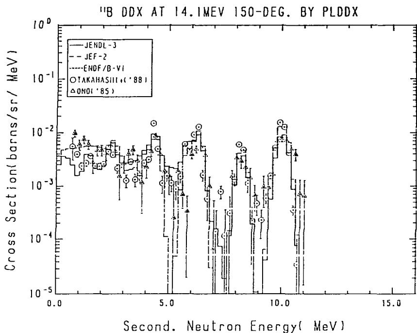
Fig. 10-5 The <sup>11</sup>B Double Differential Cross Section at 14.1 MeV,
