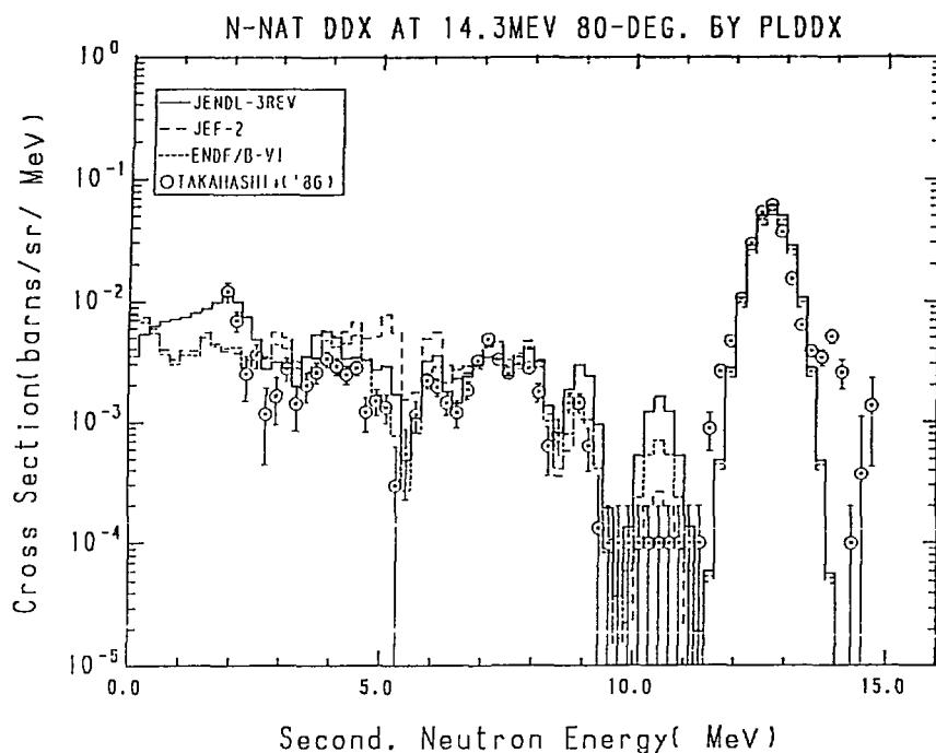
Fig. 14-3 The  $^{nat}N$  Double Differential Cross Section,
