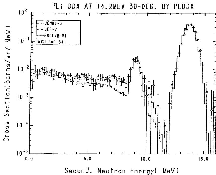
Fig. 6-1 The  $^7\text{Li}$  Double Differential Cross Section at 14.2 MeV,
