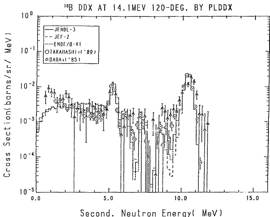
Fig. 9-4 The  $^{10}\text{B}$  Double Differential Cross Section at 14.1 MeV,
