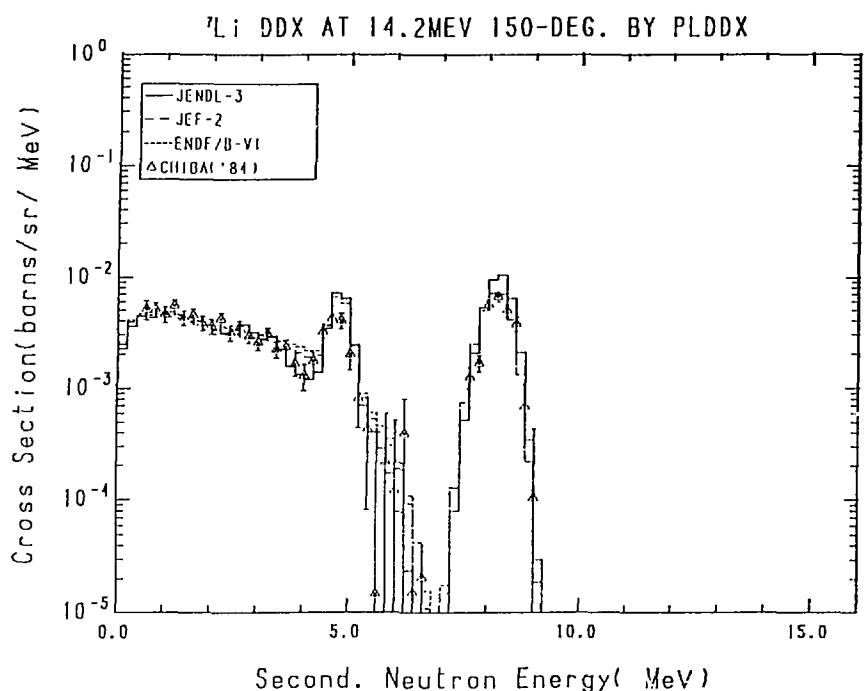
Fig. 6-5 The  $^{7}\text{Li}$  Double Differential Cross Section at 14.2 MeV,
