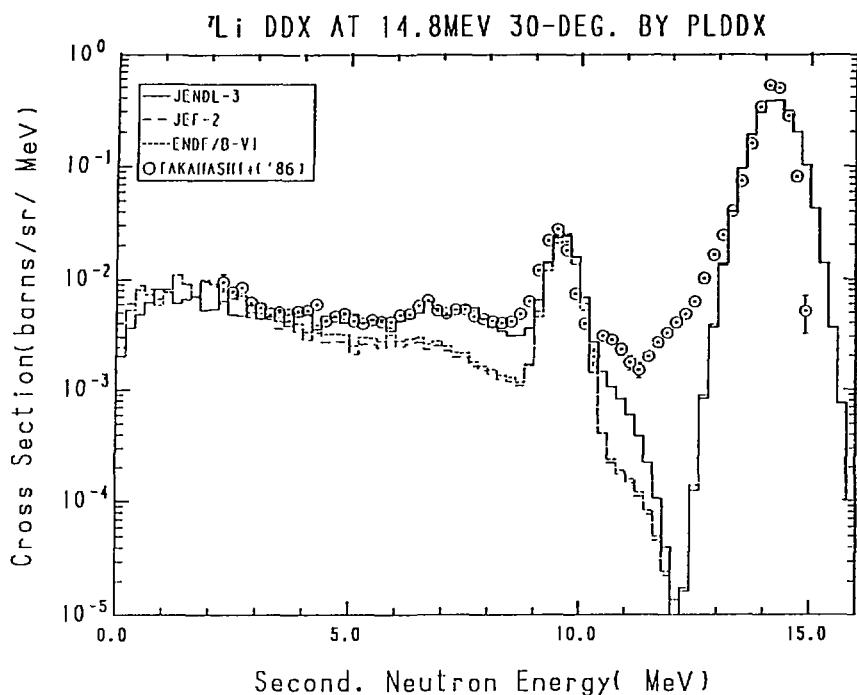
Fig. 7-1 The  ${}^7\text{Li}$  Double Differential Cross Section,
