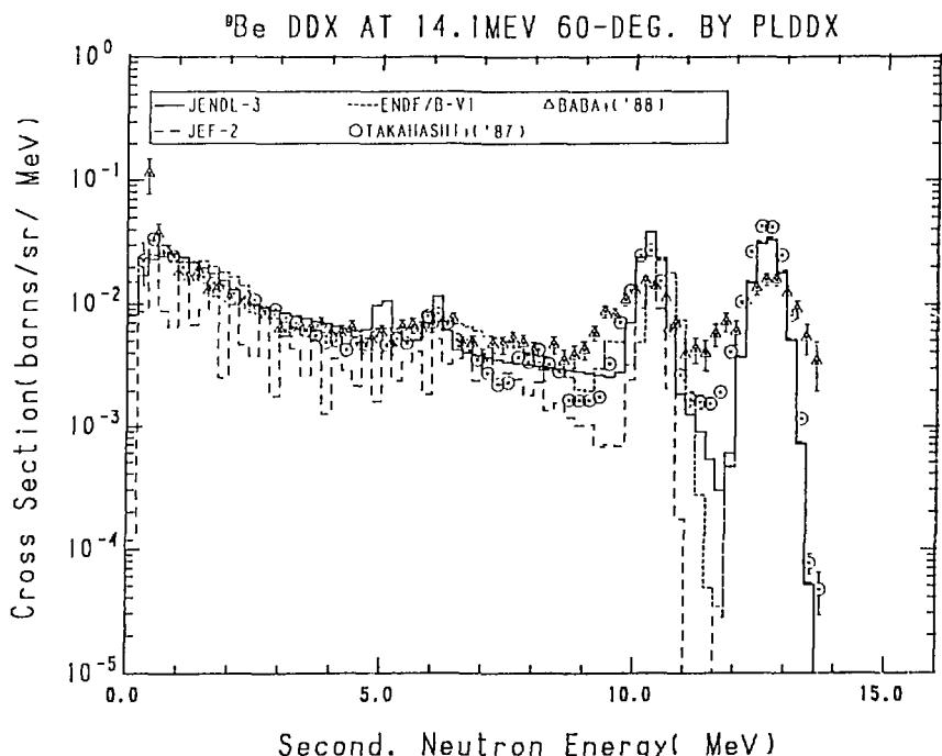
Fig. 8-2 The  ${}^9\text{Be}$  Double Differential Cross Section at 14.1 MeV,
