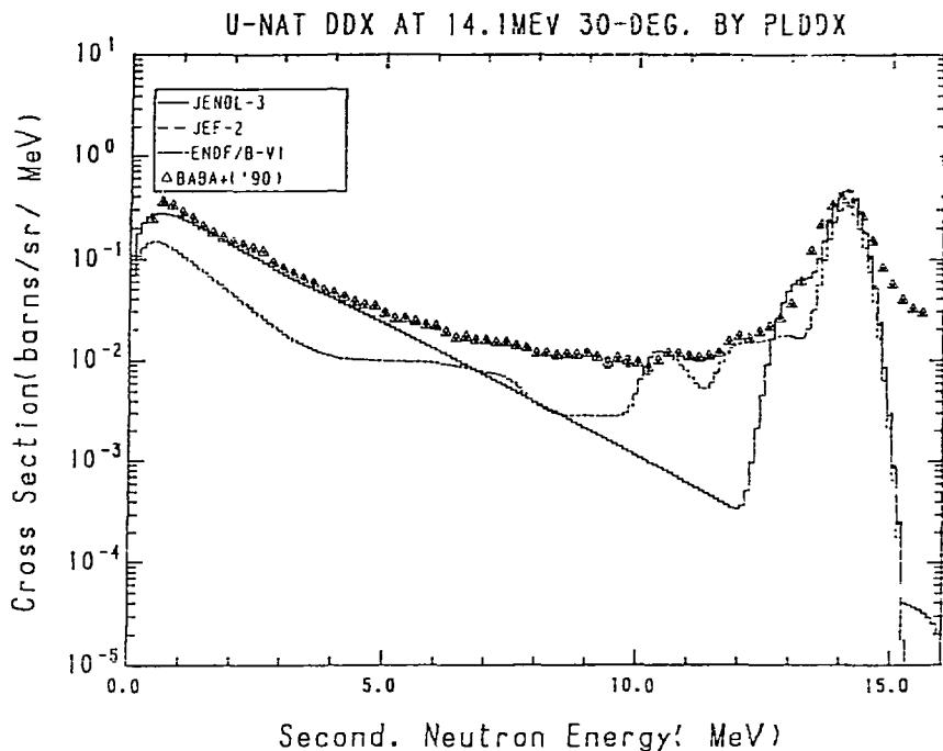
Fig. 55-1 The  $^{nat}U$  Double Differential Cross Section at 14.1 MeV,
