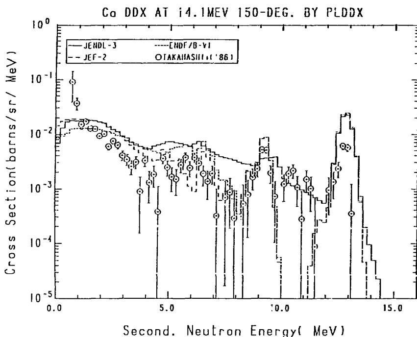
Fig. 24-5 The Calcium Double Differential Cross Section at 14.1 MeV,
