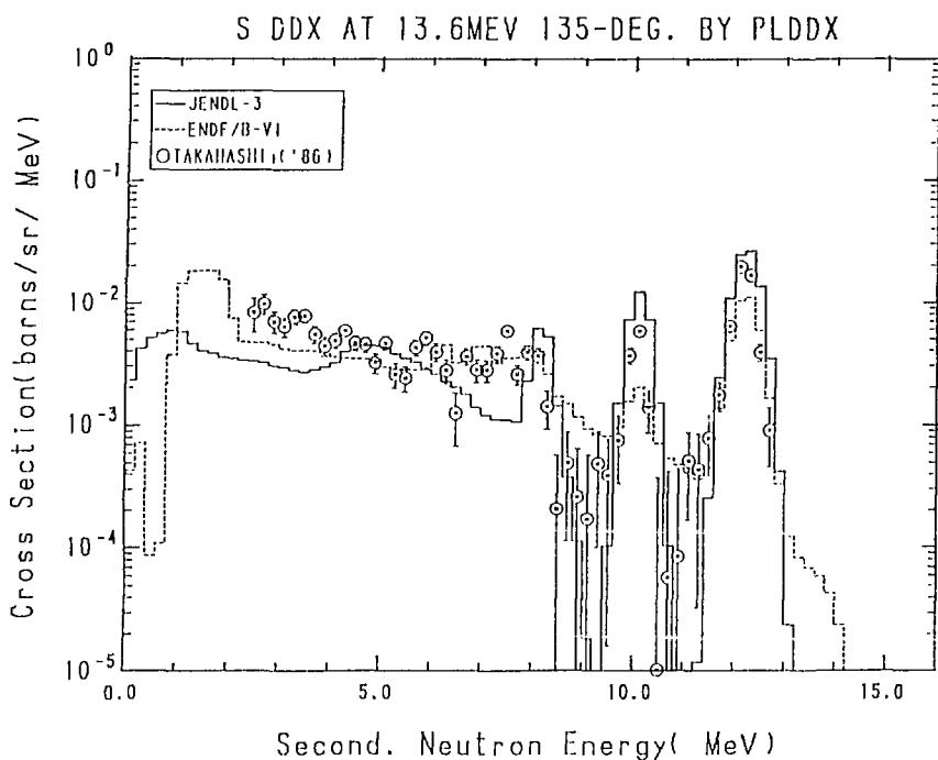
Fig. 23-5 The Sulphur Double Differential Cross Section,
