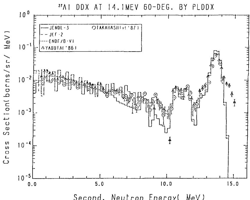
Fig. 20-2 The  $^{27}\text{Al}$  Double Differential Cross Section at 14.1 MeV,
