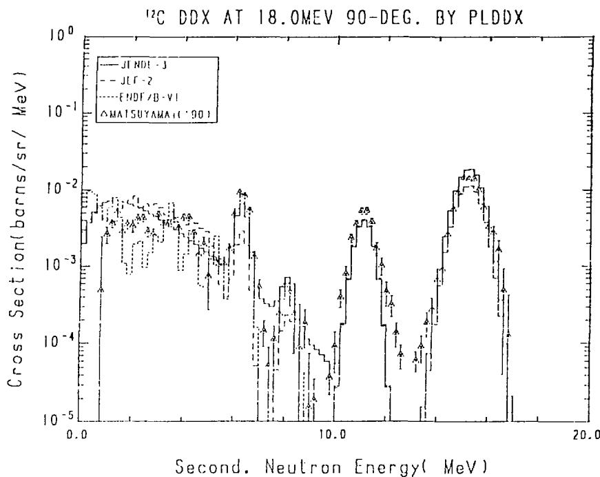
Fig. 12-3 The  $^{12}\text{C}$  Double Differential Cross Section at 18.0 MeV,
