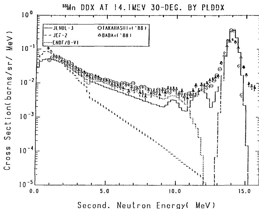
Fig. 28-1 The  $^{55}\text{Mn}$  Double Differential Cross Section at 14.1 MeV,
