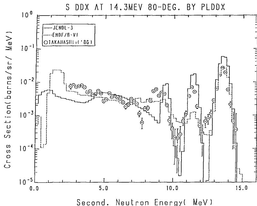
Fig. 23-3 The Sulphur Double Differential Cross Section,
