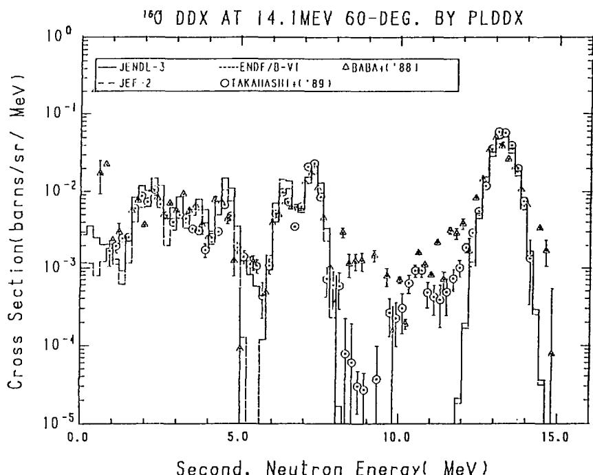
Fig. 15-2 The  $^{160}\text{O}$  Double Differential Cross Section at 14.1 MeV,
