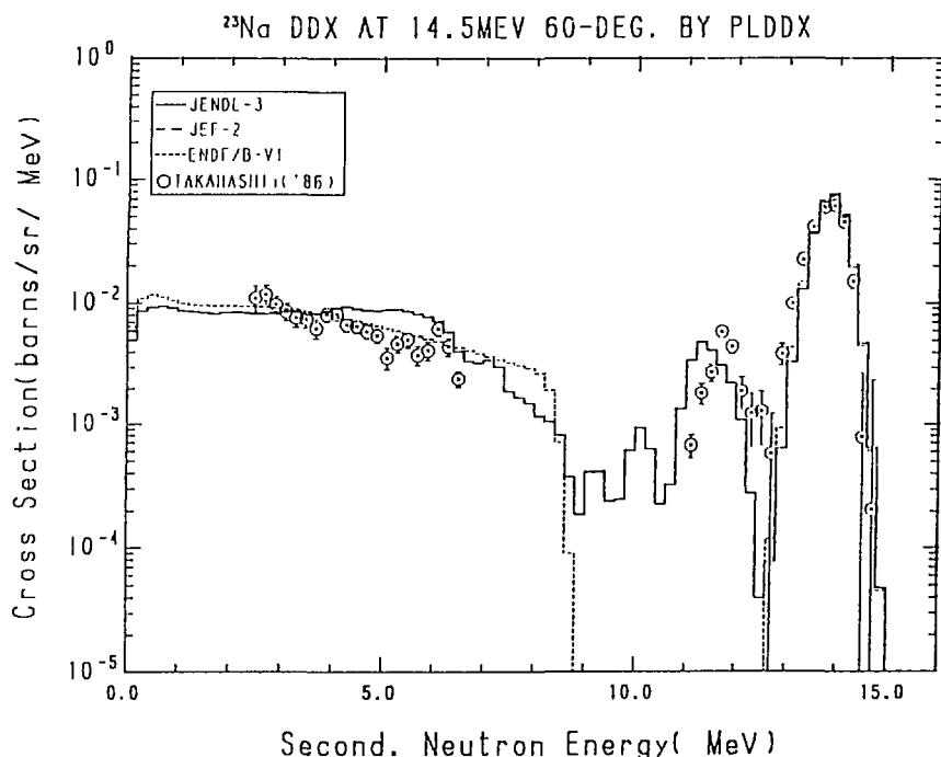
Fig. 18-2 The  $^{23}\text{Na}$  Double Differential Cross Section,
