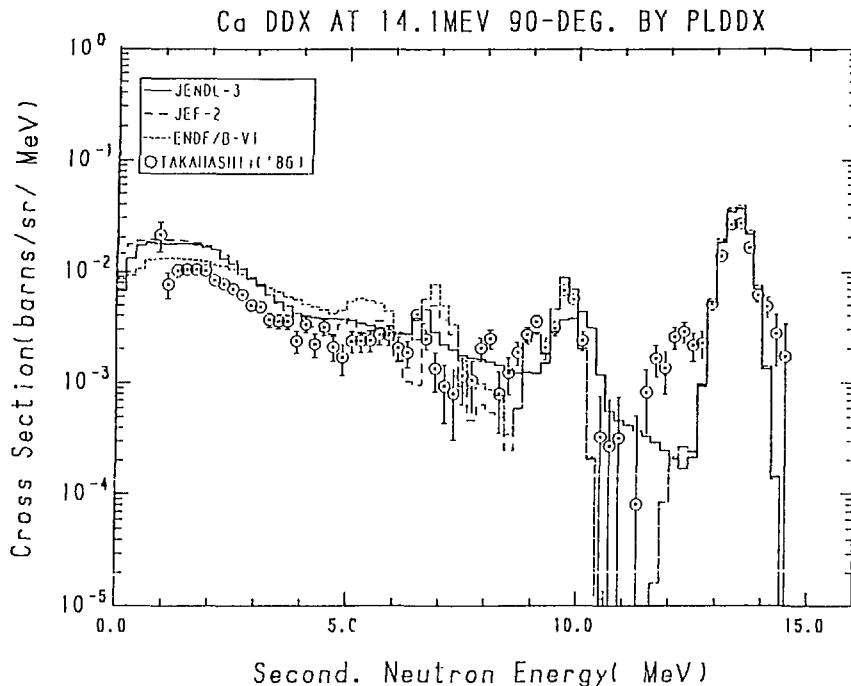
Fig. 24-3 The Calcium Double Differential Cross Section at 14.1 MeV,
