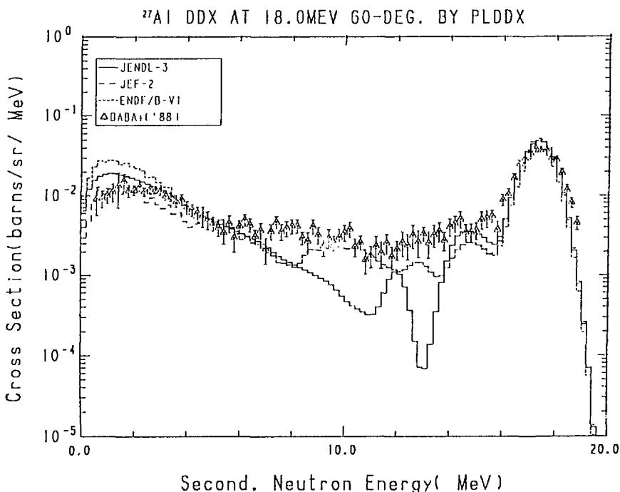
Fig. 21-2 The  $^{27}\text{Al}$  Double Differential Cross Section at 18.0 MeV,
