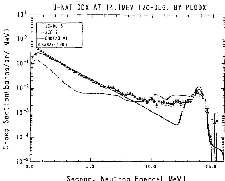
Fig. 55-4 The  $^{nat}U$  Double Differential Cross Section at 14.1 MeV,
