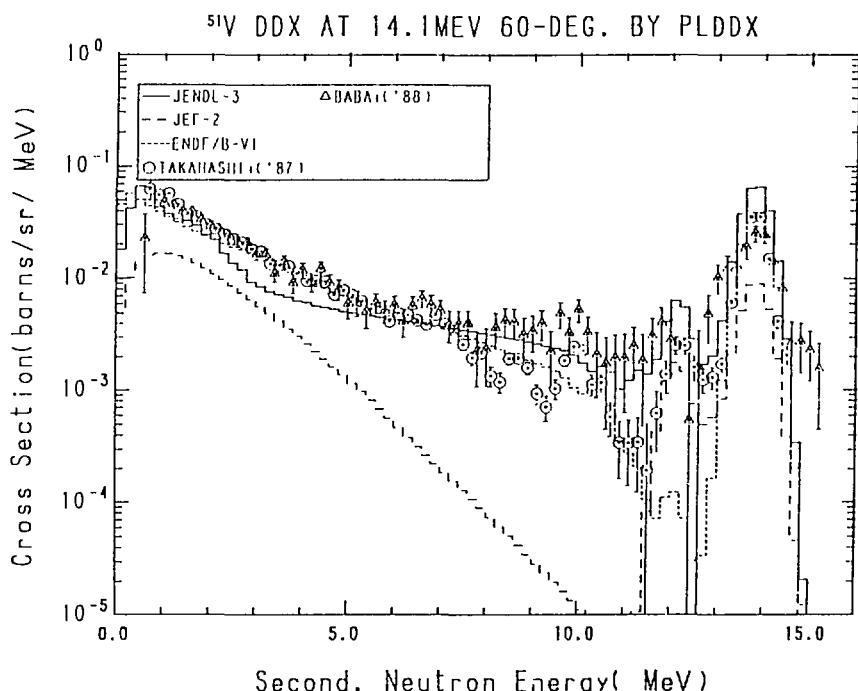
Fig. 26-2 The  $^{51}\text{V}$  Double Differential Cross Section at 14.1 MeV,
