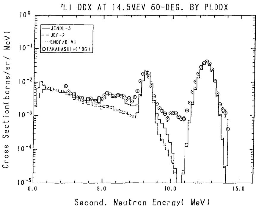
Fig. 7-2 The  ${}^7\text{Li}$  Double Differential Cross Section,
