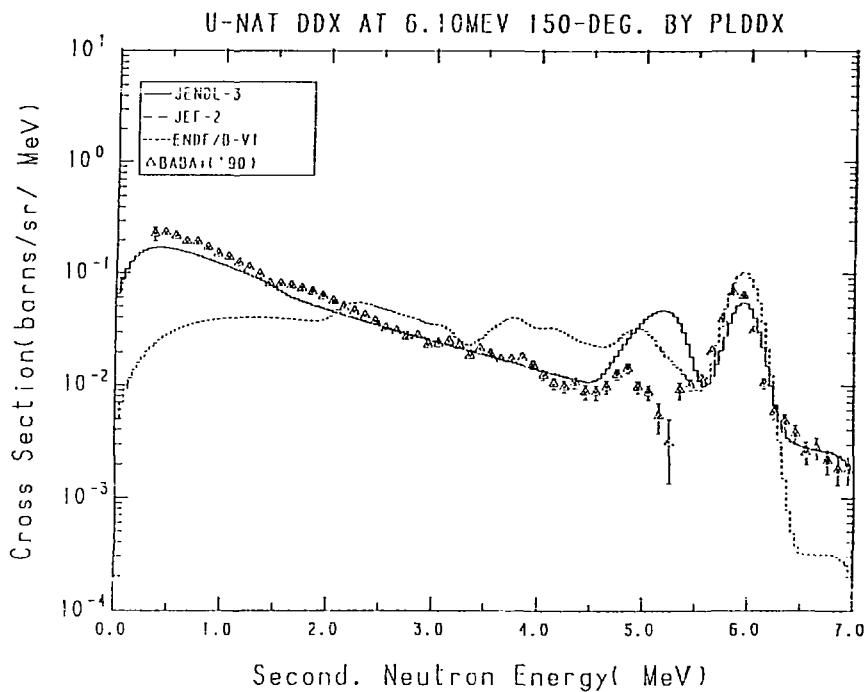
Fig. 54-5 The  $^{nat}U$  Double Differential Cross Section at 6.10 MeV,
