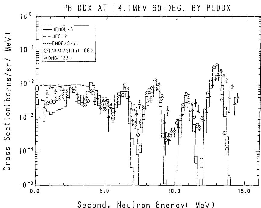
Fig. 10-2 The  $^{11}\text{B}$  Double Differential Cross Section at 14.1 MeV,
