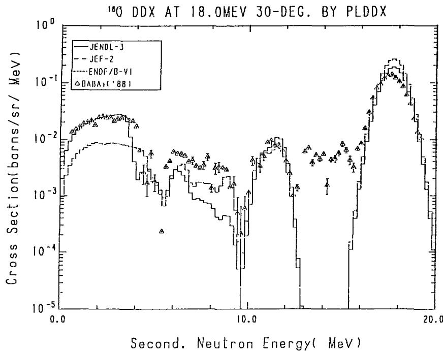
Fig. 16-1 The  $^{160}\text{O}$  Double Differential Cross Section at 18.0 MeV,
