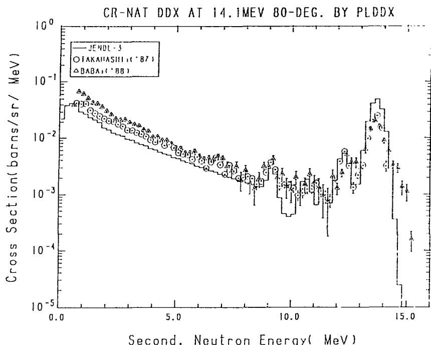
Fig. 27-3 The  $^{nat}\text{Cr}$  Double Differential Cross Section at 14.1 MeV,
