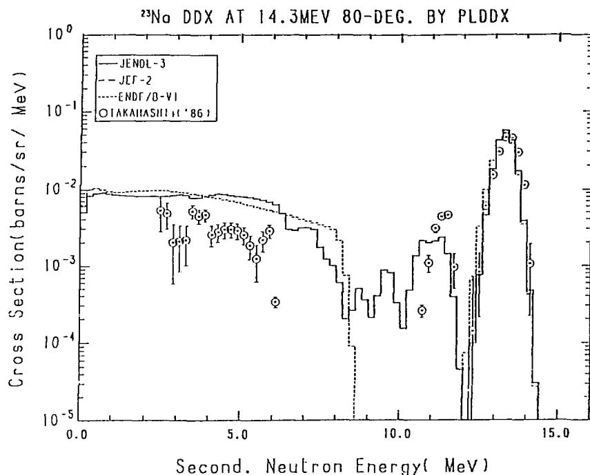
Fig. 18-3 The  $^{23}\text{Na}$  Double Differential Cross Section,
