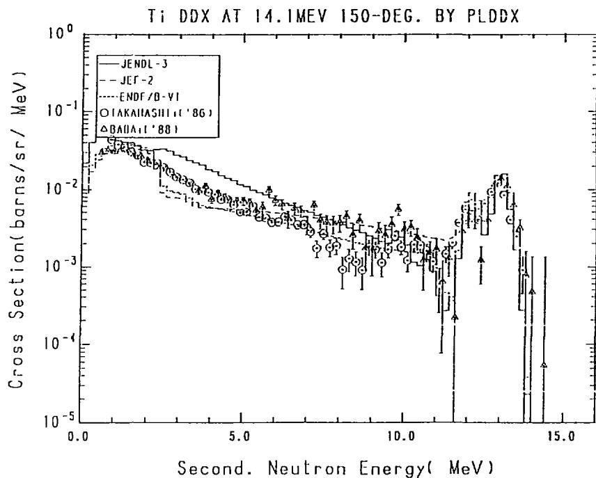
Fig. 25-5 The Titanium Double Differential Cross Section at 14.1 MeV,
