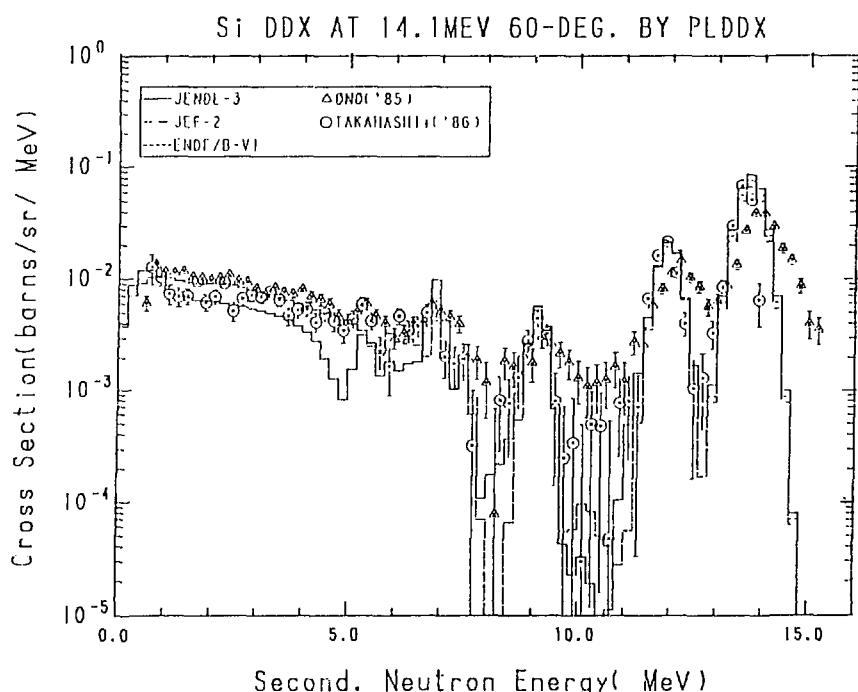
Fig. 22-2 The Silicon Double Differential Cross Section at 14.1 MeV,
