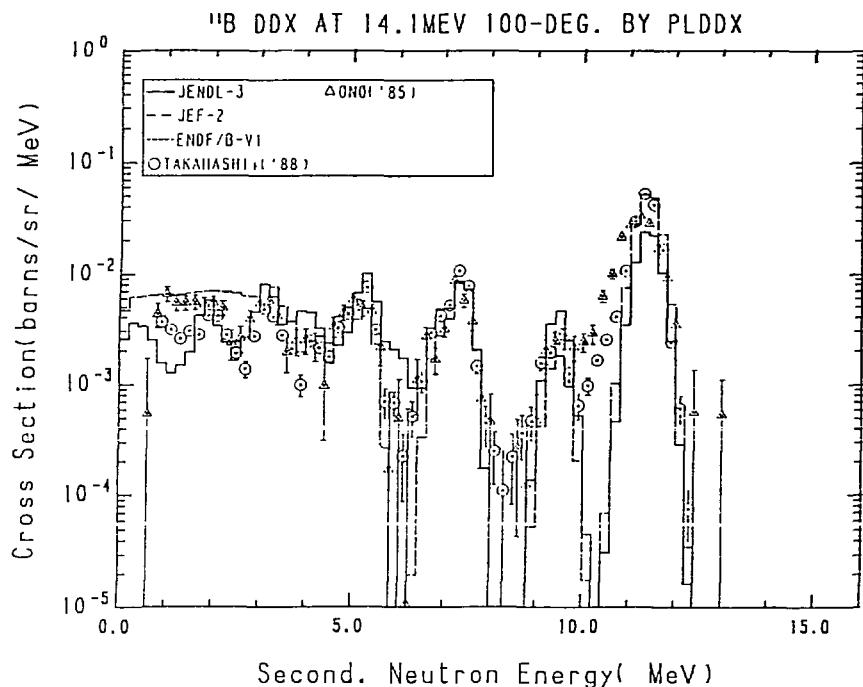
Fig. 10-3 The  $^{11}\text{B}$  Double Differential Cross Section at 14.1 MeV,
