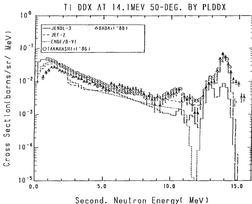
Fig. 25-2 The Titanium Double Differential Cross Section at 14.1 MeV,
