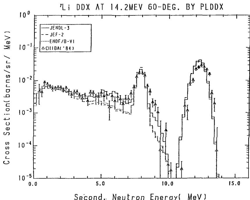
Fig. 6-2 The  $^7\text{Li}$  Double Differential Cross Section at 14.2 MeV,
