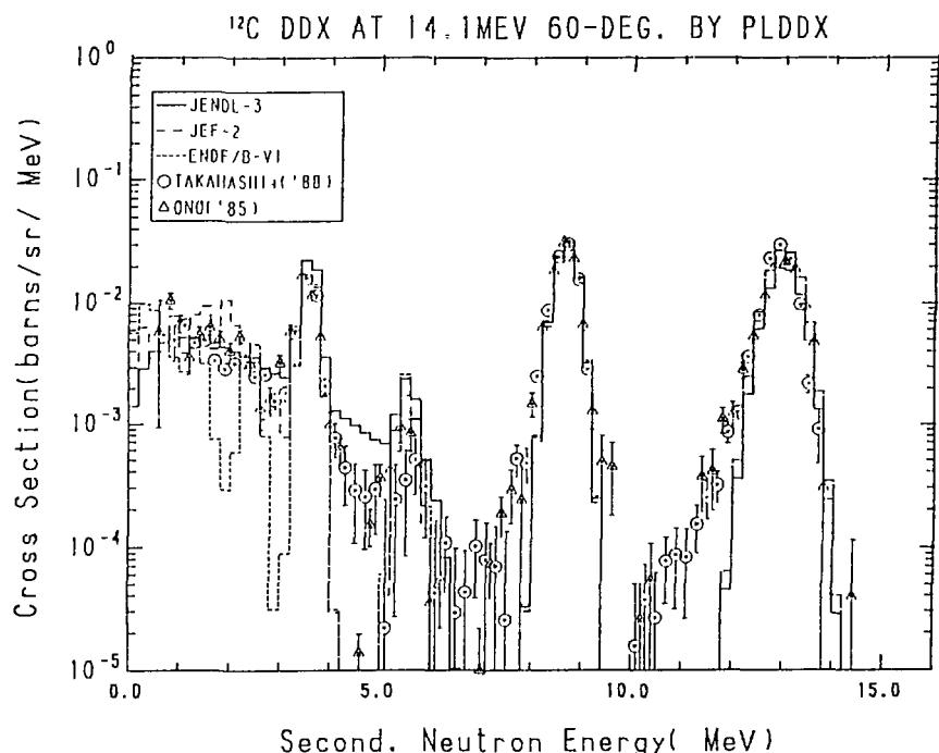
Fig. 11-2 The  $^{12}\text{C}$  Double Differential Cross Section at 14.1 MeV,
