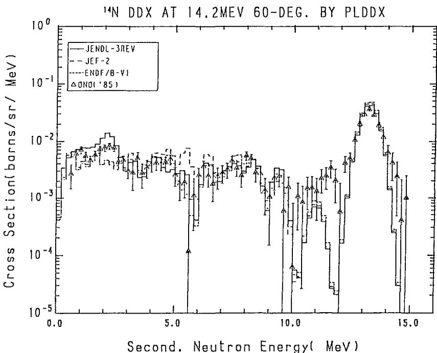
Fig. 13-2 The  $^{14}\text{N}$  Double Differential Cross Section at 14.2 MeV,
