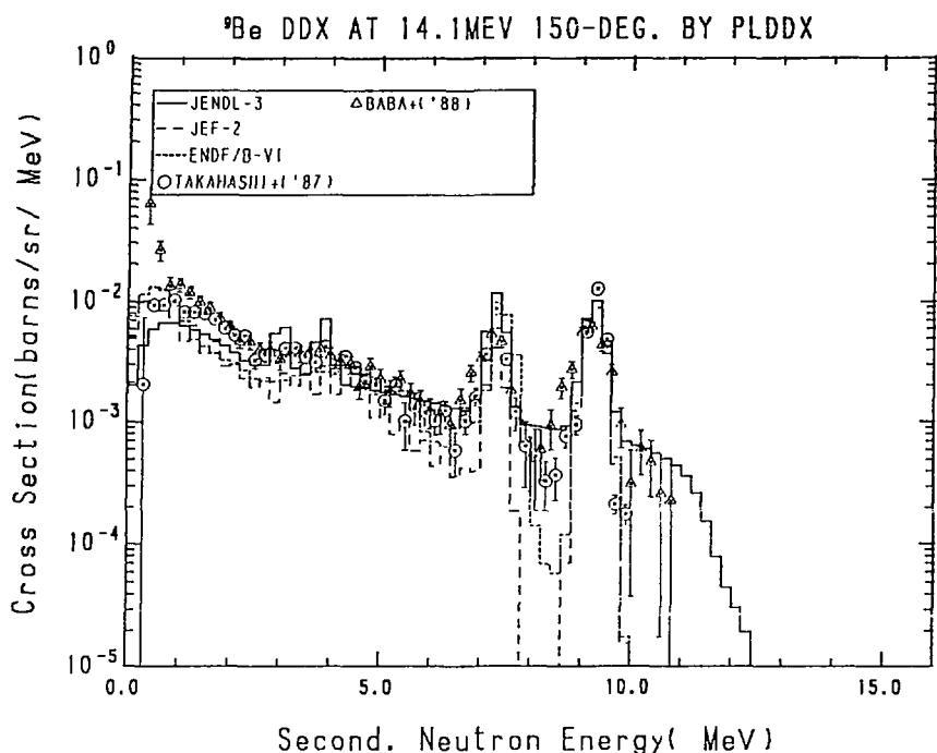
Fig. 8-5 The <sup>9</sup>Be Double Differential Cross Section at 14.1 MeV,
