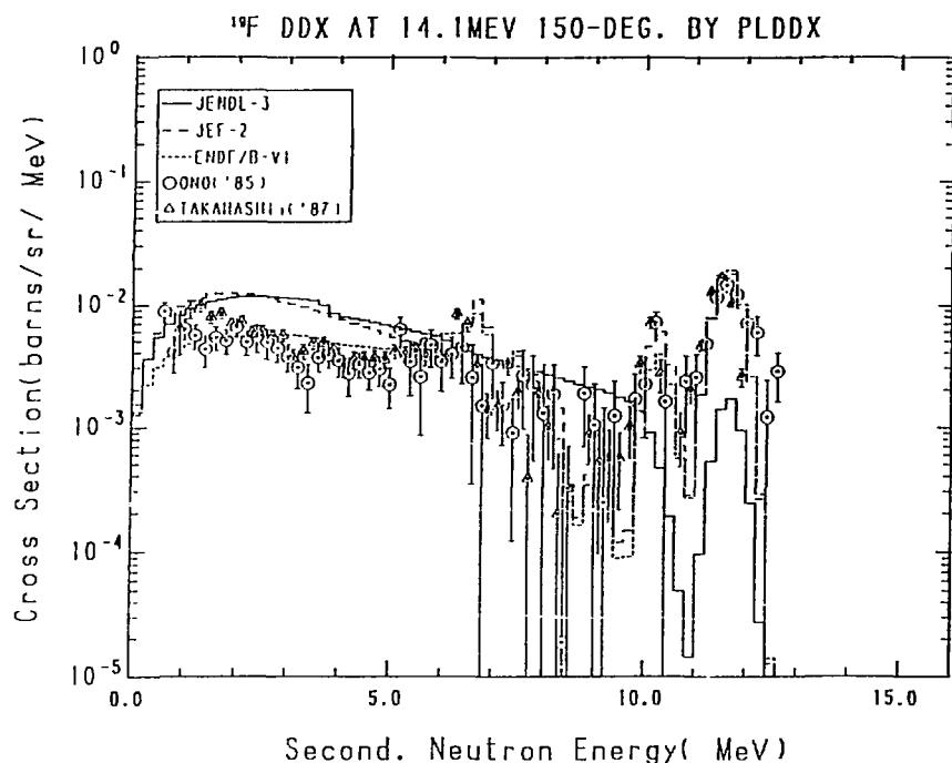
Fig. 17-5 The <sup>19</sup>F Double Differential Cross Section at 14.1 MeV,
