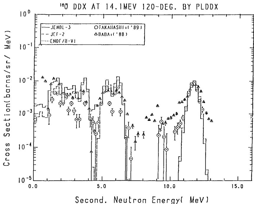
Fig. 15-4 The  $^{160}\text{O}$  Double Differential Cross Section at 14.1 MeV,
