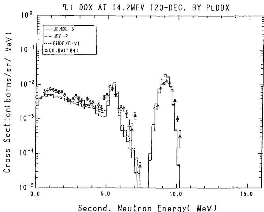
Fig. 6-4 The  $^7\text{Li}$  Double Differential Cross Section at 14.2 MeV,
