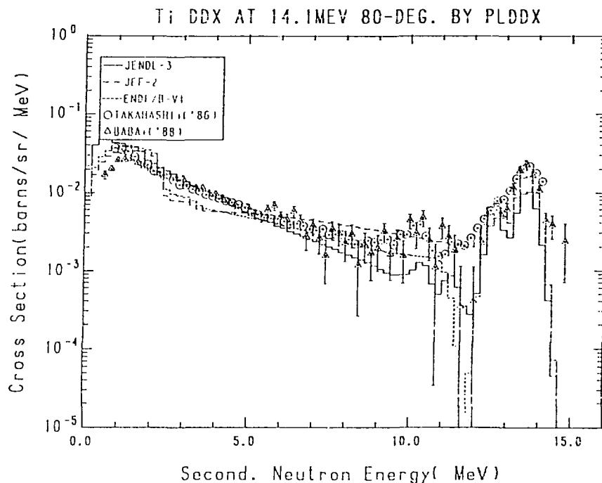
Fig. 25-3 The Titanium Double Differential Cross Section at 14.1 MeV,
