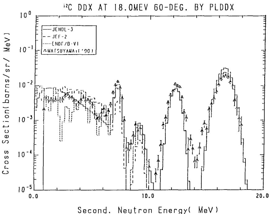
Fig. 12-2 The  $^{12}\text{C}$  Double Differential Cross Section at 18.0 MeV,
