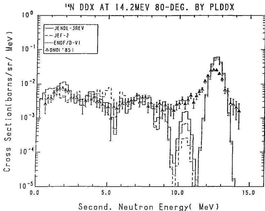
Fig. 13-3 The  $^{14}\text{N}$  Double Differential Cross Section at 14.2 MeV,
