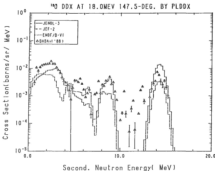
Fig. 16-5 The <sup>160</sup> Double Differential Cross Section at 18.0 MeV,
