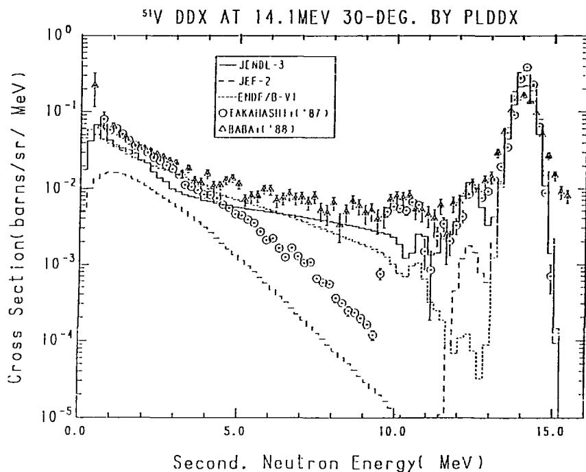
Fig. 26-1 The  $^{51}\text{V}$  Double Differential Cross Section at 14.1 MeV,
