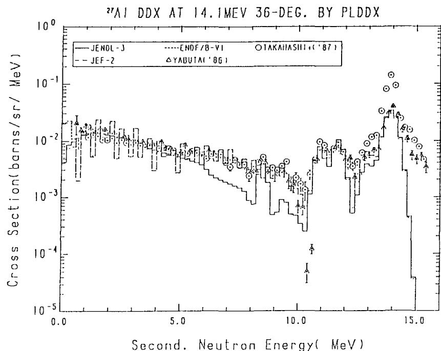
Fig. 20-1 The  $^{27}\text{Al}$  Double Differential Cross Section at 14.1 MeV,
