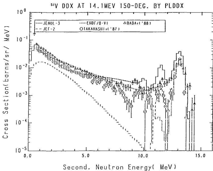
Fig. 26-5 The  $^{51}\text{V}$  Double Differential Cross Section at 14.1 MeV,
