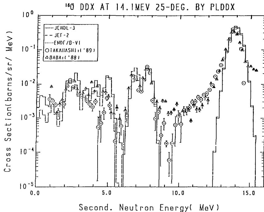
Fig. 15-1 The  $^{160}\text{O}$  Double Differential Cross Section at 14.1 MeV,
