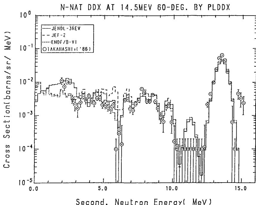
Fig. 14-2 The  $^{nat}N$  Double Differential Cross Section,
