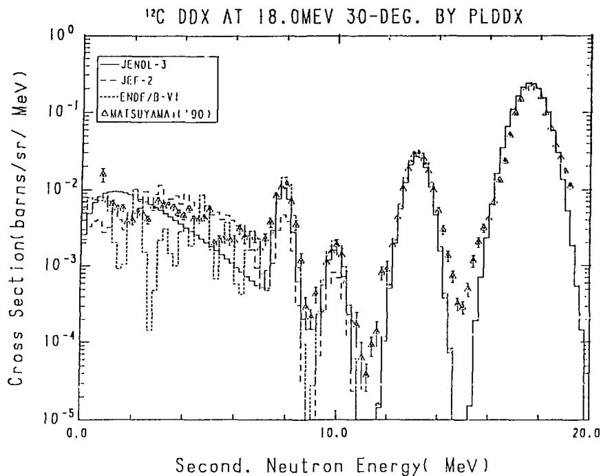
Fig. 12-1 The  $^{12}\text{C}$  Double Differential Cross Section at 18.0 MeV,
