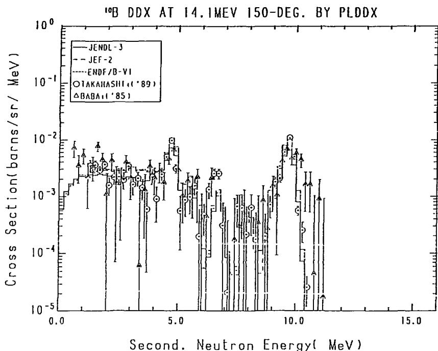
Fig. 9-5 The  $^{10}\text{B}$  Double Differential Cross Section at 14.1 MeV,
