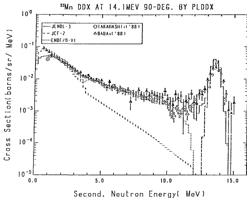
Fig. 28-3 The  $^{55}\text{Mn}$  Double Differential Cross Section at 14.1 MeV,
