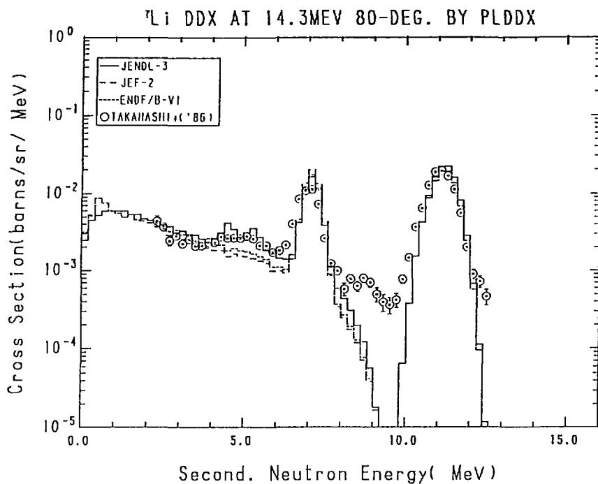
Fig. 7-3 The  $^7\text{Li}$  Double Differential Cross Section,
