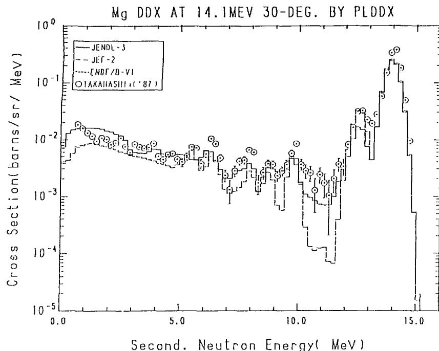
Fig. 19-1 The Magnesium Double Differential Cross Section at 14.1 MeV,
