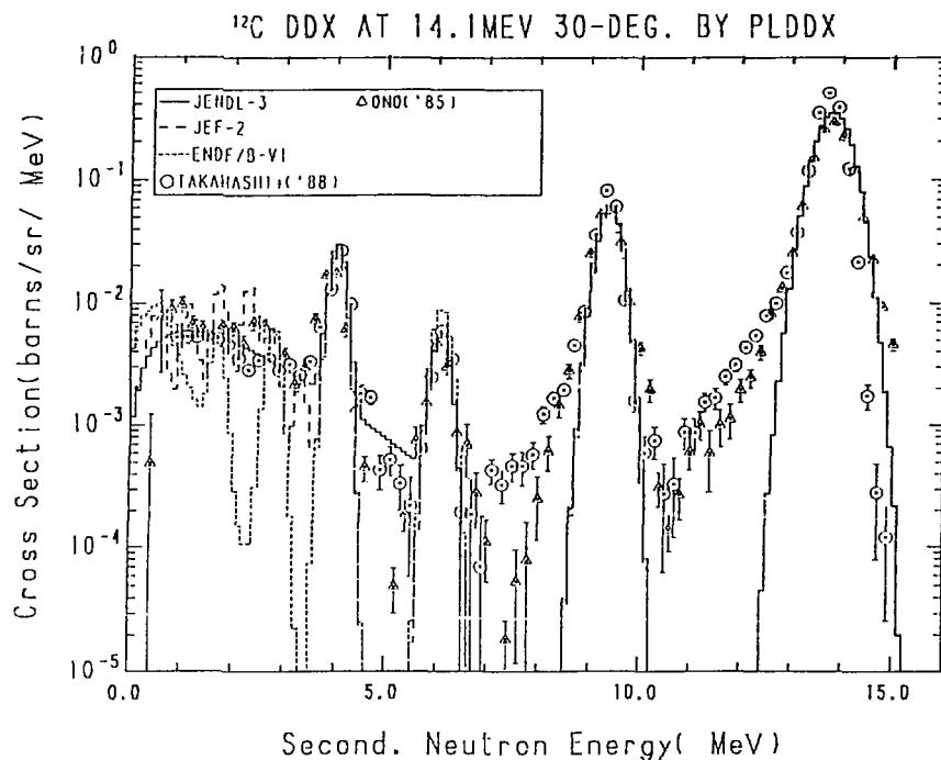
Fig. 11-1 The  $^{12}\text{C}$  Double Differential Cross Section at 14.1 MeV,
