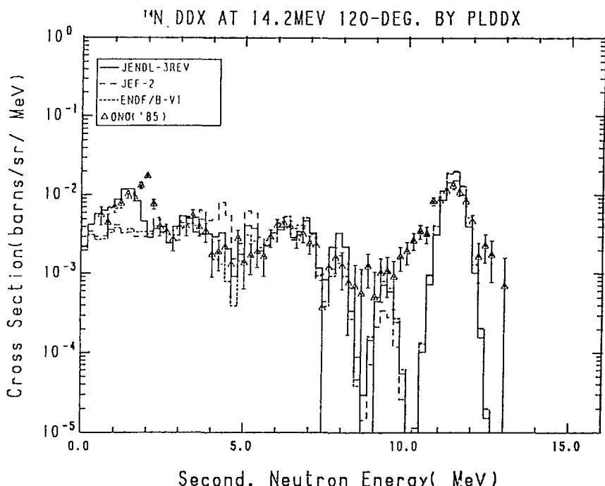
Fig. 13-4 The  $^{14}\text{N}$  Double Differential Cross Section at 14.2 MeV,
