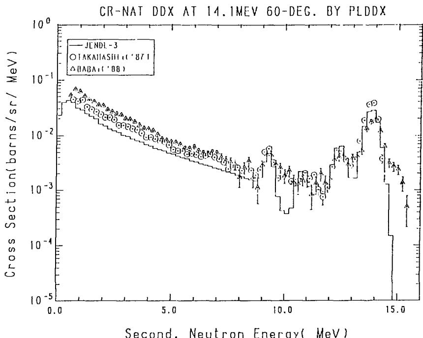
Fig. 27-2 The  $^{nat}\text{Cr}$  Double Differential Cross Section at 14.1 MeV,
