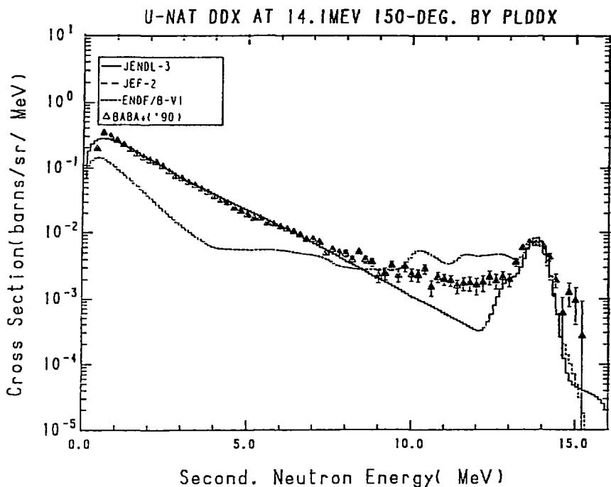
Fig. 55-5 The  $^{nat}U$  Double Differential Cross Section at 14.1 MeV,
