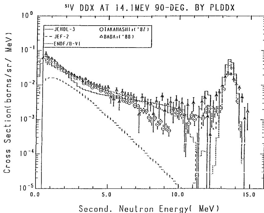
Fig. 26-3 The  $^{51}\text{V}$  Double Differential Cross Section at 14.1 MeV,
