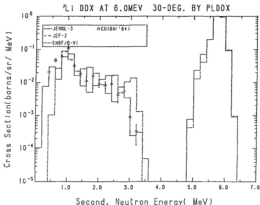
Fig. 5-1 The  ${}^7\text{Li}$  Double Differential Cross Section at 6.0 MeV,
