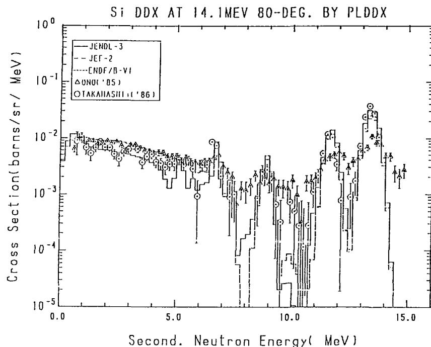
Fig. 22-3 The Silicon Double Differential Cross Section at 14.1 MeV,
