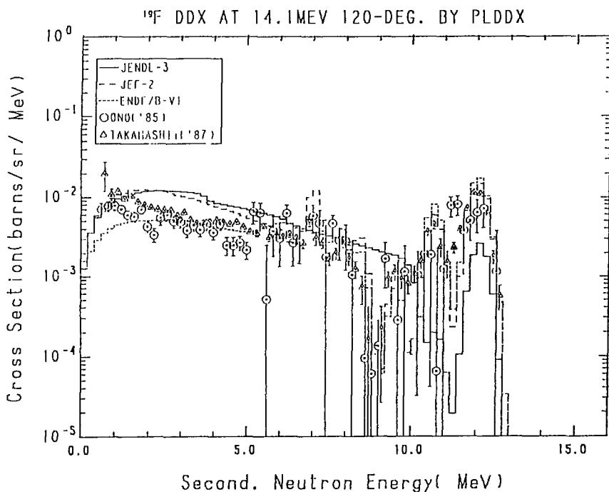
Fig. 17-4 The <sup>19</sup>F Double Differential Cross Section at 14.1 MeV,
