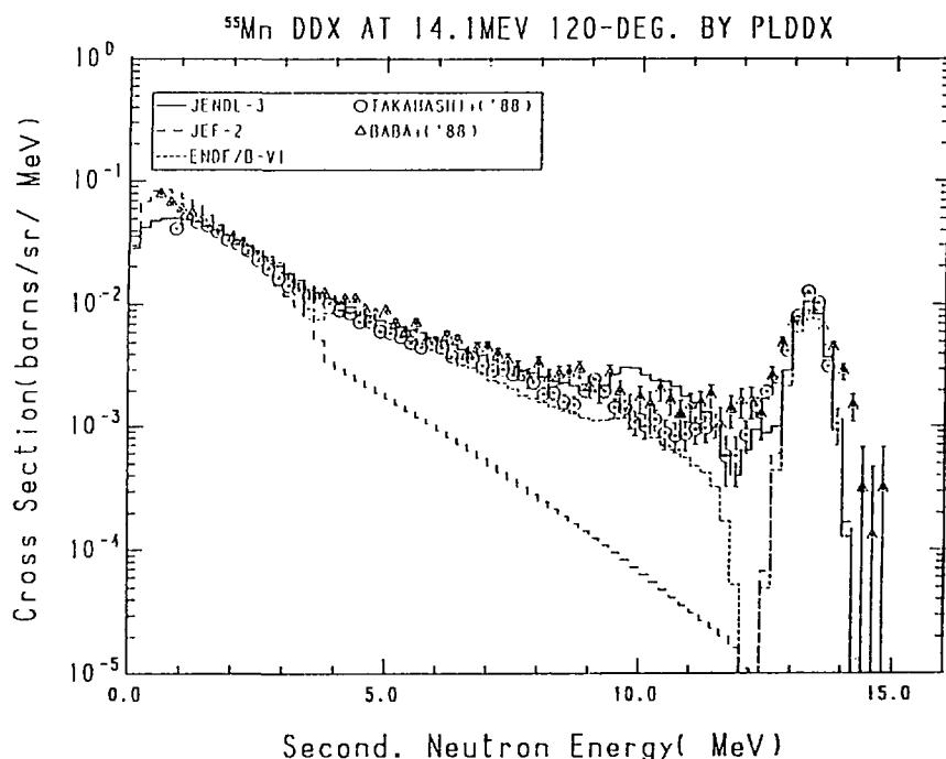
Fig. 28-4 The  $^{55}\text{Mn}$  Double Differential Cross Section at 14.1 MeV,
