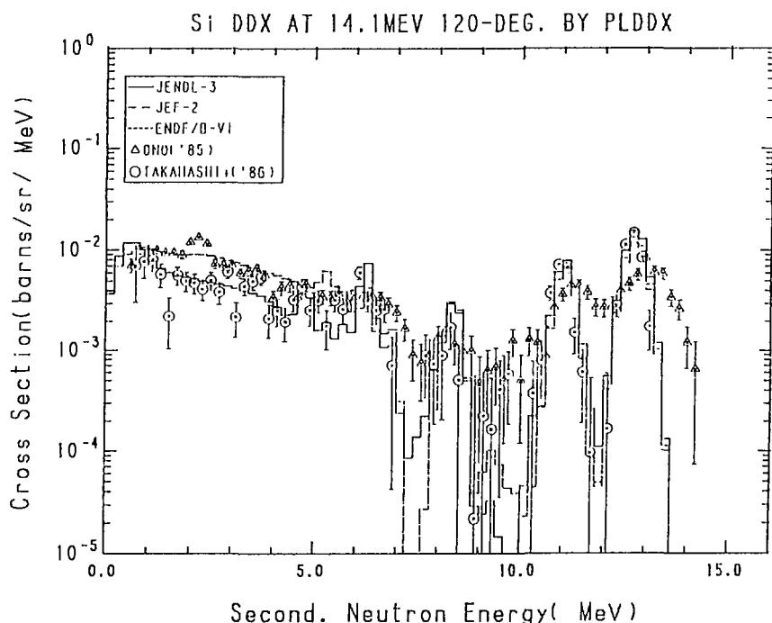
Fig. 22-4 The Silicon Double Differential Cross Section at 14.1 MeV,
