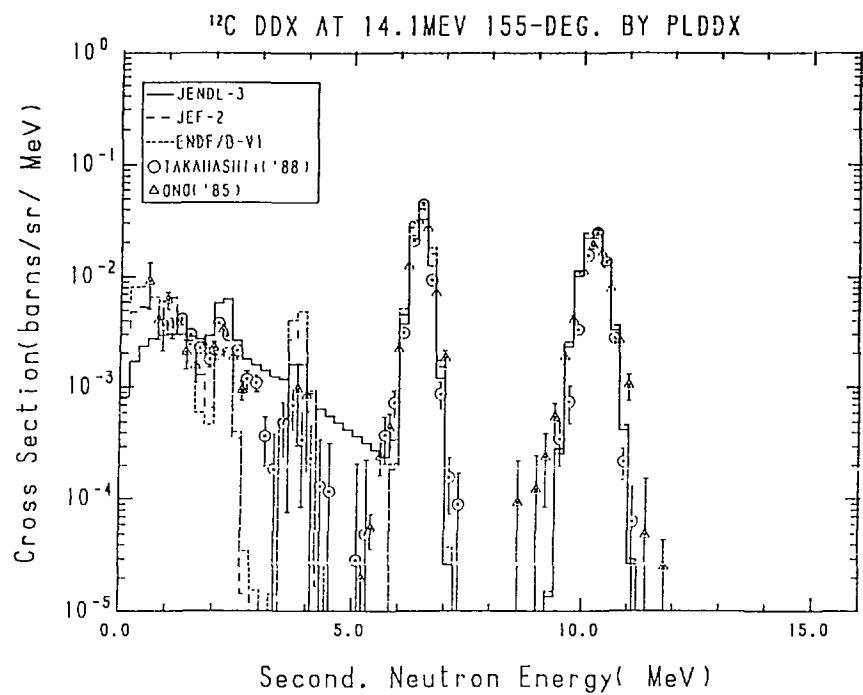
Fig. 11-5 The  $^{12}\text{C}$  Double Differential Cross Section at 14.1 MeV,
