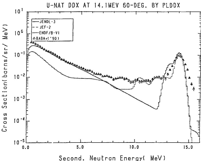
Fig. 55-2 The  $^{nat}U$  Double Differential Cross Section at 14.1 MeV,
