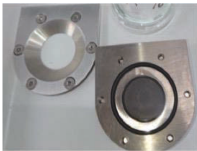
Figure 1: BL15 assembly-type cell and HCP sample. The HCP sample was sandwiched between two quartz windows.
