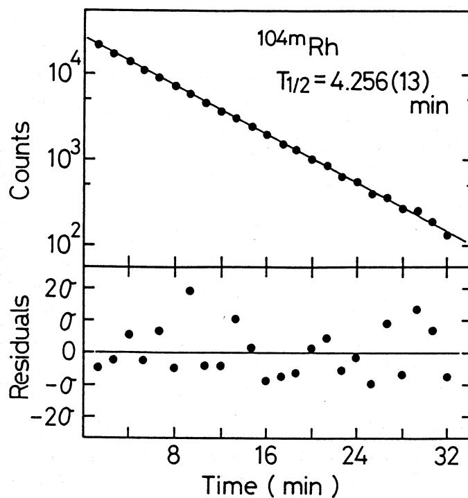
Fig. 14 Decay curve of  $4.3\text{m }^{104}\text{Rh}$  and residuals obtained from a least squares fitting analysis.
