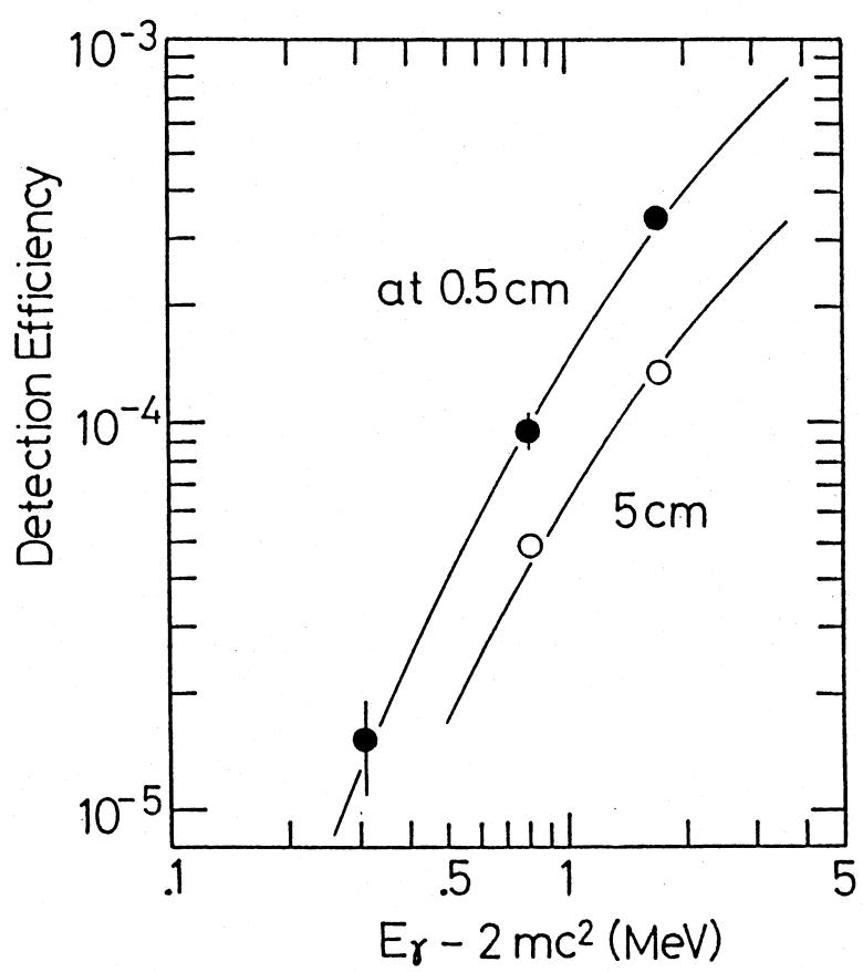
Fig. 10 Detection efficiency of a 12% high-purity Ge detector for 511 keV annihilation  $\gamma$ -rays due to electron-positron-pair production in the shielding box. The fitted lines show pair production cross section for iron in arbitrary units<sup>11</sup>.
