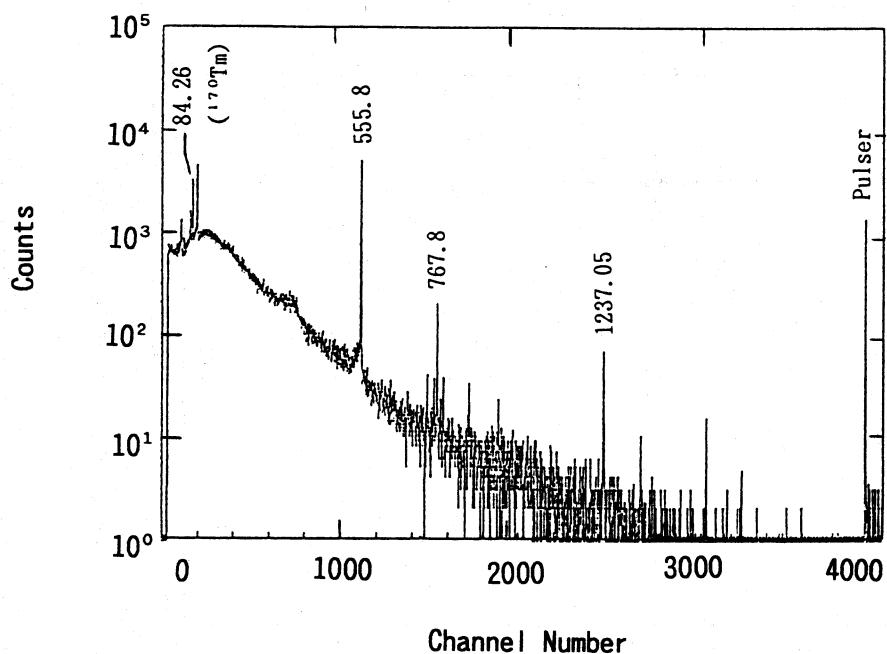
Fig. 13 Gamma-ray spectrum in the decay of  $^{104\text{m}}\text{Rh}$ . Gamma-rays from  $^{170}\text{Tm}$  and pulses were simultaneously measured for the correction of pile-up losses.
