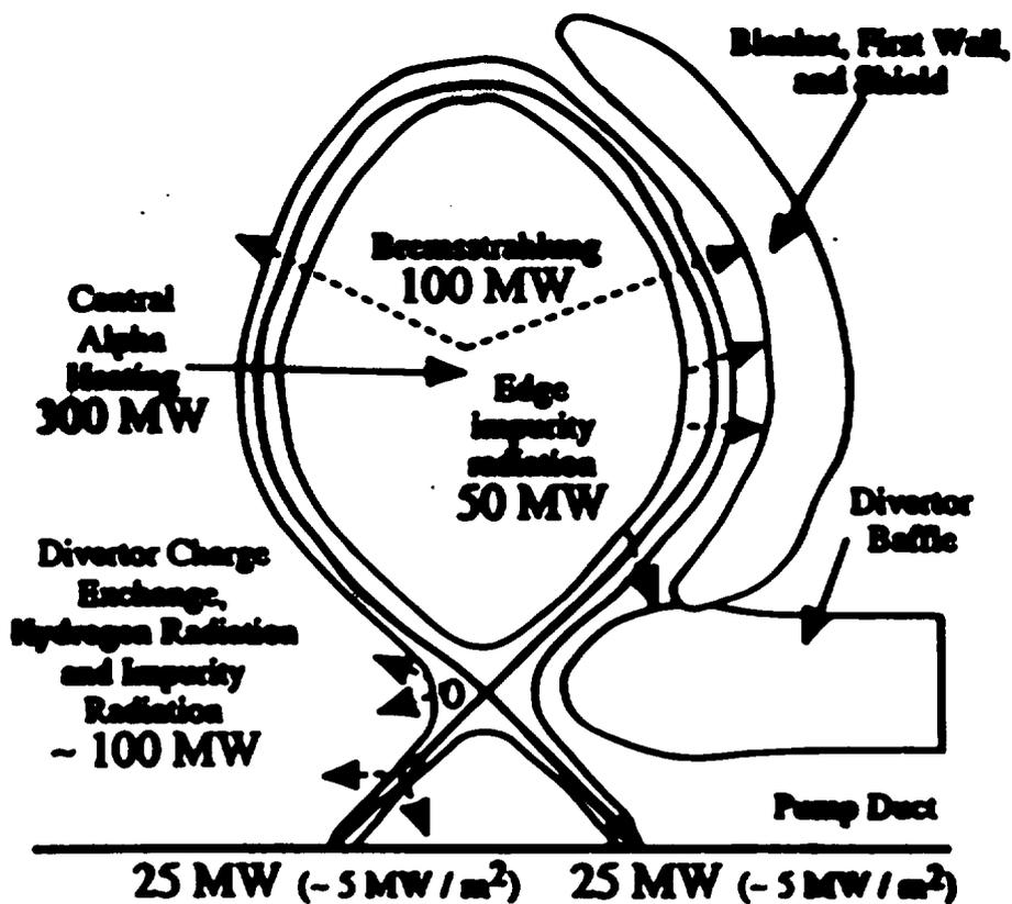
Conducted and Convected power onto the divertor plate
