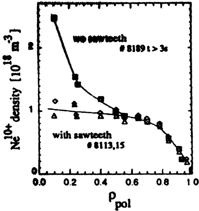
profiles of fully ionised neon from CXRS for standard CDH and without sawtooth activity. Both discharges have the same bulk plasma, where the neon-density is rather similar, but the dilution is strongly improved with sawteeth.
