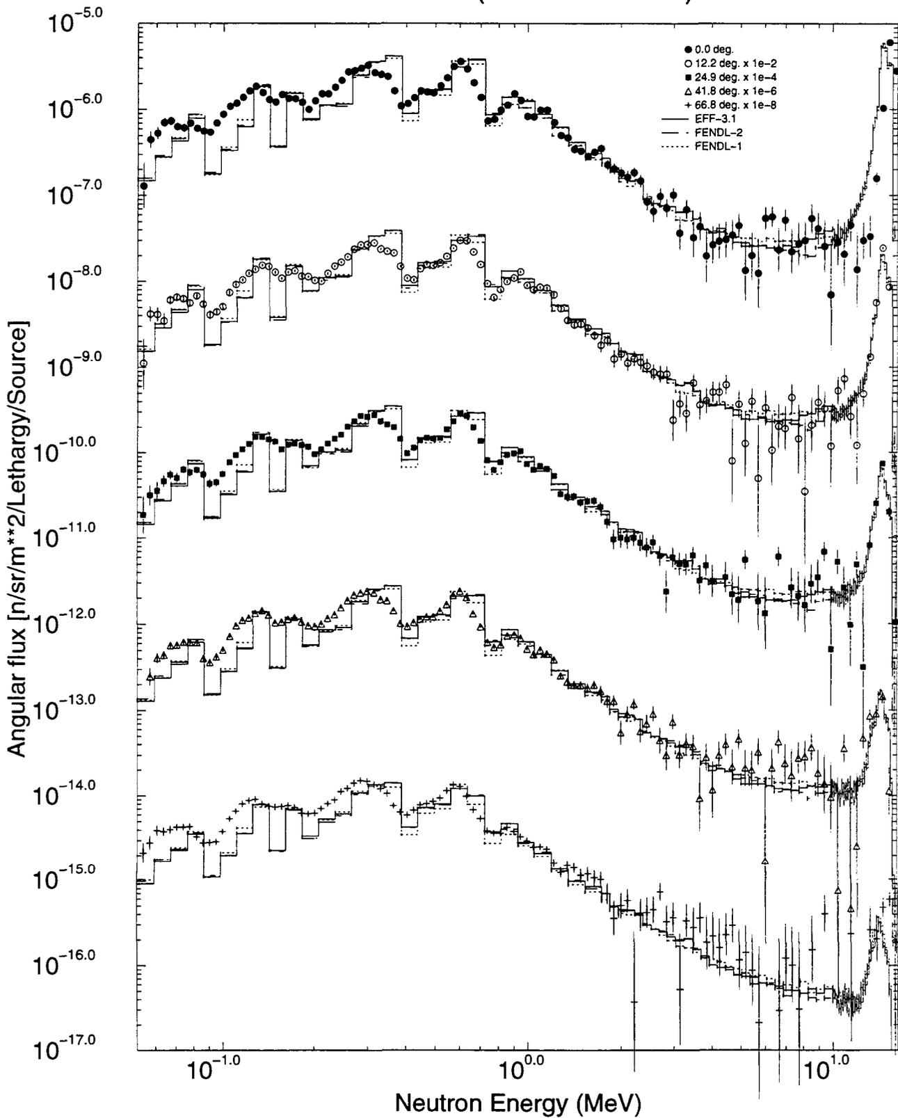
Fig. 2b: Results of MCNP calculations at the FNS-TOF 40 cm cylindrical Iron slab experiment in the energy range 0.05-16.5 MeV, with Iron data from EFF-3.1, FENDL-2 and FENDL-1.
