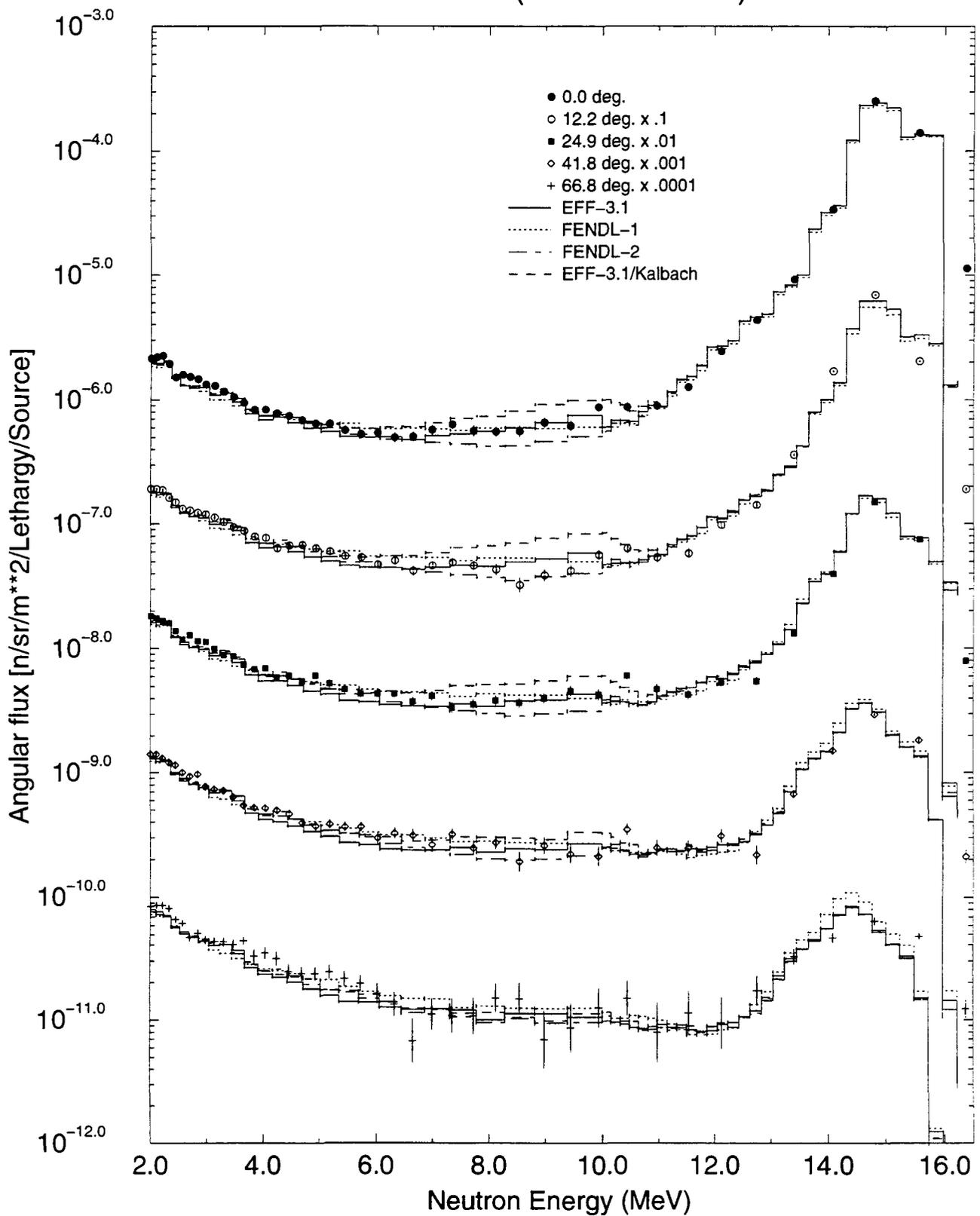
Fig. 1: MCNP calculations at the FNS-TOF 20 cm Iron slab benchmark experiment with Iron data from EFF-3.1, FENDL-2 and FENDL-1 in the energy range 2.0-16.5 MeV.
