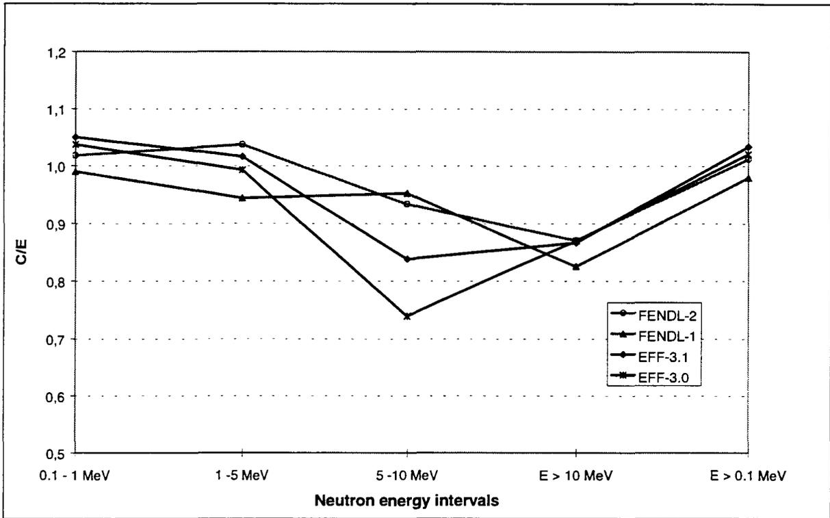
Fig. 2: TUD Iron slab experiment: C/E comparison for neutron flux integrals
