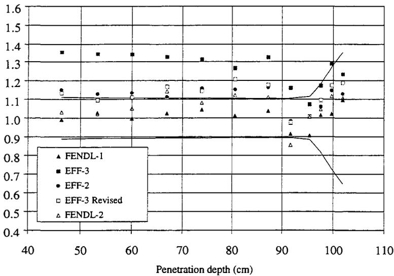
**Fig.1** C/E Comparison for nuclear heating (EFF-3Revised is EFF3.1)
