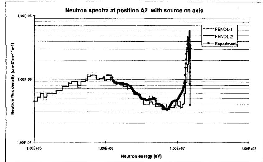
Fig. 2: ITER streaming experiment: comparison of neutron flux spectra at different positions
