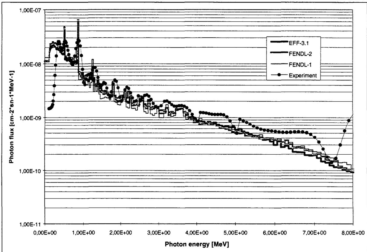
Fig. 3: TUD iron slab experiment: comparison of photon leakage spectra
