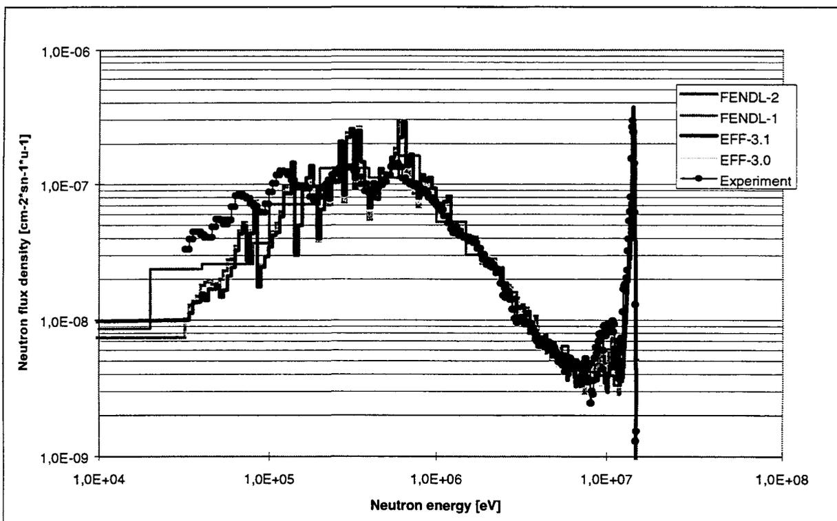
**Fig. 1: TUD Iron slab experiment: comparison of neutron flux spectra**
