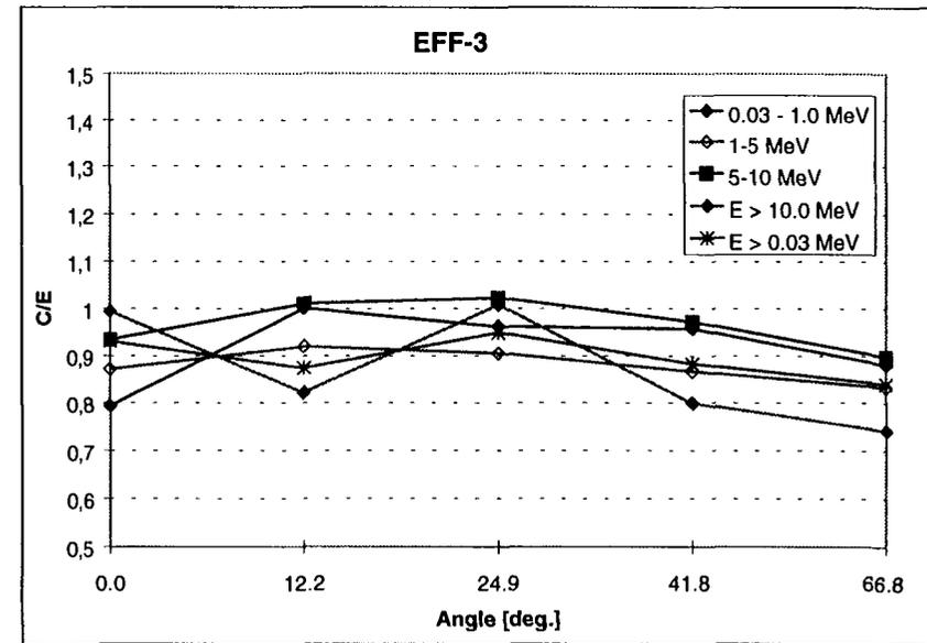
Fig. 2: FNS TOF Beryllium slab [t=15.2 cm] experiment: C/E comparison for neutron flux integrals
