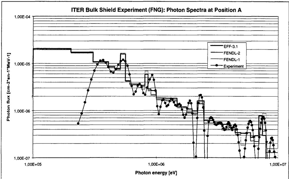
Fig. 4: Photon flux spectra at the back of the shielding blanket mock-up
