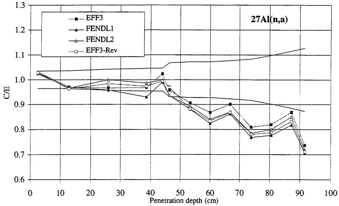
**Fig.3** C/E values for  $^{27}\text{Al}(n,a)$  reaction rate measurements along the mock-up axis (IN AXIS set-up) (EFF.3-rev is EFF3.1)
