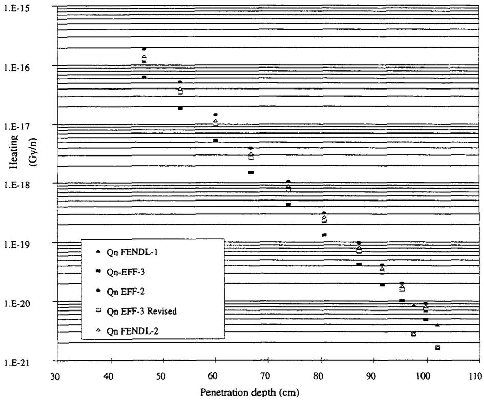
**Fig.3** Calculated neutron heating (EFF-3Revised is EFF3.1)
