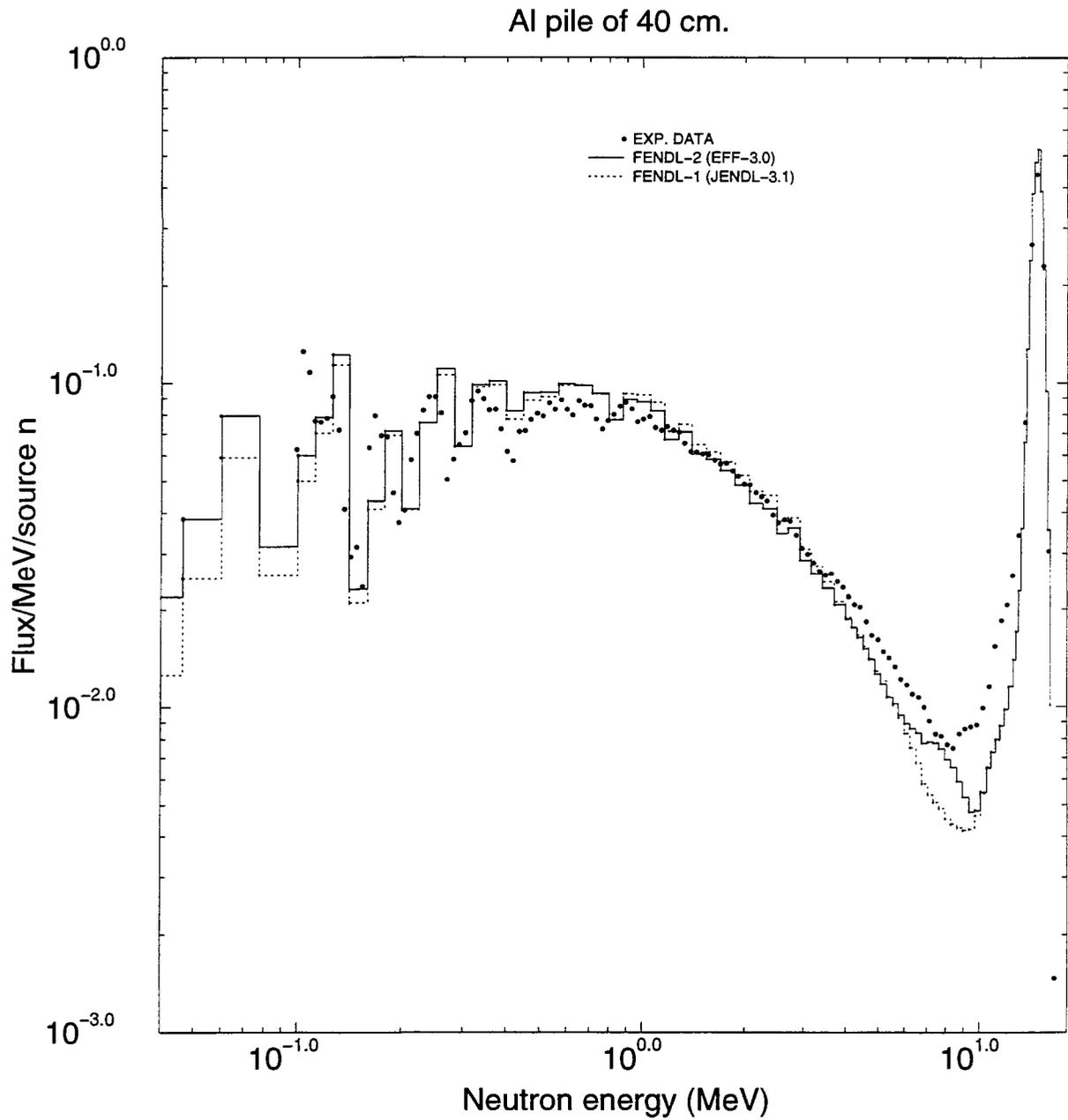
Fig. 1a: MCNP calculations with FENDL-1 (JENDL-3.1) and FENDL-2 (EFF-3.0) data at neutron leakage spectra of OKTAVIAN spherical Aluminium shell experiment.
