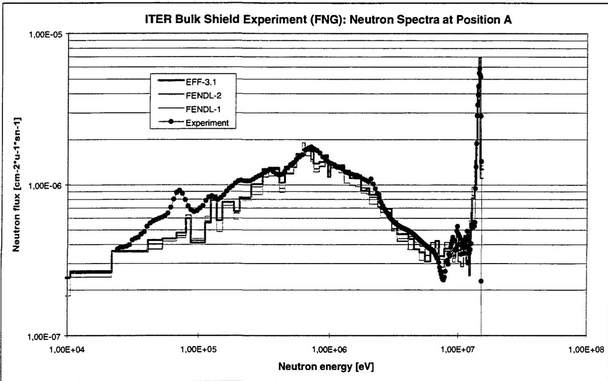
Fig. 2: Neutron flux spectra at the back of the shielding blanket mock-up
