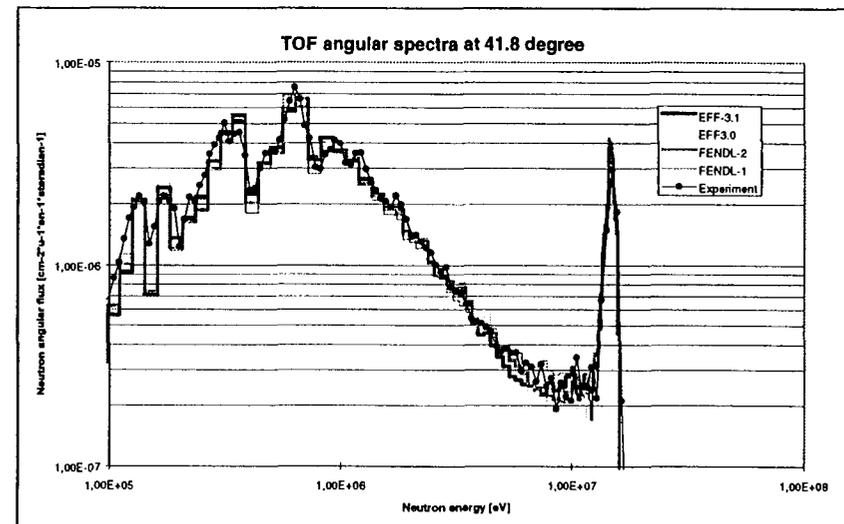
Fig. 5: FNS TOF Iron slab [ $t=20.0$  cm] experiment: comparison of angular neutron flux spectra
