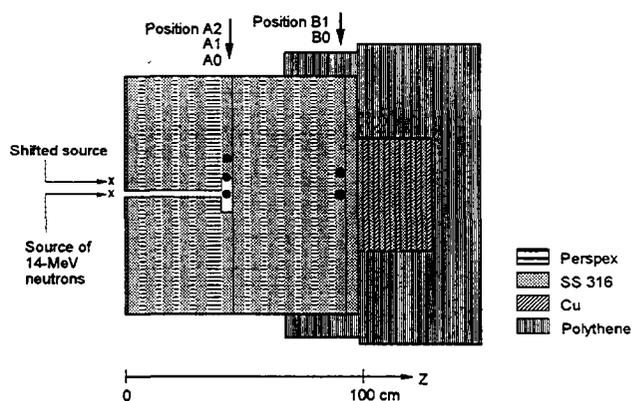
**Fig. 1: ITER mock-up assembly with streaming channel and measurement positions indicated**
