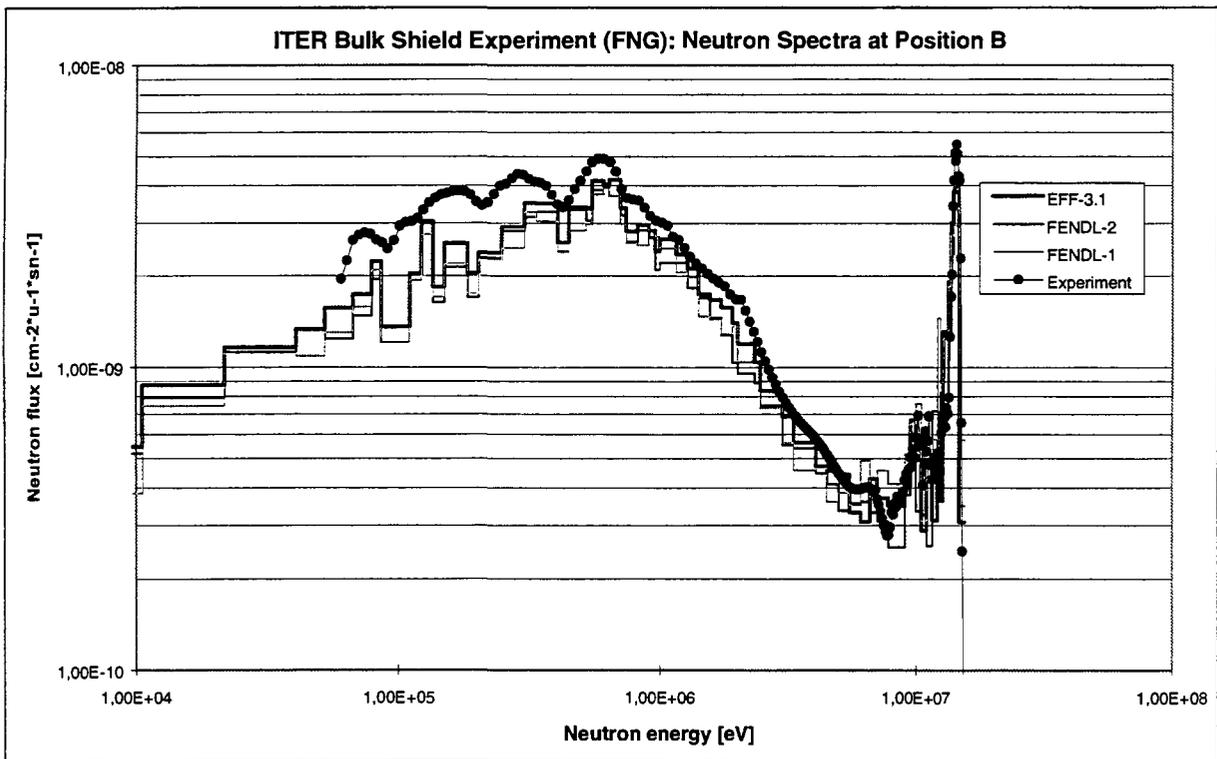
Fig. 3: Neutron flux spectra at the back of the vacuum vessel mock-up
