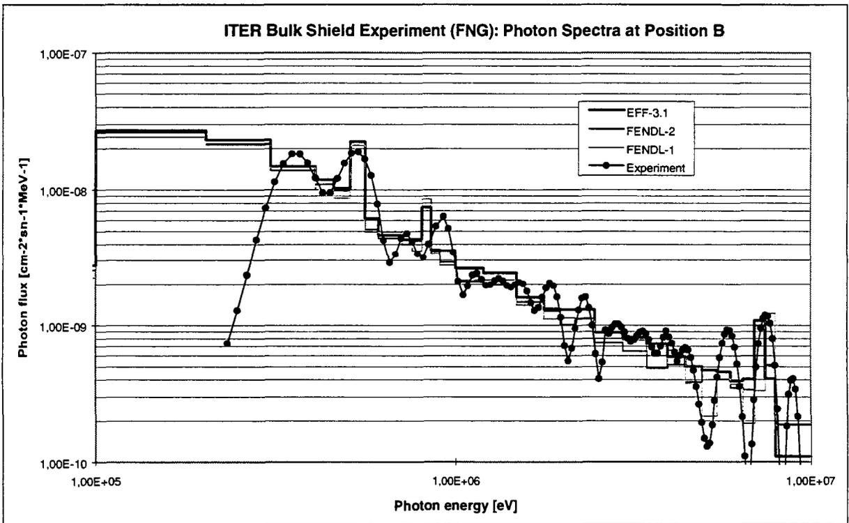
Fig. 5: Photon flux spectra at the back of the vacuum vessel mock-up
