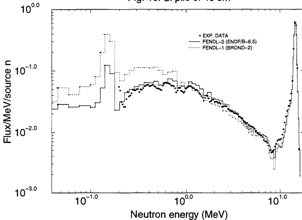
Fig. 1b,c: MCNP calculations with FENDL-1 (BROND-1) and FENDL-2 (ENDF/B-6.5) data at neutron leakage spectra of OKTAVIAN spherical Silicon shell experiments.
