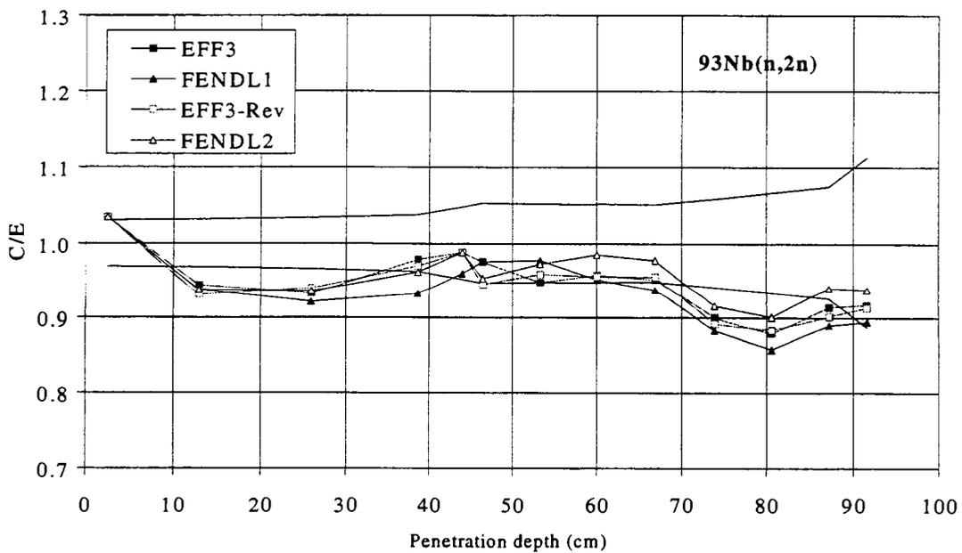
Fig.2 C/E values for  $^{93}\text{Nb}(n,2n)$  reaction rate measurements along the mock-up axis (IN AXIS set-up) (EFF.3-rev is EFF3.1)
