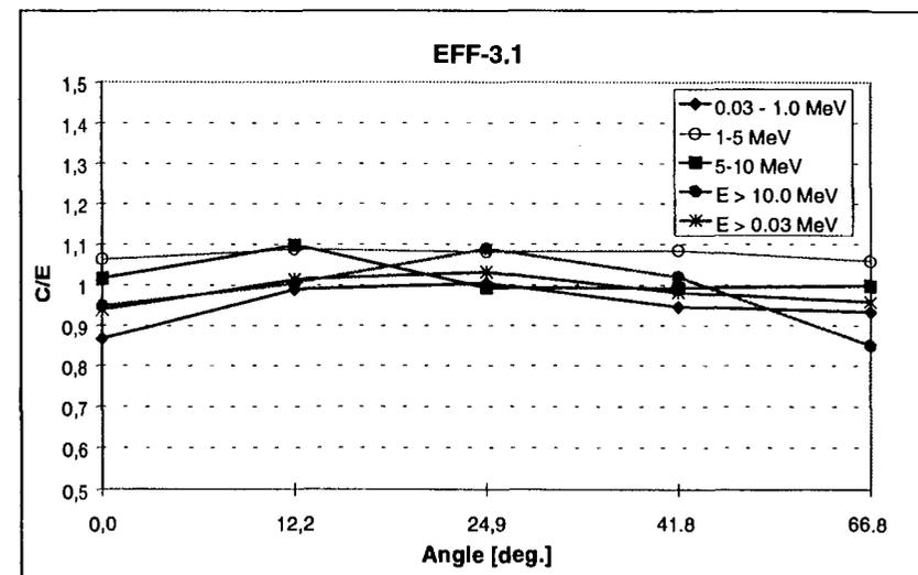
Fig. 4: FNS TOF Iron slab [t=20.0 cm] experiment: C/E comparison for neutron flux integrals
