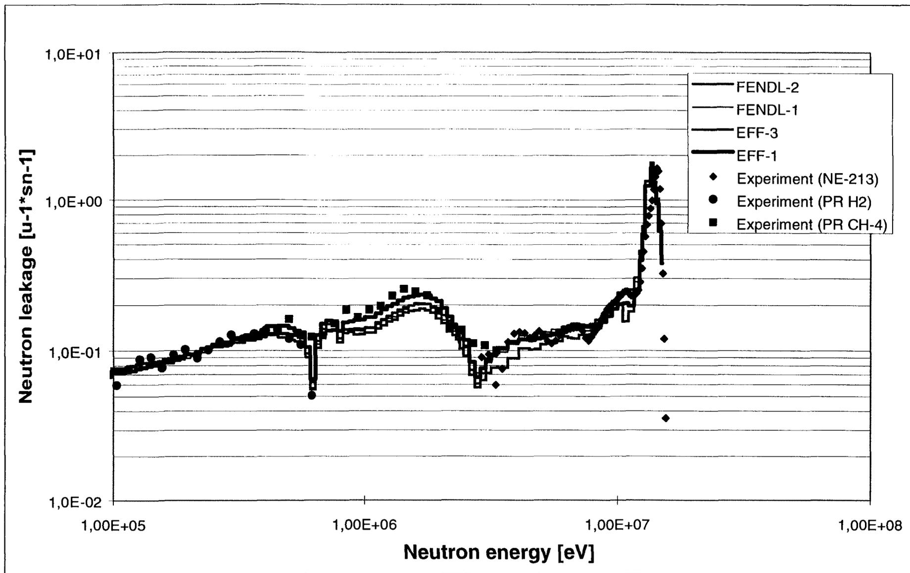
Fig. 1: KANT Beryllium spherical shell experiment [ $r_i = 5$  cm,  $r_o = 22$  cm]: comparison of neutron leakage spectra
