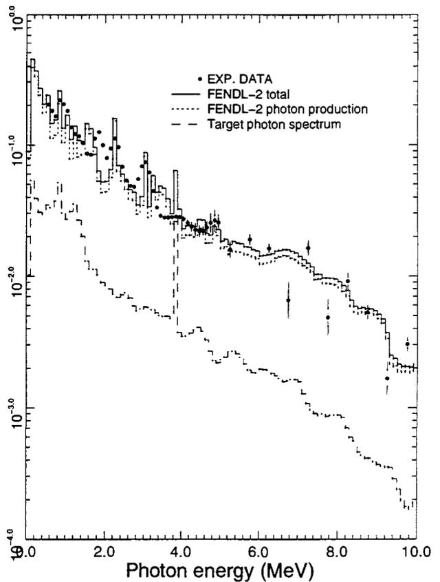
Fig. 2: MCNP calculations with FENDL-1 and FENDL-2 data at gamma leakage spectra of OKTAVIAN spherical shell experiments.
