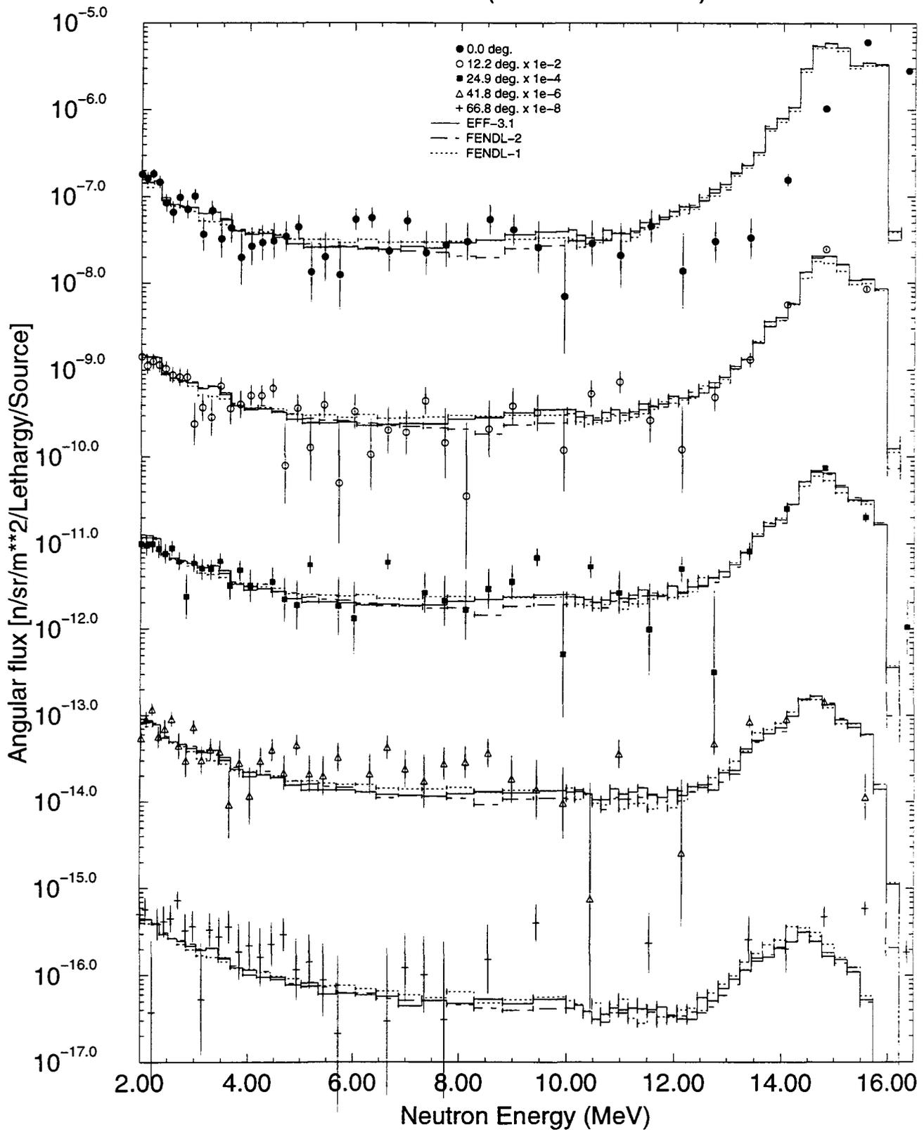
Fig. 2a: Results of MCNP calculations at the FNS-TOF 40 cm cylindrical Iron slab experiment in the energy range 2.0-16.5 MeV, with Iron data from EFF-3.1, FENDL-2 and FENDL-1.
