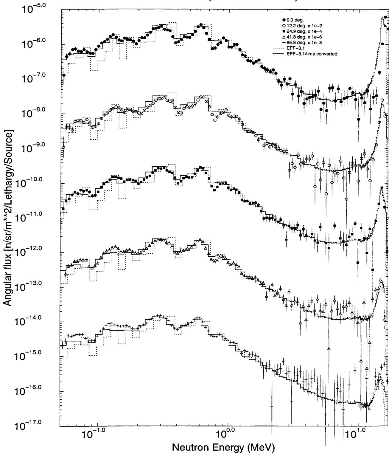
Fig. 2c: MCNP calculations with Iron data from EFF-3.1 at the FNS-TOF 40 cm slab benchmark experiment in the neutron-energy range 0.05 - 16.5 MeV. Dotted line: results of conventional MCNP calculation. Solid line: results obtained by converting the calculated time of arrival spectra into neutron energy spectra, as described in the text.
