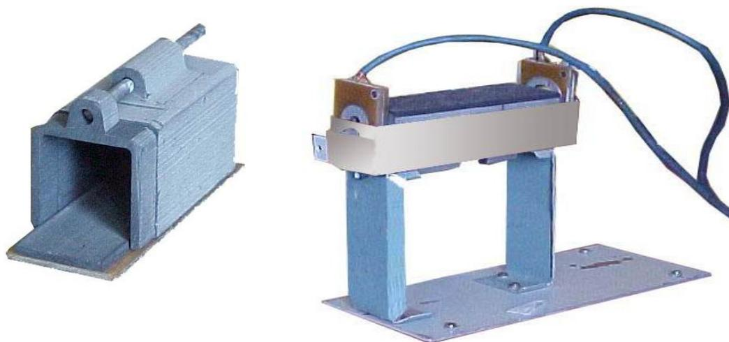
Fig. 2. Telescope of detectors - detector cells are pulled out, and the analyzed sample is displaced. Telescope made of graphite is shown on the left-hand side.
