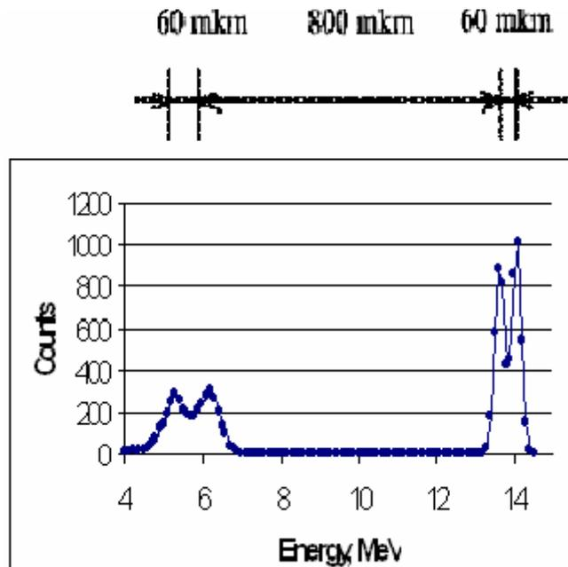
Fig. 12. Energy spectrum of protons simulated for a sample containing short-distance hydrogen-containing layers of  $\text{CH}_2$ .
