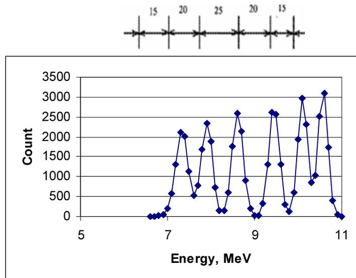
Fig. 13. Energy spectrum of tritons simulated for a complex titanium sample that contains TiT layers.
