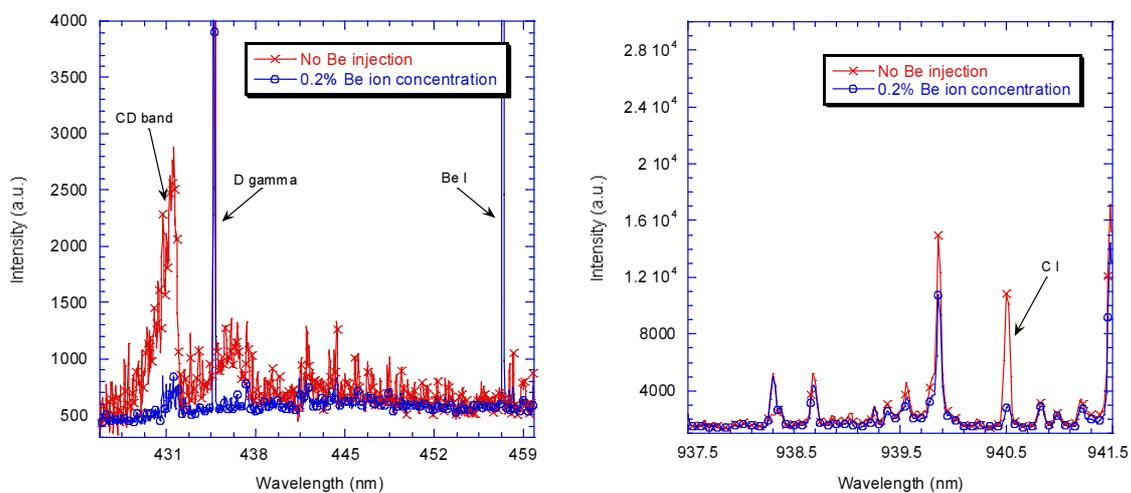
Fig. 1. Beryllium impurity seeding of the incident deuterium plasma reduces both (a) chemical erosion, and (b) physical sputtering of graphite target plates.
