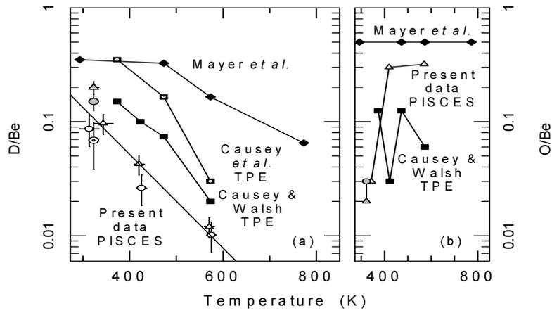
Fig. 3. Deuterium retention in witness plate samples collected during Be seeded plasma exposures.
