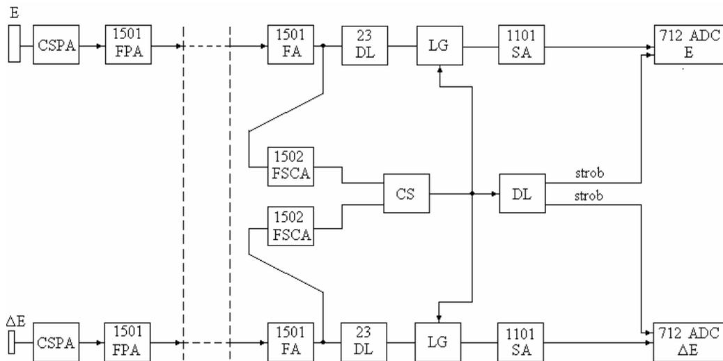
Fig. 6. Block diagram of the spectrometer.
