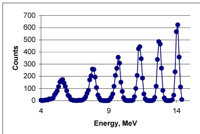
Fig. 11. Simulated energy spectrum of protons - neutron irradiation of a complex hydrogen-containing sample consisting of six films of  $\text{CH}_2$ .
