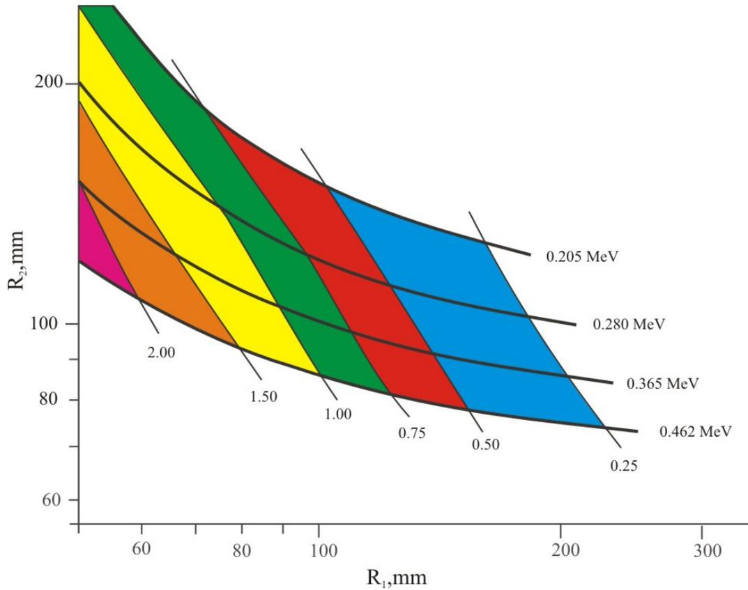
Fig. 5. Topography of the energy resolution and count rate calculated for apertures of  $\Delta E$  and  $E$ -detector  $\varnothing 8$  and  $\varnothing 16$  mm, respectively.
