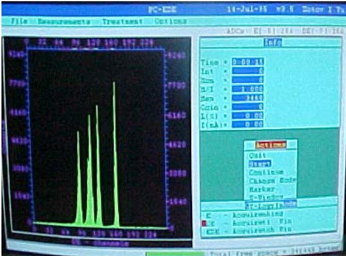
Fig. 10. Energy spectrum of alpha particles.
