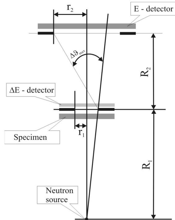
Fig. 4. Geometry of the spectrometer - a specimen is situated as close as possible to the first  $\Delta E$  detector.
