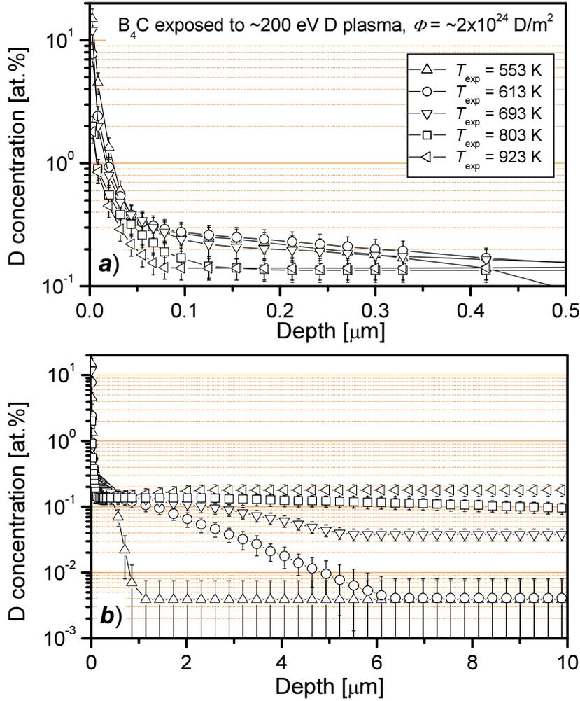
Fig. 1. Depth profiles of deuterium trapped in the near-surface layer (a) and in the bulk (b) of  $B_4C$  exposed to a low-energy ( $\approx 200$  eV/D) deuterium plasma to a fluence of about  $2 \times 10^{24}$   $D/m^2$  at different temperatures. The D concentration up to  $0.5 \mu m$  (a) was determined from the energy spectra of  $\alpha$  particles emitted from the  $D(^3He, \alpha)H$  reaction. Note that the depth and concentration scales in parts (a) and (b) are different.
