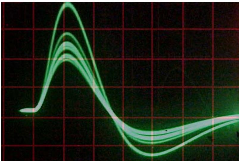
Fig. 9. Shape of pulses on output of the spectrometric amplifier 1101 - rise time of the pulse is 1  $\mu$ s.
