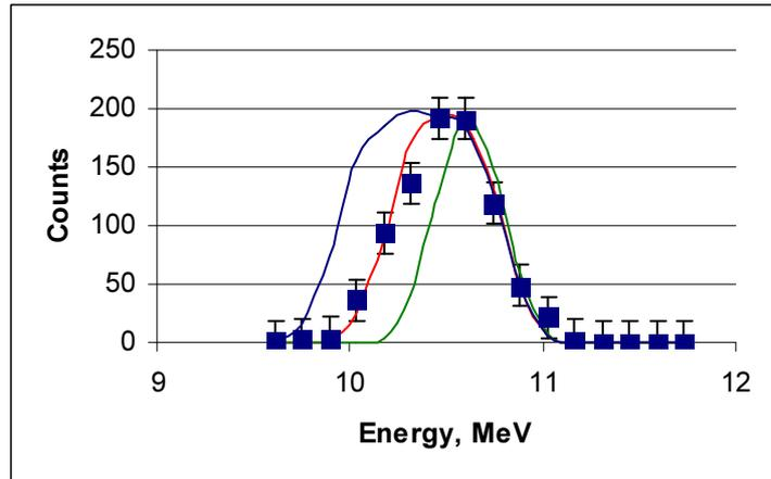
Fig. 14. The experimental energy distribution of tritons (measurement #527) and Monte-Carlo simulation for three different thicknesses of tritium location: 20 (green), 25 (red), 30 (blue) microns. Points with error bars are experimental values.
