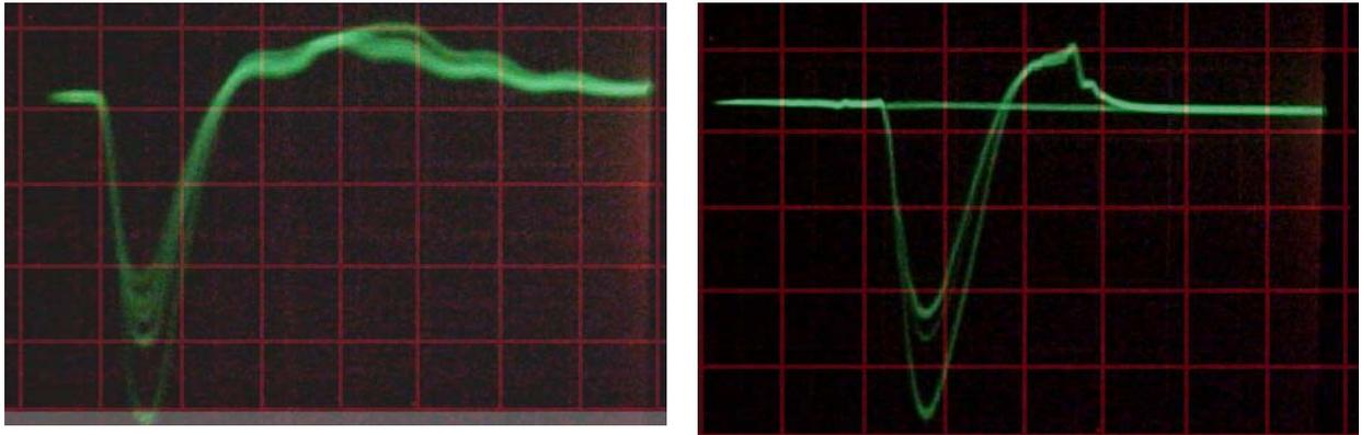
Fig. 8. Pulse shape of fast amplifier (left) and fast gate output signals - rise time of the pulse is 70 ns.
