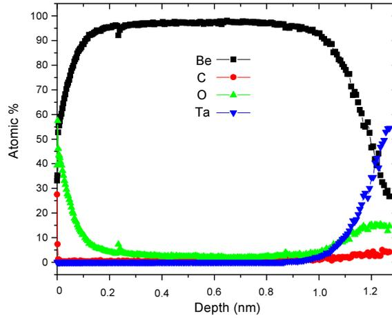
Fig. 2. Depth profile of the composition of a tantalum witness plate sample used to collect re-deposited material during exposure of a 700°C graphite sample to beryllium containing, deuterium plasma.
