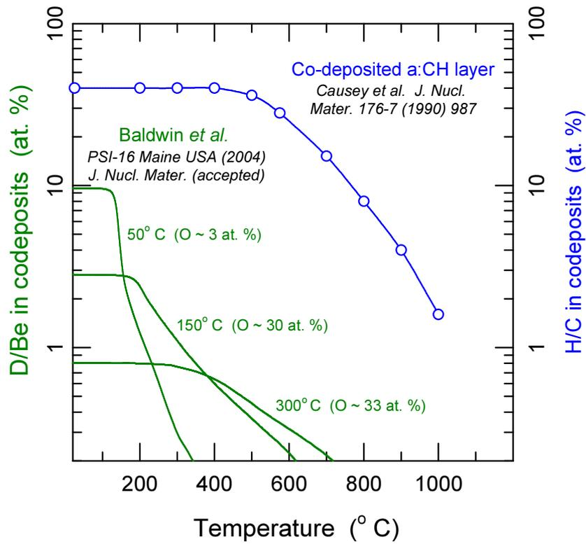
Fig. 4. Thermal release behavior of co-deposited Be films compared with co-deposited carbon films.
