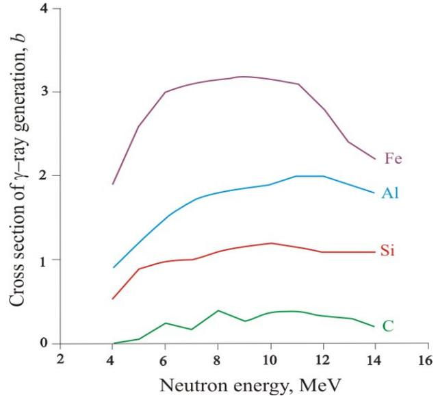
Fig 1. Total cross-sections of gamma-ray generation by neutrons in carbon, aluminum, silicon and iron, as a function of neutron energies.
