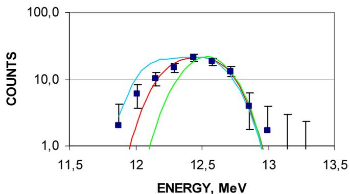
Fig. 15. The experimental energy distribution of deuterons (measurement #527) and the Monte-Carlo simulation for three different thicknesses of deuterium: 25 (green), 35 (red) and 45 (blue) mkm. The best fit is achieved when the tritium thickness is 25 microns.
