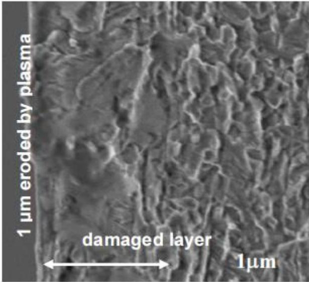
Fig. 5. C-irradiated tungsten cross section (10 MeV,  $2 \times 10^{17} \text{cm}^{-2}$ ) after deuterium plasma (1  $\mu\text{m}$  eroded).
