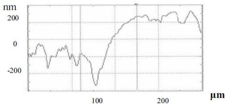
Fig. 3. Boundary of C-ion irradiated area on tungsten sample: the irradiated area is to the right; the left part was masked from irradiation. Surface profile shows elevation of the irradiated part.
