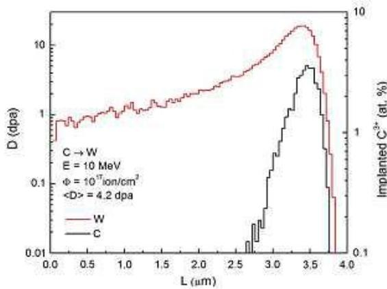
Fig. 2. Primary defect distribution in tungsten irradiated by  $^{12}\text{C}^{+3}$  ions at 10 MeV to fluence of  $10^{17} \text{ ion/cm}^2$ .  $\langle D \rangle = 12.5 \text{ dpa}$  average over damaged layer 3.5  $\mu\text{m}$  in depth.
