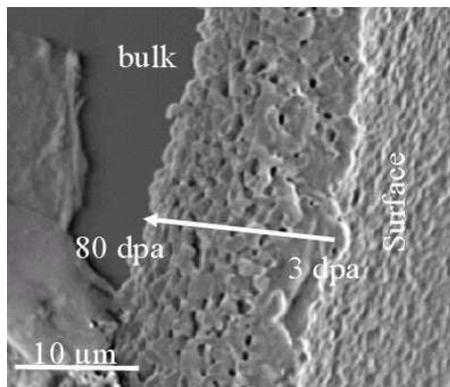
Fig. 1. Surface layer of tungsten damaged by He-ions ( $3 \times 10^{18} \text{ cm}^{-2}$ , 3.5-4 MeV): from 3 dpa at the surface to 80 dpa at 6-micron depth.
