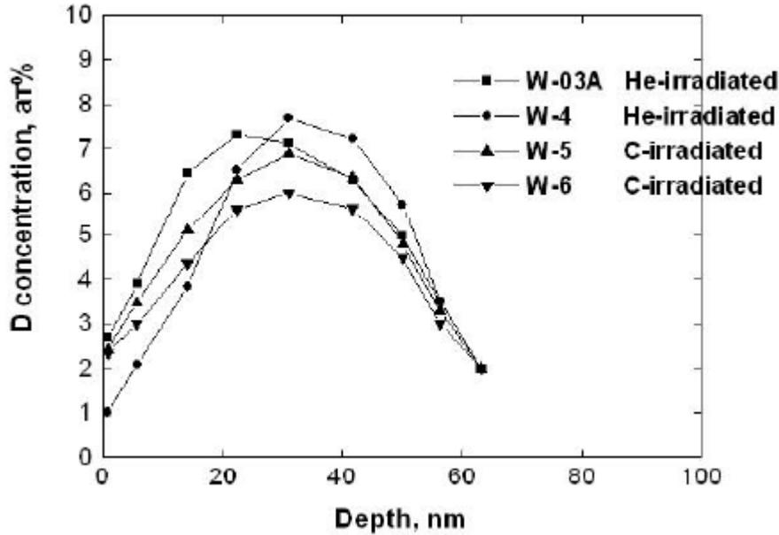
Fig 6. Deuterium concentrations (ERDA) in damaged plasma exposed tungsten: W-03A and W-4 – He-irradiated samples, 2-3 dpa at the surface; W-5 and W-6 – C-irradiated samples 2 dpa at the surface.
