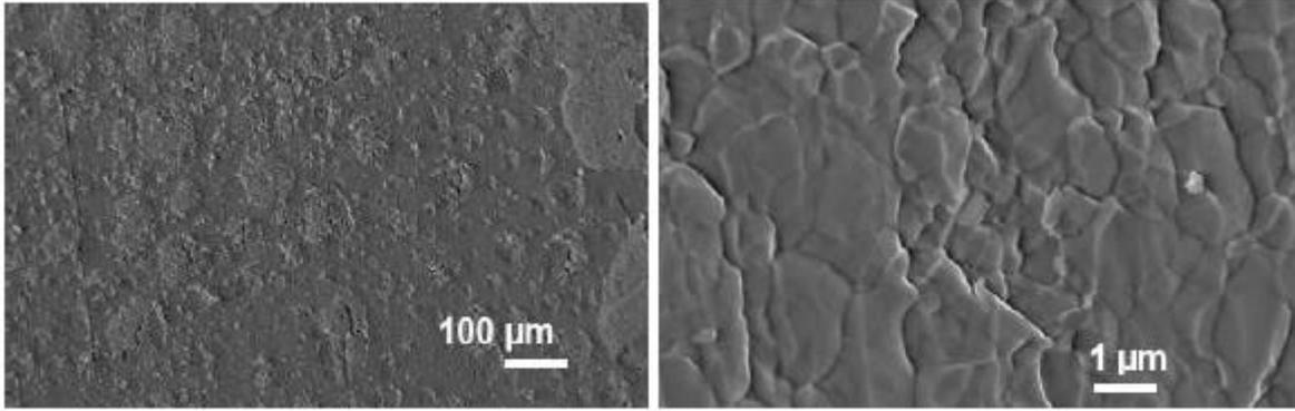
Fig. 4. He-irradiated tungsten ( $3 \times 10^{18} \text{cm}^{-2}$ , 4 MeV): a – surface after irradiation; b –after 4-fold deuterium plasma exposure, 3.6  $\mu\text{m}$  eroded; c, d – after 6-fold plasma, 5.4  $\mu\text{m}$  eroded.
