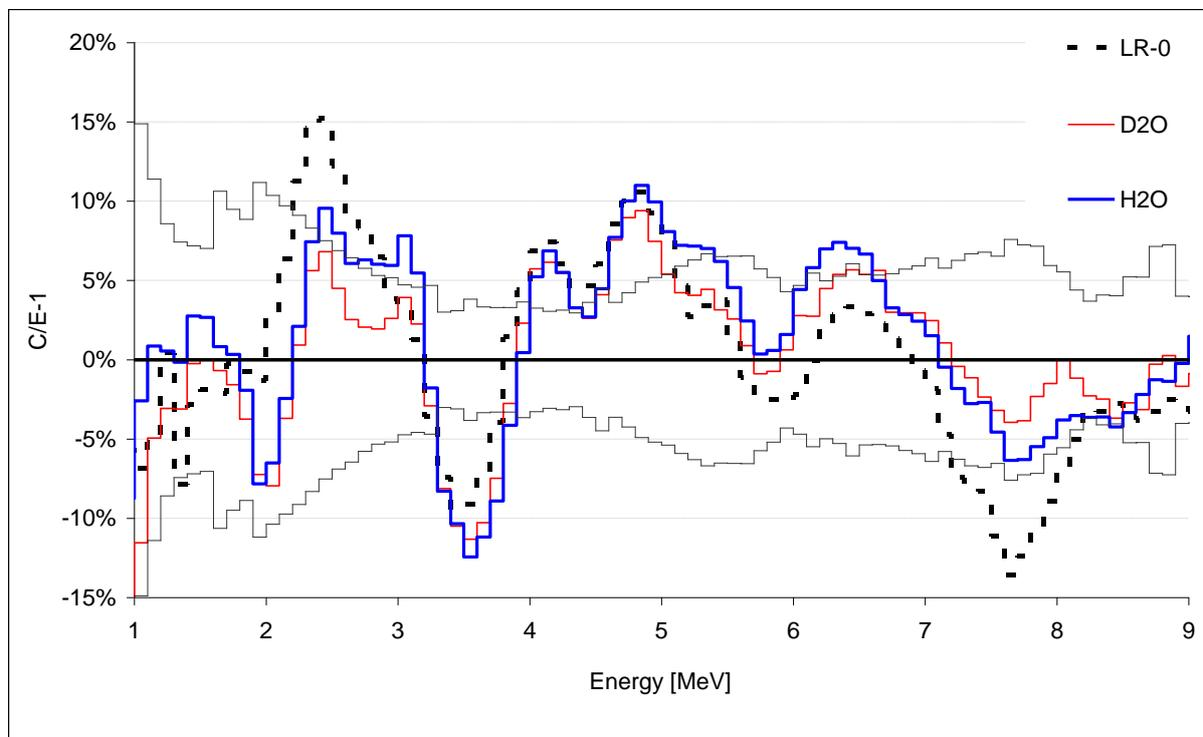
*C/E comparison of neutron leakage spectra from H<sub>2</sub>O/D<sub>2</sub>O sphere, D=30cm, calculation realized with ENDF/B-VII.1*
