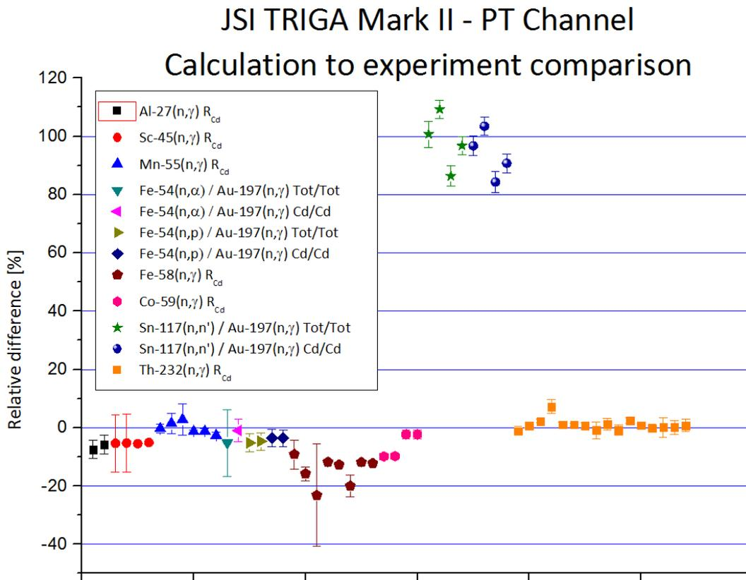
Fig. 10. Relative difference in the measured and calculated  $R_{Cd}$  values and reaction rate ratios
