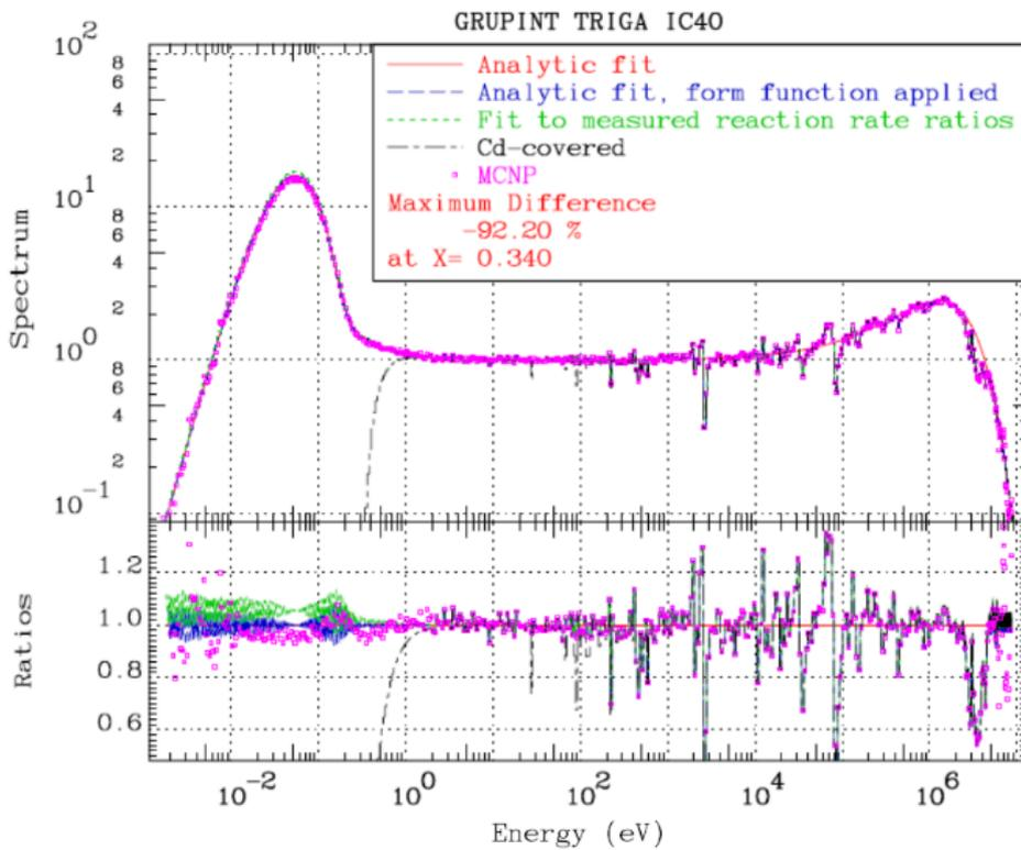
Fig. 6. JSI TRIGA IC40 channel spectrum fitting.
