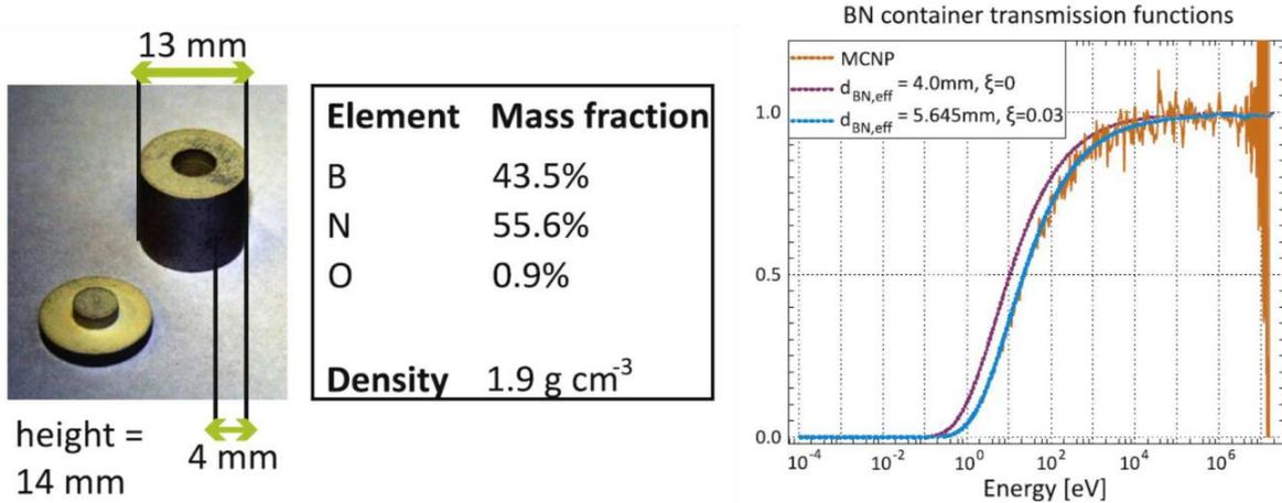
Fig. 11: Boron nitride filter used in the experiments and its transmission function.
