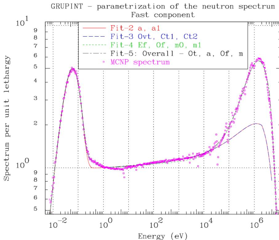
Fig. 3. Fitting the parameters of the fast part to an input spectrum, overall fit.
