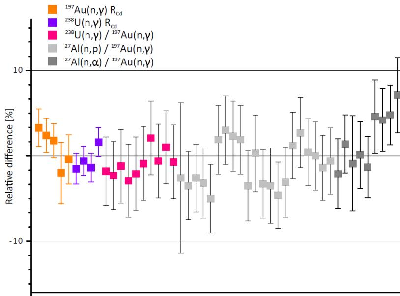
Fig. 7. JSI TRIGA Central Channel – relative differences between measured and calculated reaction rate ratios for nuclear reactions used to characterize the neutron spectrum.
