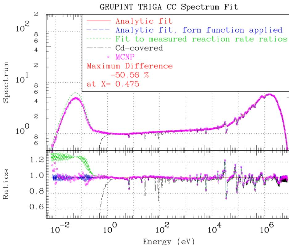
Fig. 4. JSI TRIGA Central Channel spectrum fitting.
