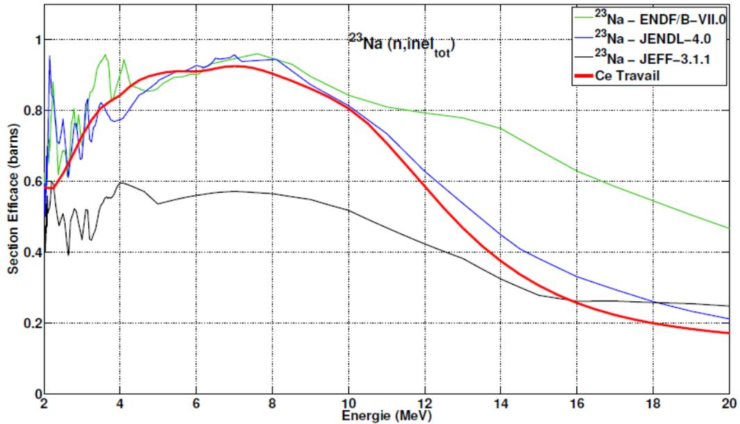
Fig. 1.  $^{23}\text{Na}(n,n')$  cross sections available in different library. The cross section in JEFF-3.1.1 comes from integral data adjustment performed in the frame of the ERALIB libraries. The red curve is equivalent to JEFF-3.2.
