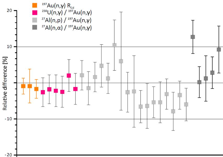
Fig. 9. JSI TRIGA IC40 channel – relative differences between measured and calculated reaction rate ratios for nuclear reactions used to characterize the neutron spectrum.
