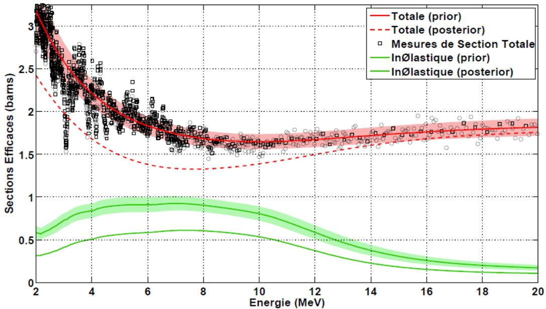
Fig. 2. Adjustment of the  $^{23}\text{Na}$  cross sections with integral experiments performed in the fast reactor MASURCA of CEA Cadarache.
