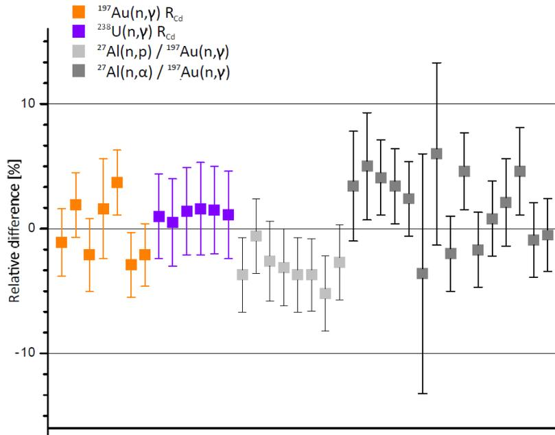
Fig. 8. JSI TRIGA Pneumatic Tube (PT) – relative differences between measured and calculated reaction rate ratios for nuclear reactions used to characterize the neutron spectrum.
