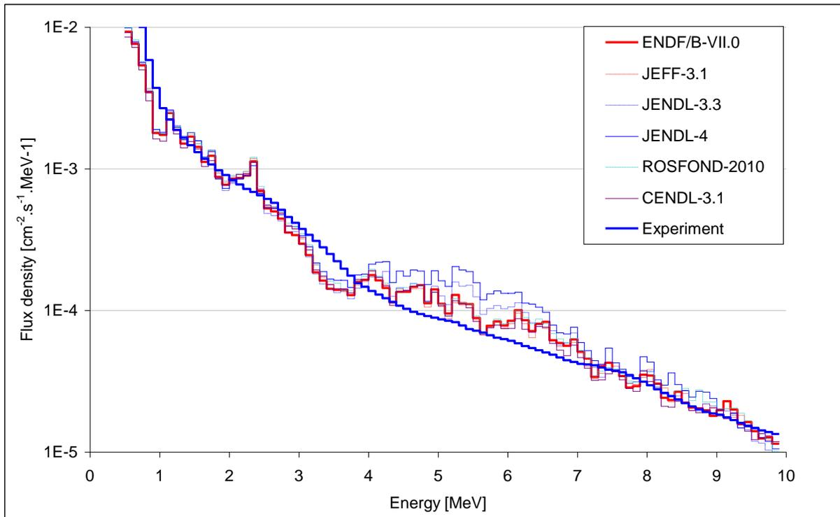
*Neutron flux density in biological shielding simulator (Point 8), (Kostal et al, Annals of Nuclear Energy, Vol. 94, (2016), pp 672-683)*
