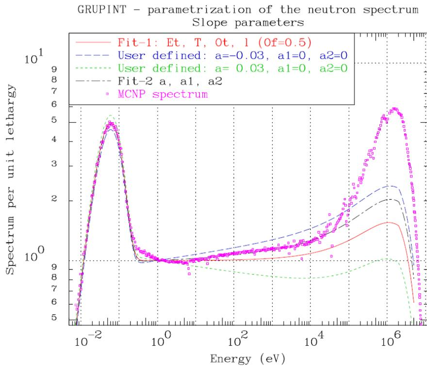
Fig. 2. Fitting the epithermal slope parameters to an input spectrum.
