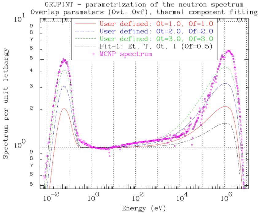
Fig. 1. Fitting the parameters of the thermal part to an input spectrum.
