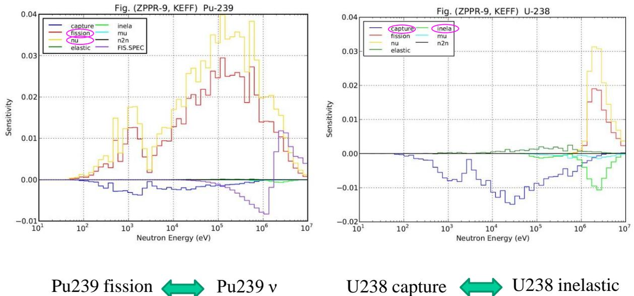
Fig. 3.1. Sensitivity coefficients for keff of a large fast reactor core ZPPR-9
