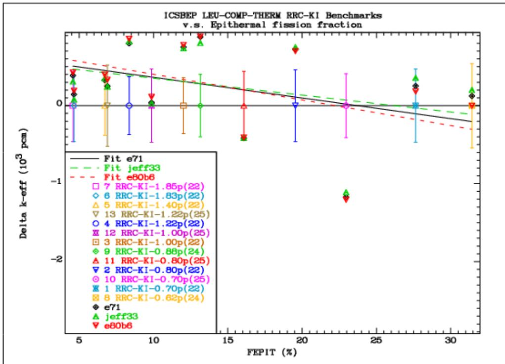
FIG. 6.1.6. Comparison of the differences between the calculated  $k_{\text{eff}}$  values and the reference benchmark values for the LEU-COMP-THERM-022, 24, 25 group of benchmarks as a function of the epithermal fission fraction.
