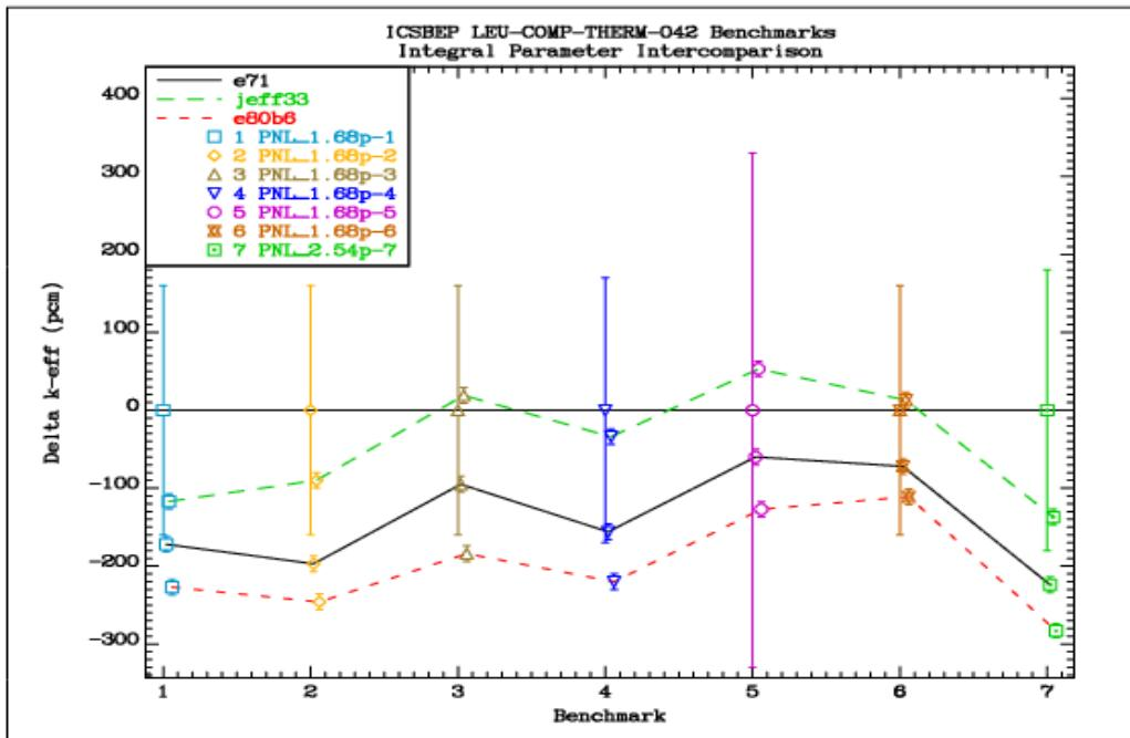
FIG. 6.1.7. Comparison of the differences between the calculated  $k_{\text{eff}}$  values and the reference benchmark values for the LEU-COMP-THERM-042 group of benchmarks.
