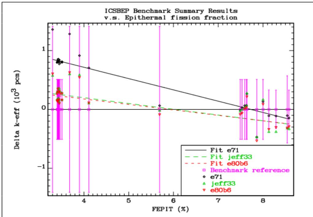
*FIG. 6.2.1. Comparison of the differences between the calculated  $k_{\text{eff}}$  values and the reference benchmark values as a function of EALF for the LEU-MET-THERM benchmarks with a heavy water moderator.*
