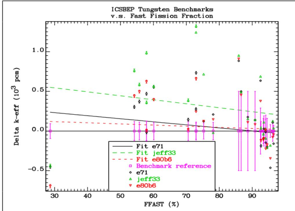
FIG. 7.3.1. Comparison of the differences between the calculated  $k_{\text{eff}}$  values and the reference benchmark values for all benchmarks containing tungsten. Benchmarks in which tungsten is the fuel dilutant have the softer spectrum.
