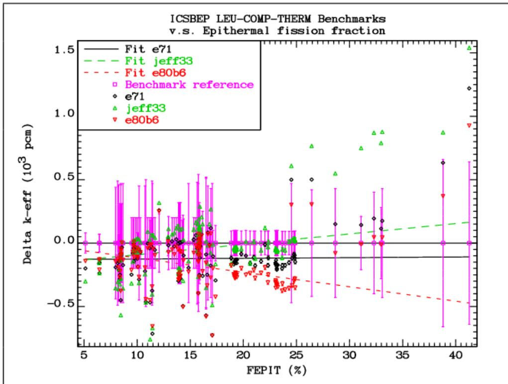
**FIG. 6.1.9.** Comparison of the differences between the calculated  $k_{\text{eff}}$  values and the reference benchmark values for the selected groups of benchmarks as a function of the epithermal fission fraction.
