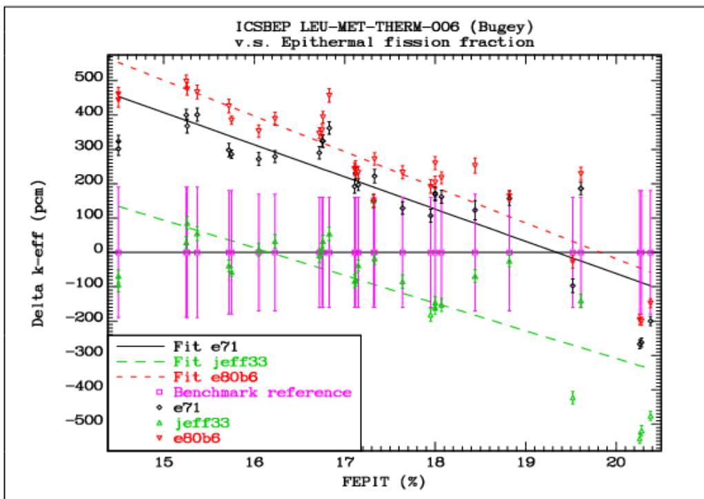
*FIG. 6.2.6. Comparison of the differences between the calculated  $k_{\text{eff}}$  values and the reference benchmark values as a function of the epithermal fission fraction for the LEU-MET-THERM-006 benchmarks with a light water moderator.*
