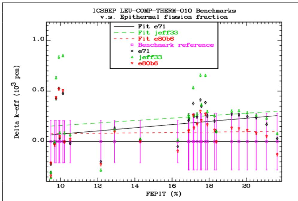
FIG. 6.1.5. Comparison of the differences between the calculated  $k_{\text{eff}}$  values and the reference benchmark values for the LEU-COMP-THERM-010 group of benchmarks as a function of the epithermal fission fraction.
