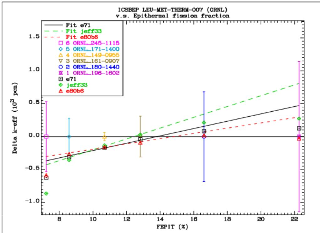
FIG. 6.2.4. Comparison of the differences between the calculated  $k_{\text{eff}}$  values and the reference benchmark values as a function of the epithermal fission fraction for the LEU-MET-THERM-007 benchmarks with a light water moderator.
