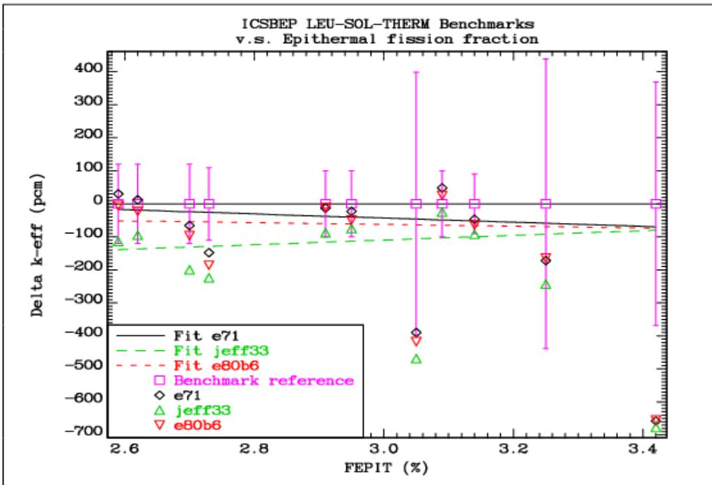
*FIG. 6.3.3. Comparison of the differences between the calculated  $k_{\text{eff}}$  values and the reference benchmark values as a function of the epithermal fission fraction for the LEU-SOL-THERM benchmarks, which do not exhibit a gradient in reactivity.*
