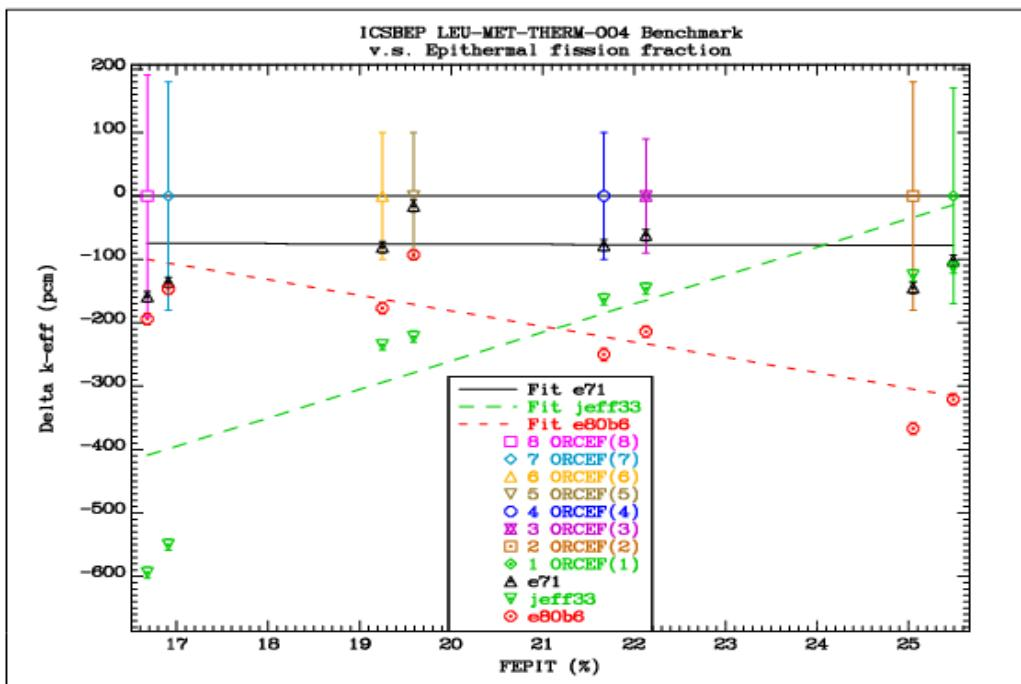
*FIG. 6.2.5. Comparison of the differences between the calculated  $k_{\text{eff}}$  values and the reference benchmark values as a function of the epithermal fission fraction for the LEU-MET-THERM-004 benchmarks with a light water moderator.*
