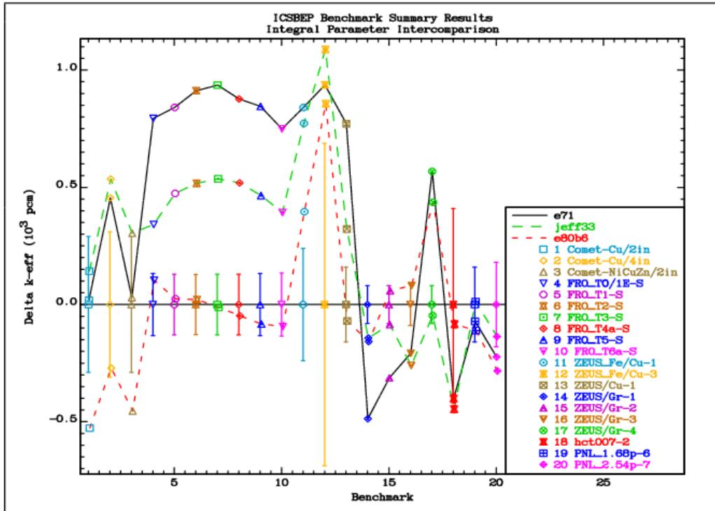
FIG. 7.2.1. Comparison of the differences between the calculated  $k_{\text{eff}}$  values and the reference benchmark values for the copper-reflected assemblies.
