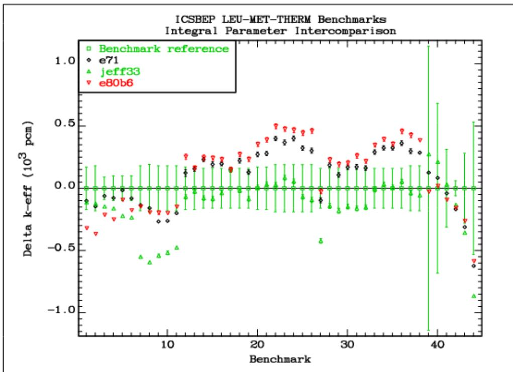
FIG. 6.2.3. Comparison of the differences between the calculated  $k_{\text{eff}}$  values and the reference benchmark values for the LEU-MET-THERM benchmarks with a light water moderator.
