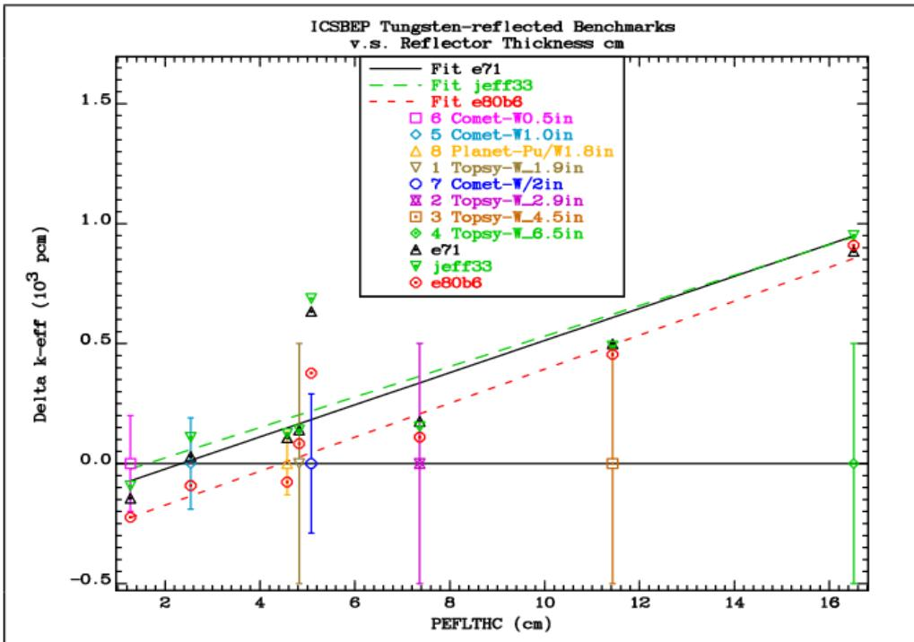
FIG. 7.3.2. Comparison of the differences between the calculated  $k_{\text{eff}}$  values and the reference benchmark values for the benchmarks with a tungsten reflector as a function of reflector thickness.
