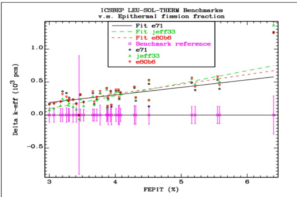
*FIG. 6.3.2. Comparison of the differences between the calculated  $k_{\text{eff}}$  values and the reference benchmark values as a function of the epithermal fission fraction for the LEU-SOL-THERM benchmarks, which exhibit a gradient in reactivity.*
