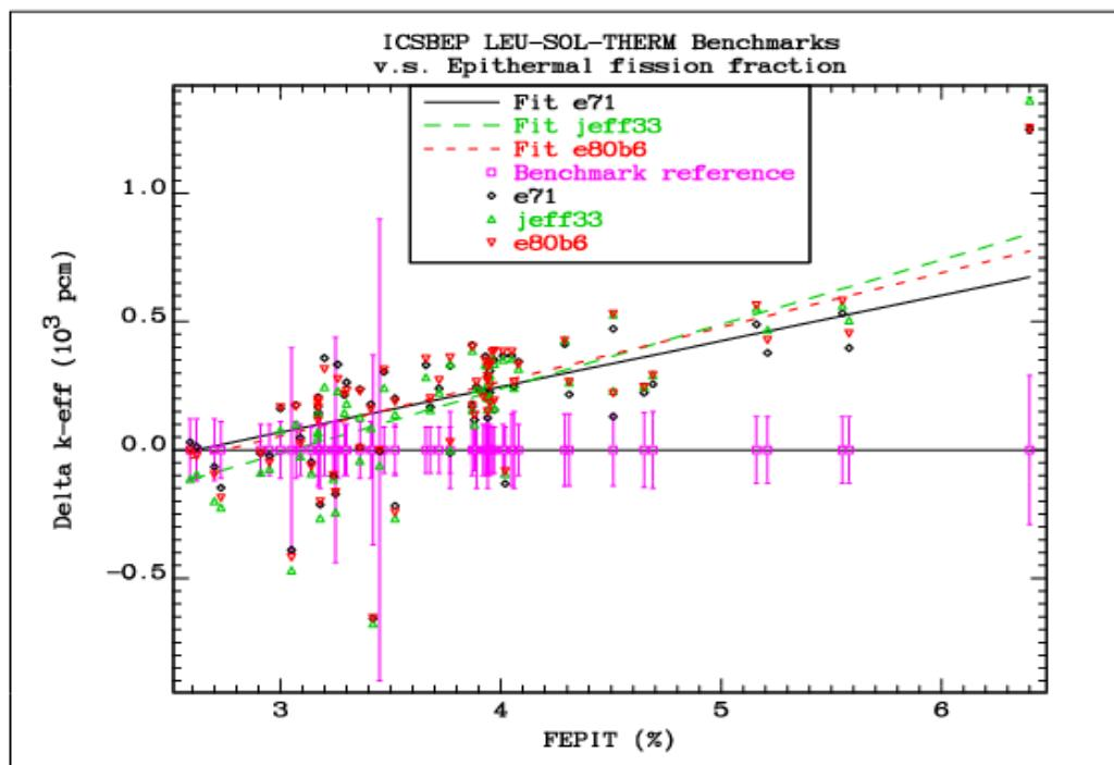
FIG. 6.3.1. Comparison of the differences between the calculated  $k_{\text{eff}}$  values and the reference benchmark values as a function of the epithermal fission fraction for the LEU-SOL-THERM benchmarks.
