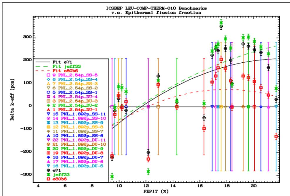
FIG. 6.1.5a. Comparison of the differences between the calculated  $k_{\text{eff}}$  values and the reference benchmark values for the LEU-COMP-THERM-010 group of benchmarks (excluding the lead-reflected cases) as a function of the epithermal fission fraction. The trendlines are parabolic fits.
