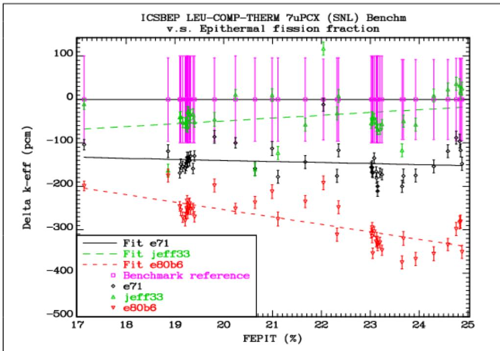
*FIG. 6.1.8. Comparison of the differences between the calculated  $k_{\text{eff}}$  values and the reference benchmark values for the LEU-COMP-THERM-078, 80 and 96 group of benchmarks as a function of the epithermal fission fraction.*
