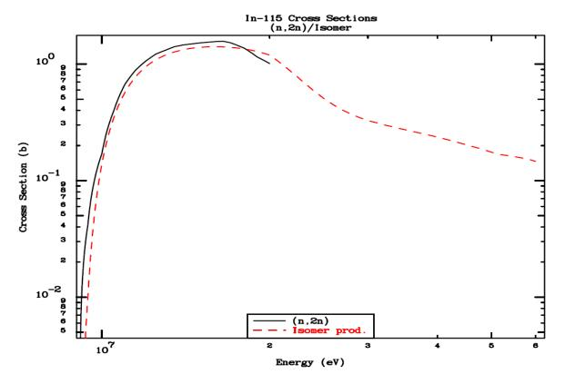
The capture cross sections are not changes and the isomer production cross sections In-116m are not included from IRDFF-II. Isomer production cross sections In-114m and In-115m depend not only on the inelastic and (n,2n) cross sections, respectively, but also on the whole cascade of levels, so the isomer production cross sections from inelastic scattering and (n,2n) are included from IRDFF-II.
