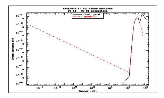
The (n,2n) cross section from IRDFF-II was inserted into the original ENDF file up to 45 MeV to avoid a discontinuity. The maximum difference in the elastic cross section is less than 4 %. No change is needed for the (n,p) cross sections. The question about the sub-threshold (n, $\alpha$ ) cross sections needs a more detailed investigation, so no changes were made.
