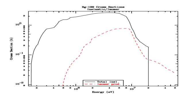
Isomer production cross sections Hg-199m depend not only on the inelastic cross sections but also on the whole cascade of levels, so the isomer production cross sections from inelastic scattering are not in contradiction with the inelastic cross sections in MF 3, and so the data from IRDFF-II are included in the new ENDF file.
