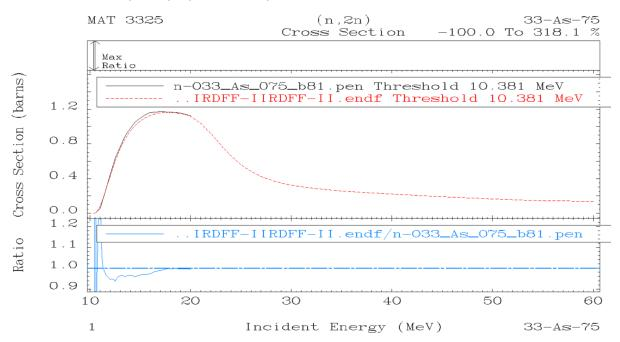
The MT 16 cross sections from IRDFF-II were inserted into the original ENDF file. The impact on the elastic cross sections is negligible.
