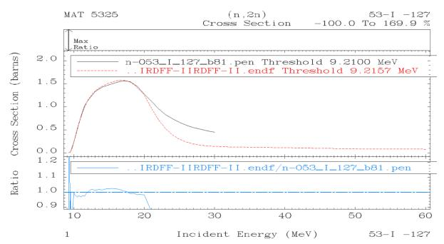
The MT 16 cross sections from IRDFF-II were inserted into the original ENDF file up to 30 MeV. The IRDFF-II cross sections drop rapidly above 20 MeV, giving rise to significant increase in the elastic cross section. It might be worth considering using the IRDFF-II cross sections only up to 20 MeV.
