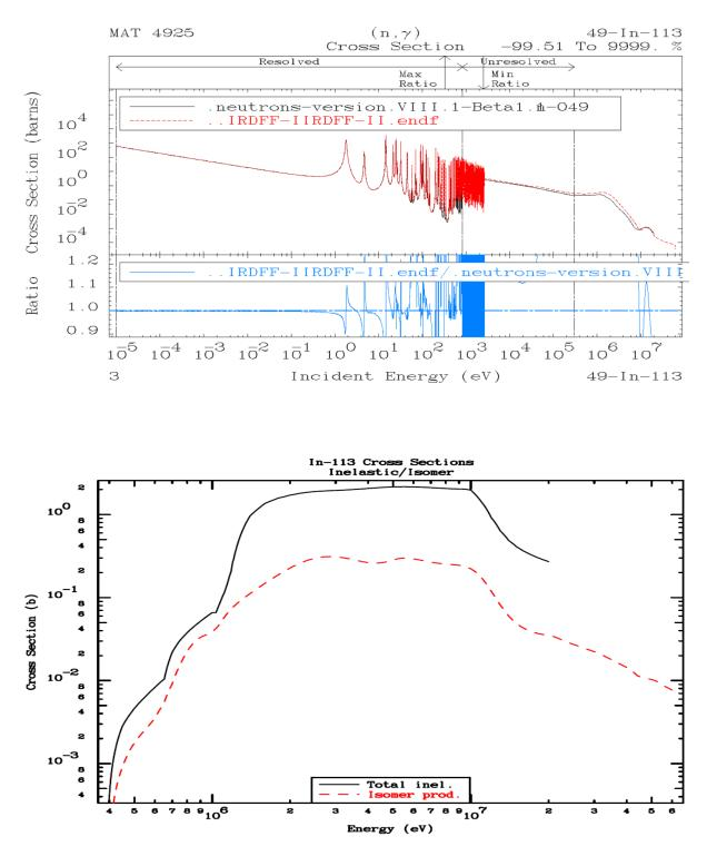
The capture cross sections are not changes and the isomer production cross sections In-114m are not included from IRDFF-II. Isomer production cross sections In-113m depend not only on the inelastic cross sections but also on the whole cascade of levels, so the isomer production cross sections from inelastic scattering are included from IRDFF-II.
