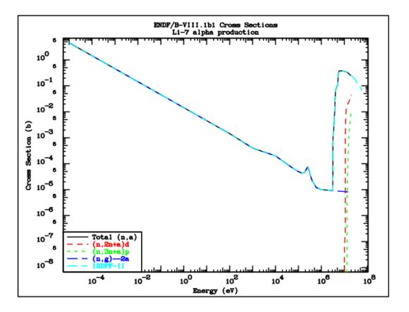
MT 207 in IRDFF-II is exactly equivalent to the sum of MT 24, 25 plus twice MT 102, since two alphas are emitted when <sup>8</sup>Li\* decays with a half life of 840 ms into <sup>8</sup>Be\*, which in turn breaks up almost instantly into two alphas. The two libraries are consistent.
