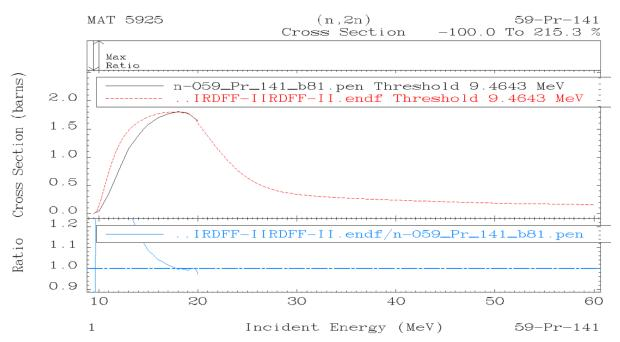
Insertion of the MT 16 cross sections from IRDFF-II library into the original ENDF file makes a significant impact on the elastic cross sections. Suitability of the modification might need some further consideration.
