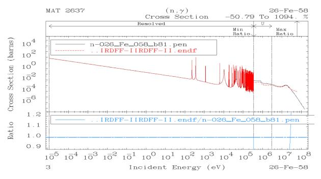
There are differences above the resonance range, which require further investigation, so no changes to the cross sections were made.
