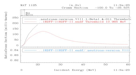
The (n,2n) cross section in the file was replaced with the data from IRDFF-II up to 20 MeV.
