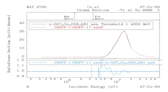
Cross sections for the (n,2n), (n,3n), (n,p), (n,a) were replaced with IRDFF-II. The change in the elastic cross section approaches 5 % near the upper end of the evaluation at 20 MeV.
