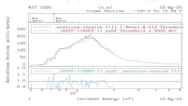
The (n,p) cross section in the file was replaced with the data from IRDFF-II up to 20 MeV. The fluctuations in the elastic cross sections are amplified, but not dramatically so.
