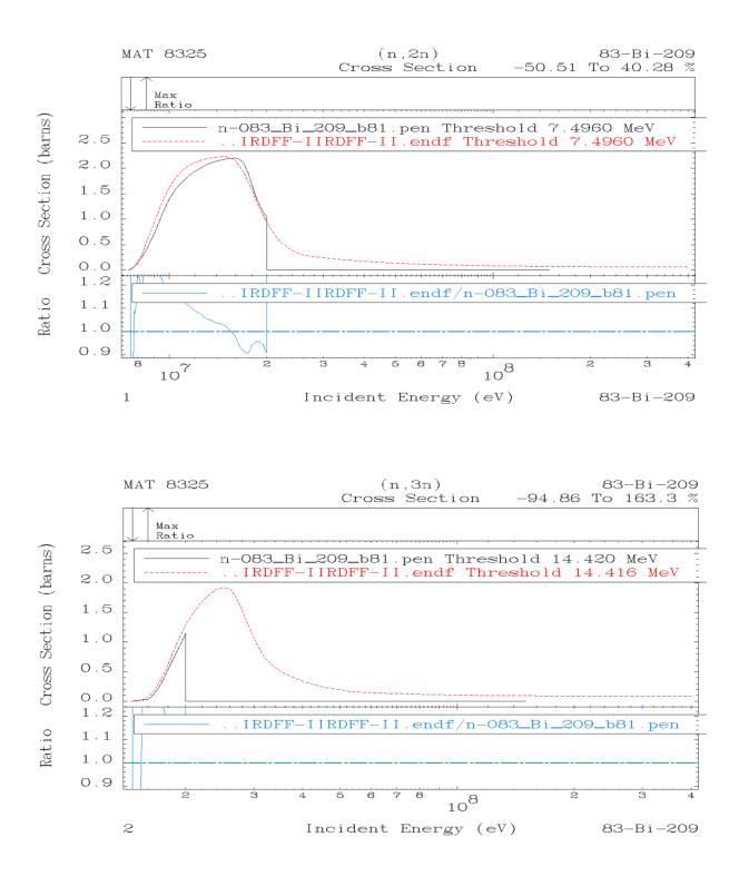
The elastic cross sections are affected by up to 10 %. The (n,2n) and (n,3n) cross sections from IRDFF-II were inserted into the original ENDF file up to 20 MeV because at higher energies the dual representation in MT 5 is used and the implied cross sections cannot be updated consistently.
