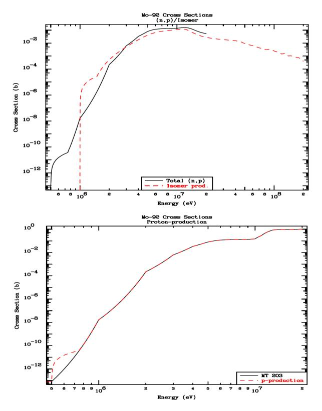
The proton-emission cross section MT 103 (including discrete levels) is related to the isomer production, but the latter depends on the summation of higher levels feeding the long-lived isomeric level, so the inclusion of the isomer production from IRDFF-II is valid.
