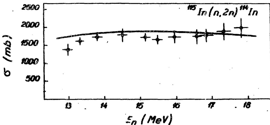
Fig.4 The cross sections for the  $^{115}\text{In}(n, 2n)^{114}\text{In}$  reaction.
