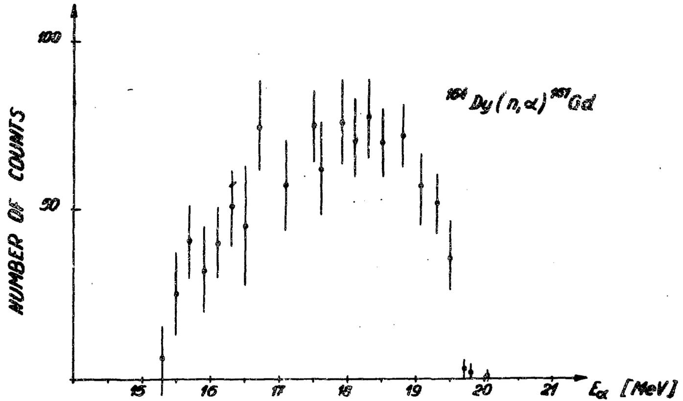
Fig. 2 The experimental  $\alpha$ -particle spectrum from the  $^{164}\text{Dy}(n, \alpha)^{161}\text{Gd}$  reaction.
