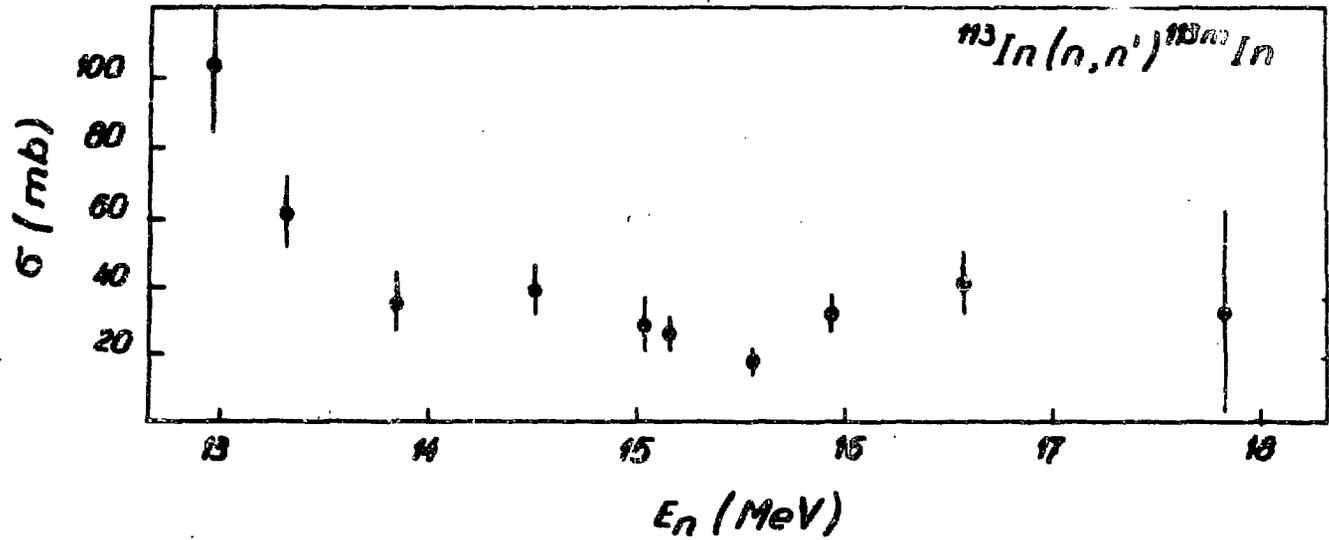
Fig. 1. Cross sections for the  $^{113}\text{In}(n,n')^{113\text{m}}\text{In}$  reaction.
