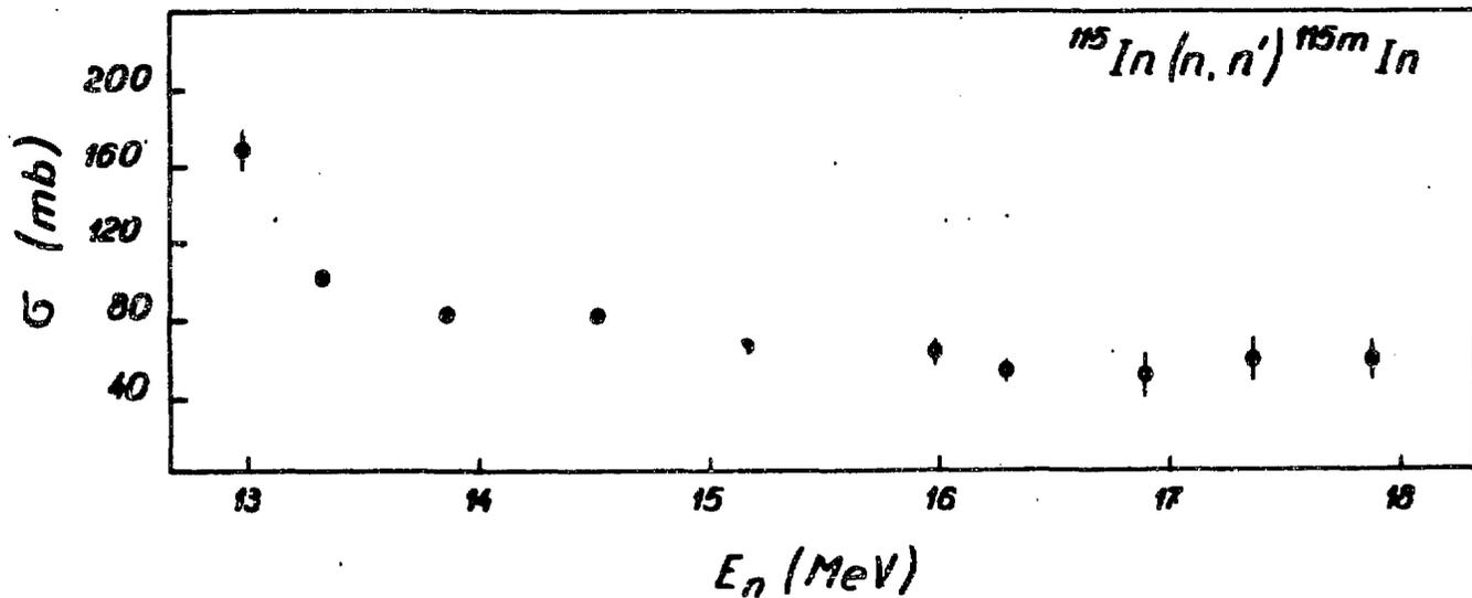
Fig.2. Cross sections for the  $^{115}\text{In}/n, n' / ^{115m}\text{In}$  reaction.
