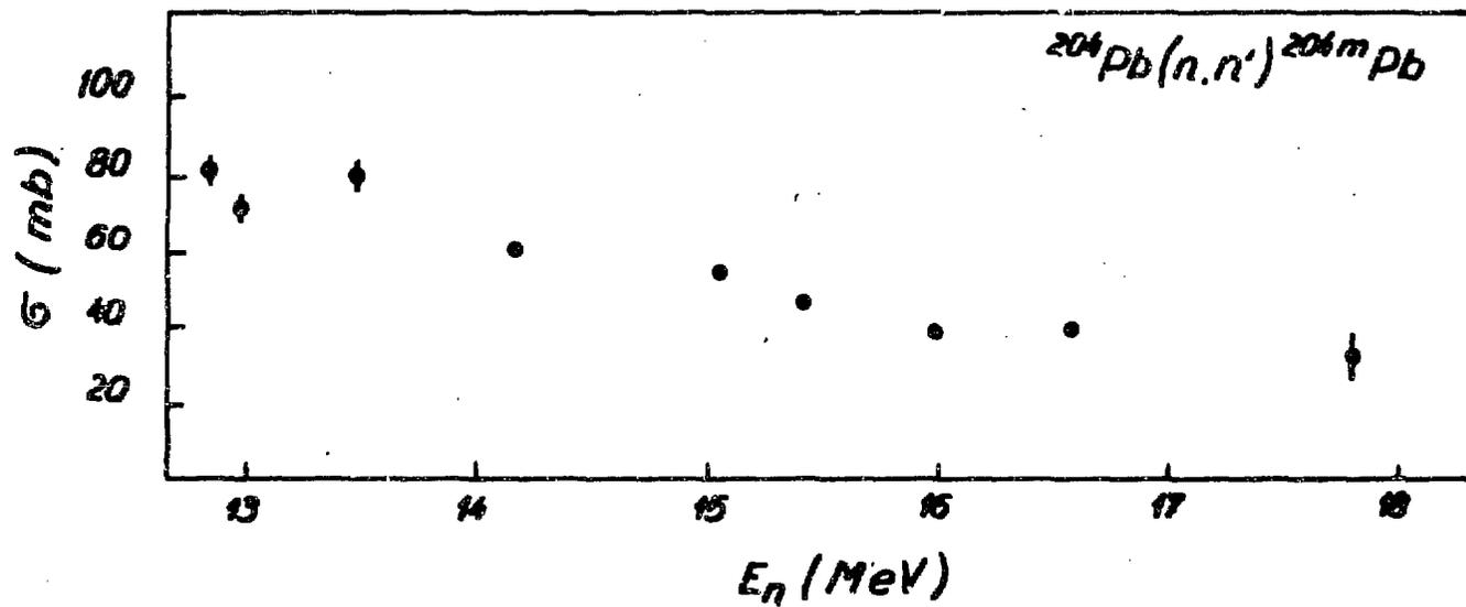
Fig.3. Cross sections for the  $^{204}\text{Pb}/n,n'/^{204m}\text{Pb}$  reaction.
