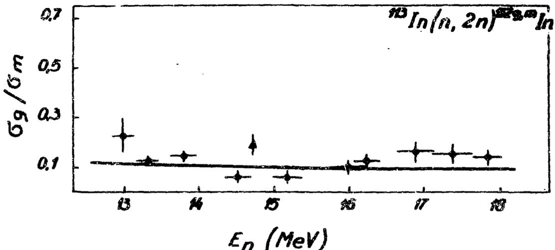
Fig.1 The isomeric ratios for the  $^{113}\text{In}(n, 2n)^{112g,m}\text{In}$  reaction. ● - our results; ▲ - result of ref. /7/. The solid line presents the statistical calculations based on the superconductivity model of the level density.
