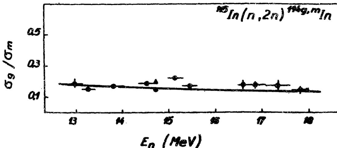
Fig.2 The isomeric ratios for the  $^{115}\text{In}(n, 2n)^{114g,m}\text{In}$  reaction. ● -our results; ▲ -result of ref./7/; ○ - result of ref. /6/. The solid line presents the statistical calculations.
