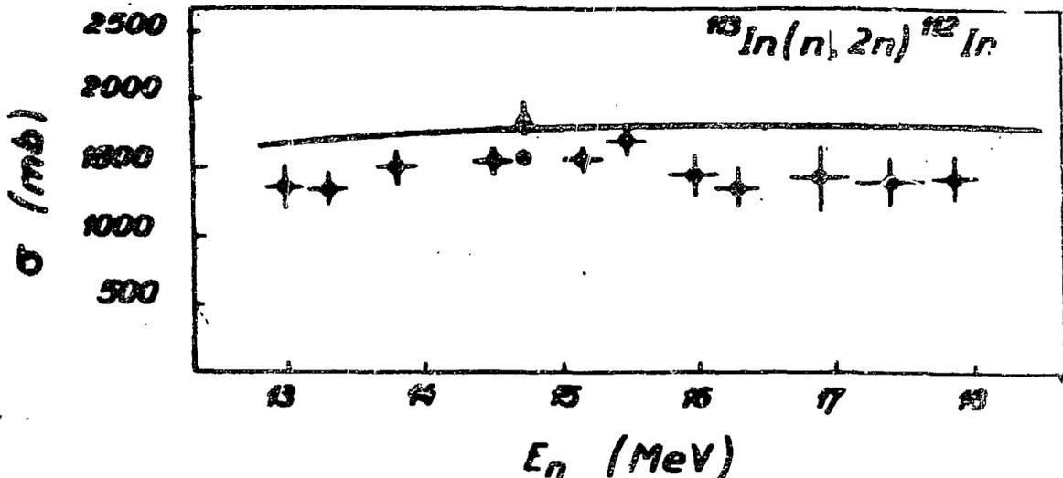
Fig.3 The cross sections for the  $^{113}\text{In}(n, 2n)^{112}\text{In}$  reaction.
