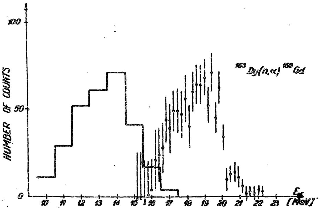
Fig. 1 The experimental  $\alpha$ -particle spectra from the  $^{161}\text{Dy}/n,\alpha/^{158}\text{Gd}$  and  $^{163}\text{Dy}/n,\alpha/^{160}\text{Gd}$  reactions, and the predictions of the statistical theory.
