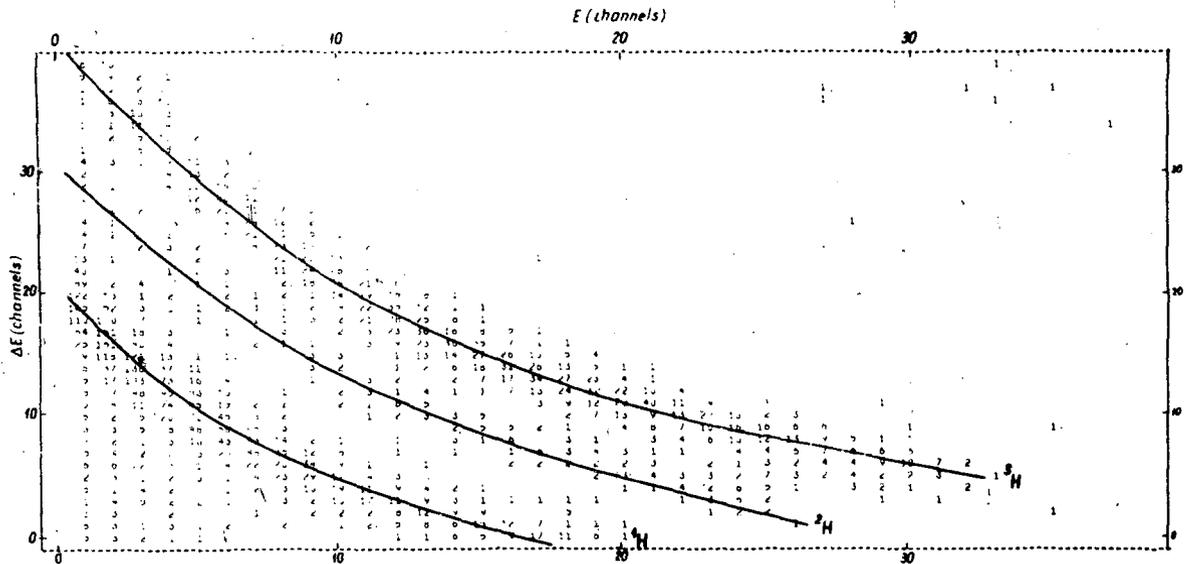
Fig. 2 The two-parameter spectrum for particles with  $Z = 1$
