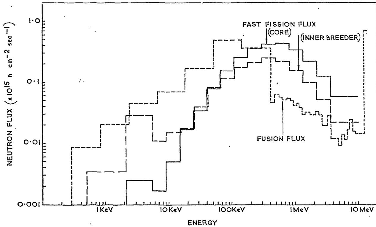
Fig.3 Neutron Flux Values in various Energy Groups in (a) Dounreay Fast Reactor Core; (b) D.F.R. Inner Breeder; (c) Fusion Reactor Model First Wall.
