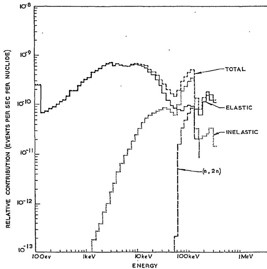
Fig.17 A Histogram of the Three Contributing Damage Energy Spectra, and their sum, in the Neutron Flux in the First Wall of a Model Fusion Reactor.
