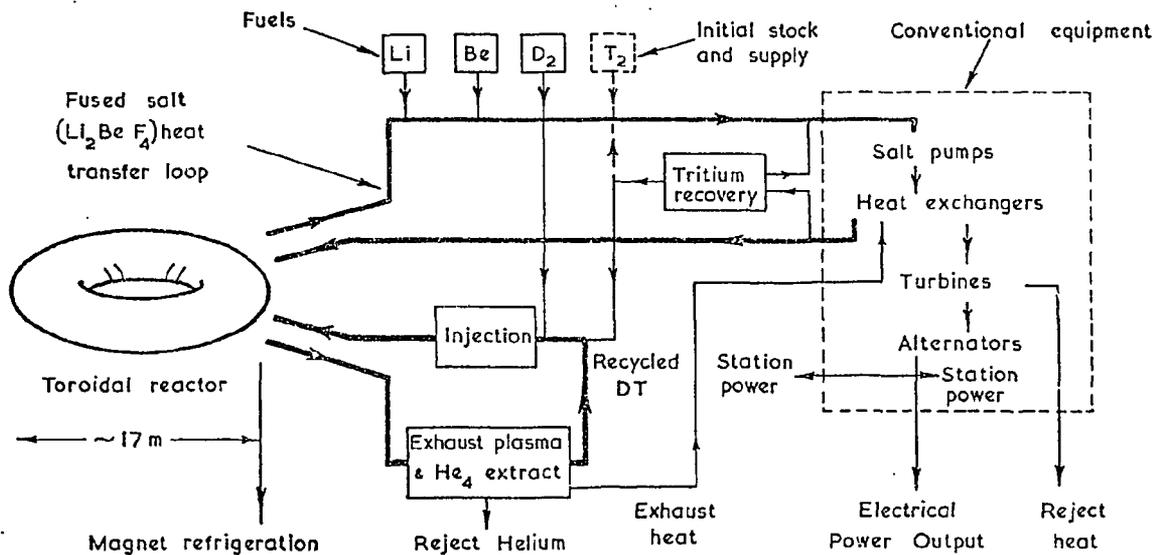
Fig.2 Functional diagram of D-T fusion reactor generating station.
