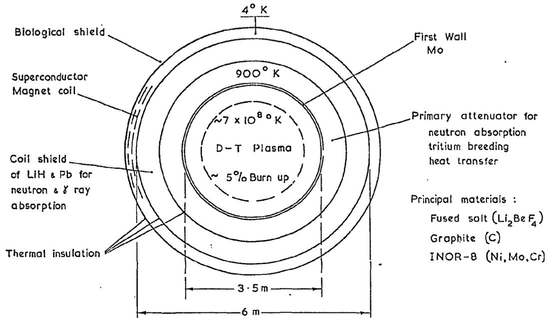
Fig.1 Conceptual design cross-section of D-T Reactor - blanket after Homeyer (1965).
