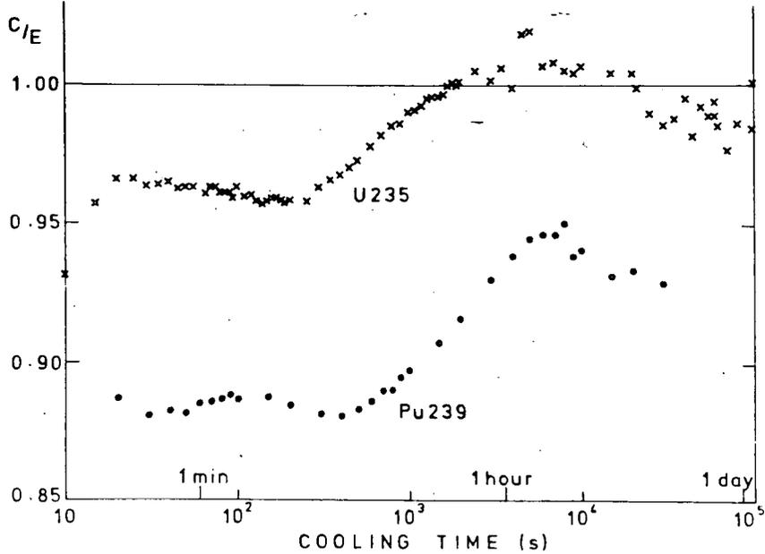
Fig. 2. Comparison of UKFPDD-1/C31 calculations of the total decay heat for <sup>235</sup>U (x) and <sup>239</sup>Pu (●) after 2 x 10<sup>4</sup>s irradiation with LASL measurements.
