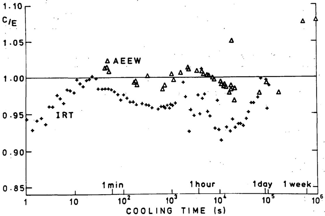
Fig. 5. Comparison of UKFPDD-1/C3I calculations of the beta heating for  $^{235}\text{U}$  with IRT measurements (+) after  $8.64 \times 10^4$ s irradiation and also with AEEW measurements ( $\Delta$ ) after  $10^5$ s.
