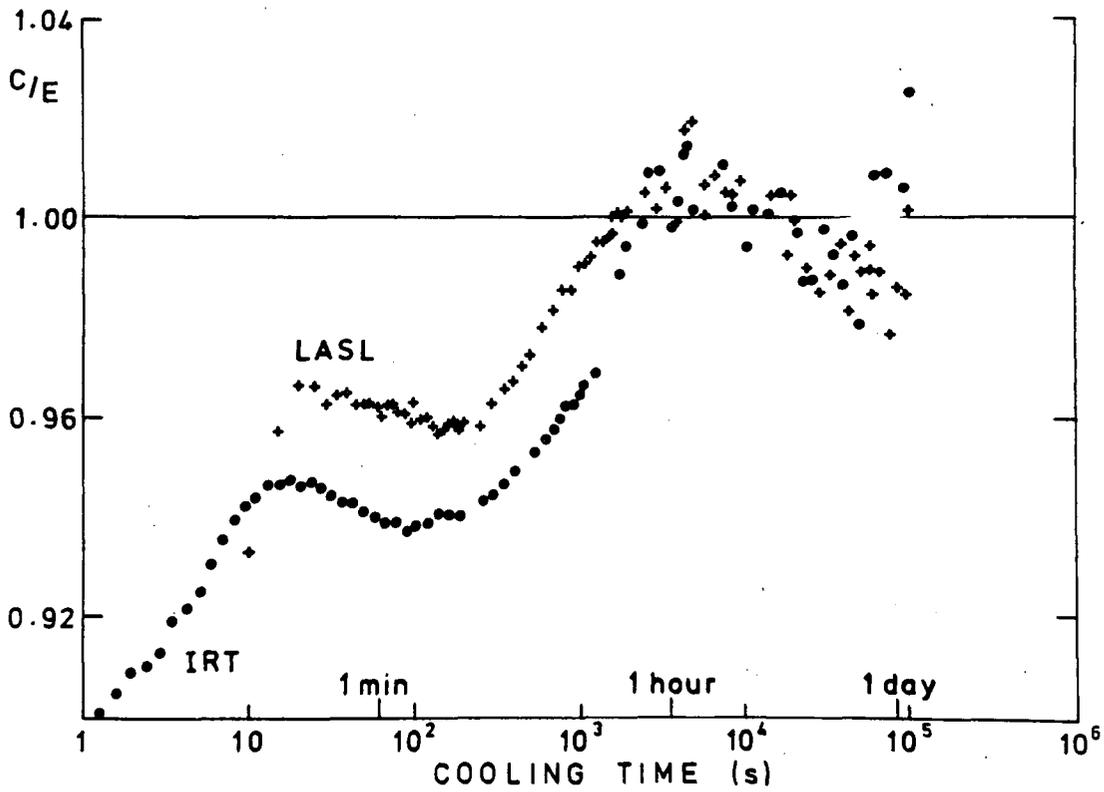
Fig. 3. Comparison of UKFPDD-1/C3I calculations of the total decay heat for  $^{235}\text{U}$  after  $2 \times 10^4$  s irradiation with the LASL measurements (+) and the IRT measurements (●).
