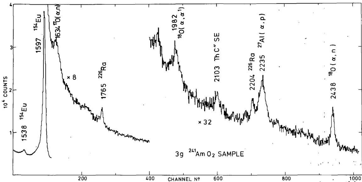
Fig. 1.7 The gamma-ray spectrum from the 3 g  $^{241}\text{AmO}_2$  sample between 1.5 and 2.5 MeV. The  $^{154}\text{Eu}$  impurity will not contribute to the  $(\alpha, n)$  yield.
