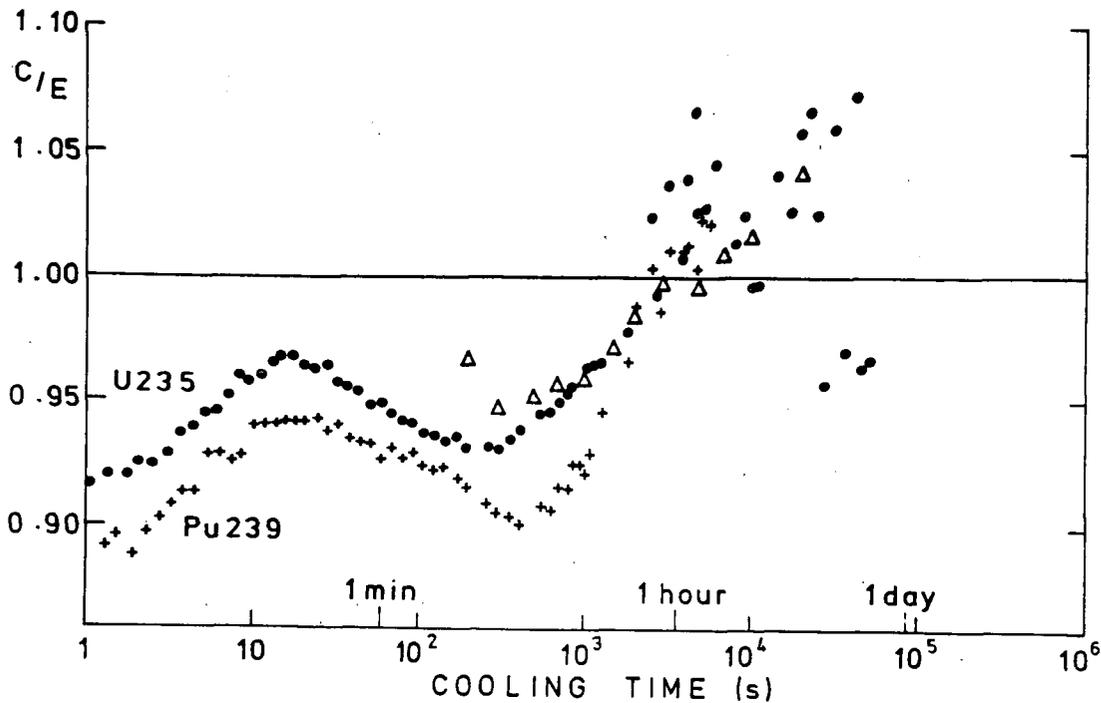
Fig. 4. Comparison of UKFPDD-1/C3I calculations of the total decay heat after  $10^3$  s irradiation with IRT measurements on  $^{239}\text{Pu}$  (+) and for  $^{235}\text{U}$  (●) also shown for  $^{235}\text{U}$  ( $\Delta$ ) are the measurements of ref. (21).
