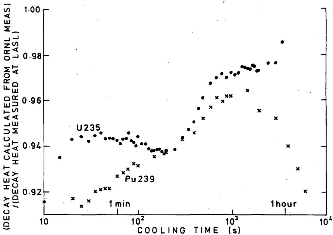
Fig. 7. Comparison of the total decay heat computed from short irradiation measurements at ORNL and compared to measurements at LASL after  $2 \times 10^4$ s irradiation for  $^{235}\text{U}$  (●) and  $^{239}\text{Pu}$  (x).
