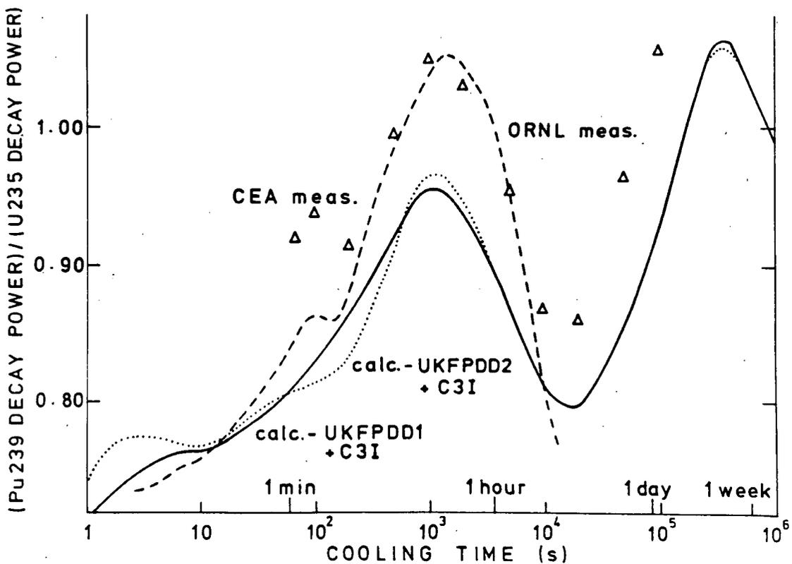
Fig. 10. Ratio of total decay powers after 1 fission for  $^{239}\text{Pu}/^{235}\text{U}$ ; data are (Δ) CEA, (- - -) ORNL, (—) calculated using UKFPDD-1/C3I and (.....) calculated using UKFPDD-2/C3I.
