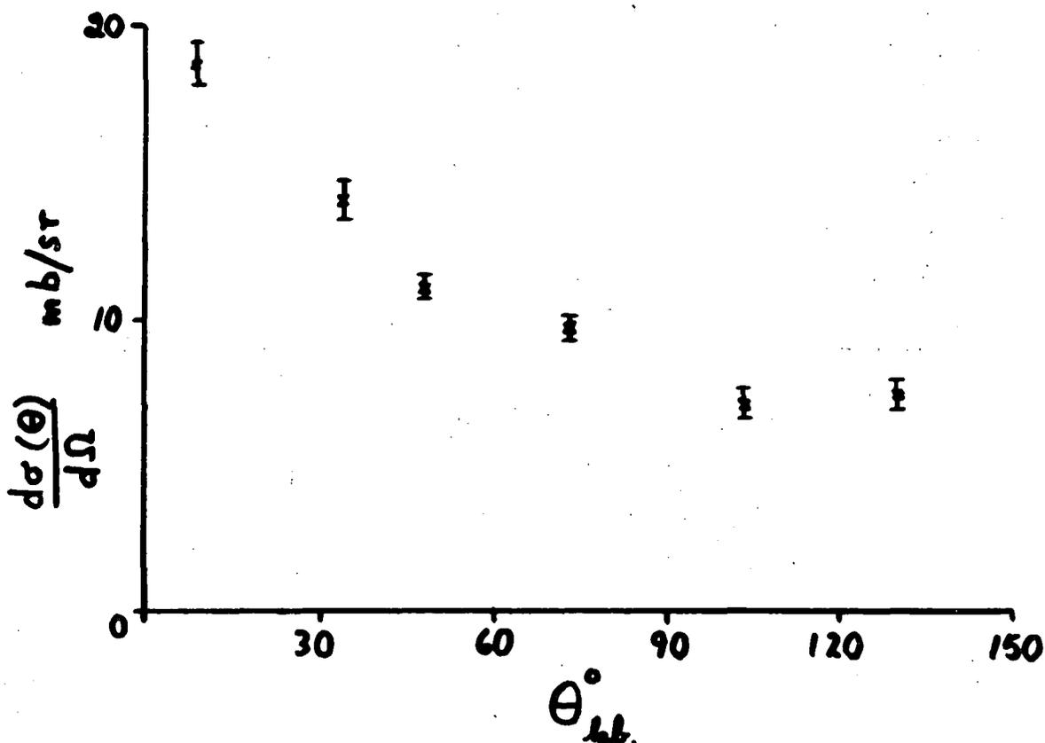
Fig. 1.5 Preliminary cross section values for the  $^{27}\text{Al}(n,\alpha)$  reactions at a neutron energy of 14.5 MeV. Errors shown are purely statistical.
