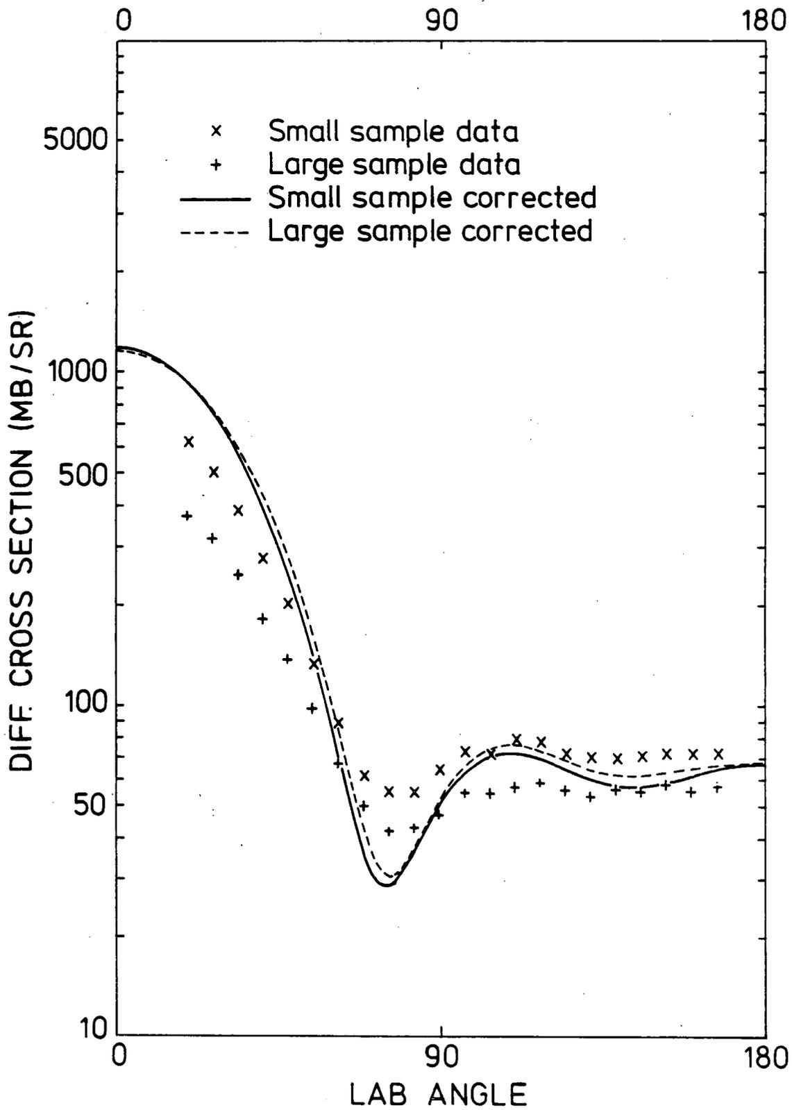
Fig. 7.2 Differential elastic cross section for 3 MeV neutrons incident upon iron.
