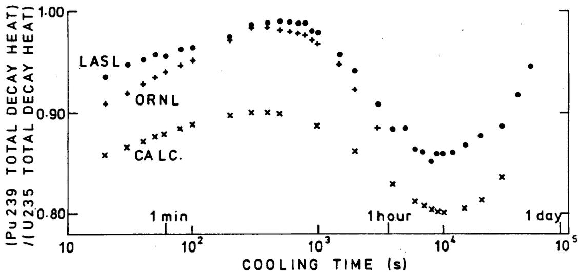
Fig. 9. Ratio of total decay heat for  $^{239}\text{Pu}/^{235}\text{U}$  after  $2 \times 10^4\text{s}$  irradiation; data are (●) lasl measurement, (+) derived from ORNL and (x) calculated using UKFPDD-1/C3I.
