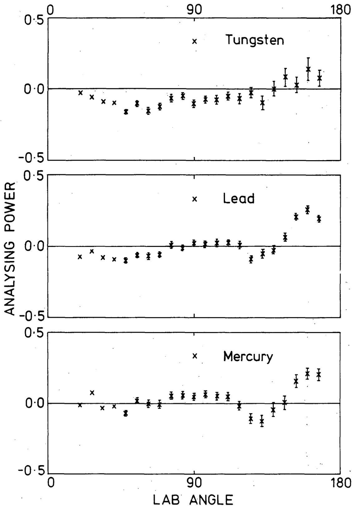
Fig. 7.1 Analysing power for 3 MeV neutrons as measured by the new polarimeter
