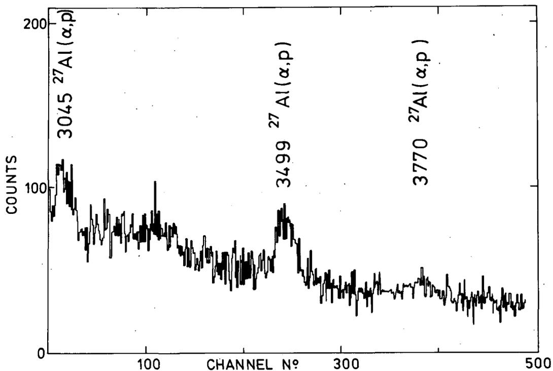
Fig. 1.8 The gamma-ray spectrum from the 3 g  $^{241}\text{AmO}_2$  sample between 3 and 4 MeV.
