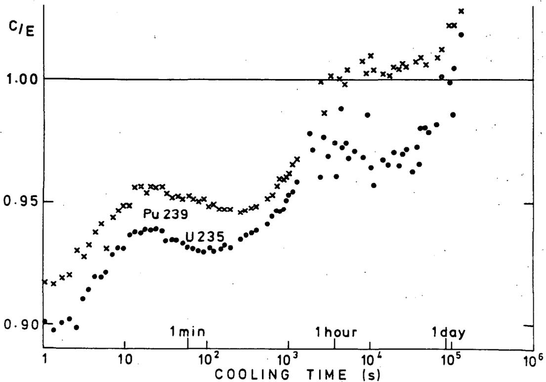
Fig. 6. Comparison of UKFPDD-1/C3I calculations of the total decay heat after 24 hours irradiation with IRT measurements on  $^{235}\text{U}$  (●) and  $^{239}\text{Pu}$  (x).
