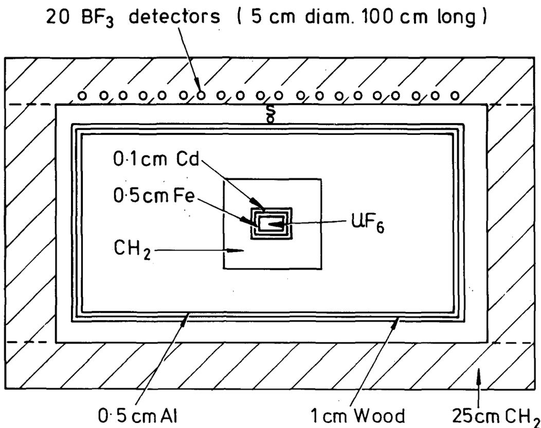
Fig. 1.6 Geometrical arrangement of  $UF_6$  sample, neutron shielding, package and package monitor used in MONK calculations
