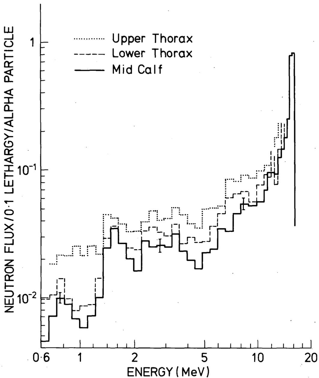
Fig. 8.1 Measured neutron spectrum in a water-filled anthropomorphic phantom, at lower and upper positions in the mid thorax, and at the centre of the lower leg.
