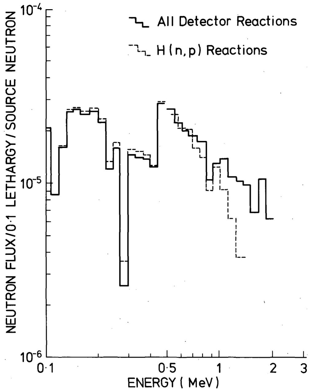
Fig. 8.4 Comparison of the neutron spectrum in LiF unfolded with and without allowing for charged particle production in the walls and in argon (detector as in Fig. 8.2)
