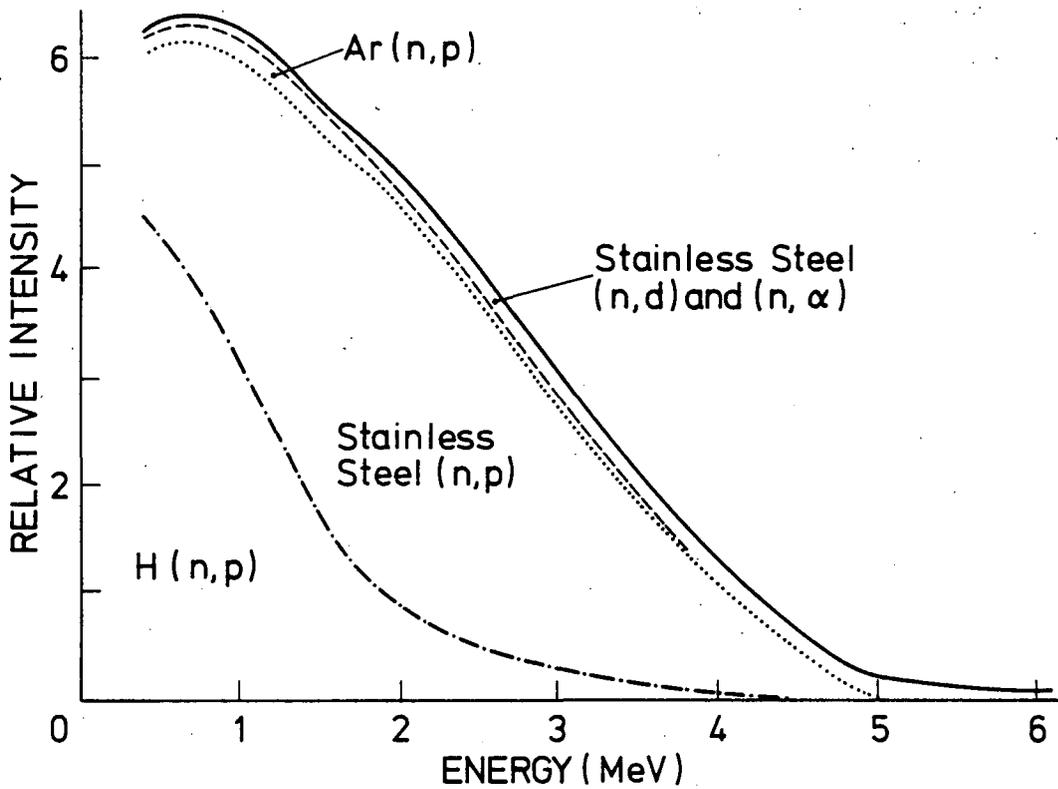
Fig. 8.2 Components of the response of a 4 cm diameter spherical proportional counter (2 atmos.  $H_2$  and 8 atmos. Ar) exposed to 14.2 MeV neutrons.
