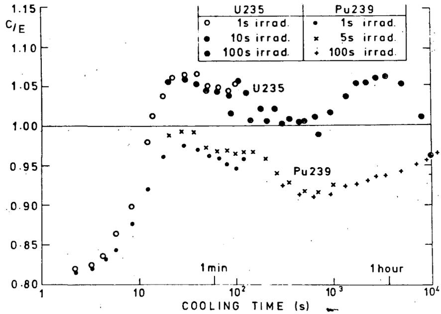
Fig. 1. Comparison of UKFPDD-1/C2 calculations of the total decay heat with the ORNL measurements.
