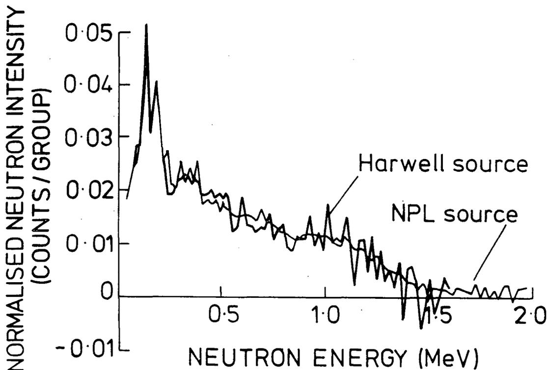
Fig. 6.1 The neutron spectrum from the Harwell and NPL Am/Li sources
