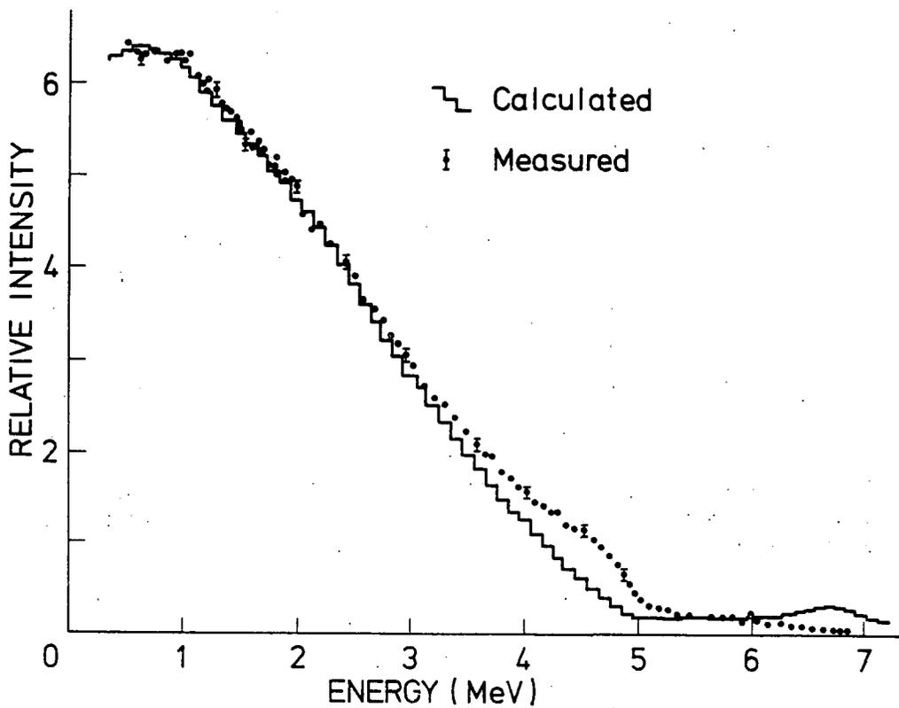
Fig. 8.3 Comparison of experimental and predicted detector response functions for 14.2 MeV neutrons (detector as in Fig. 8.2)
