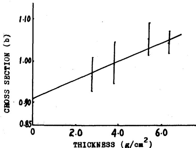
Fig. 1. Apparent nonelastic cross section of Si as a function of absorber thickness
