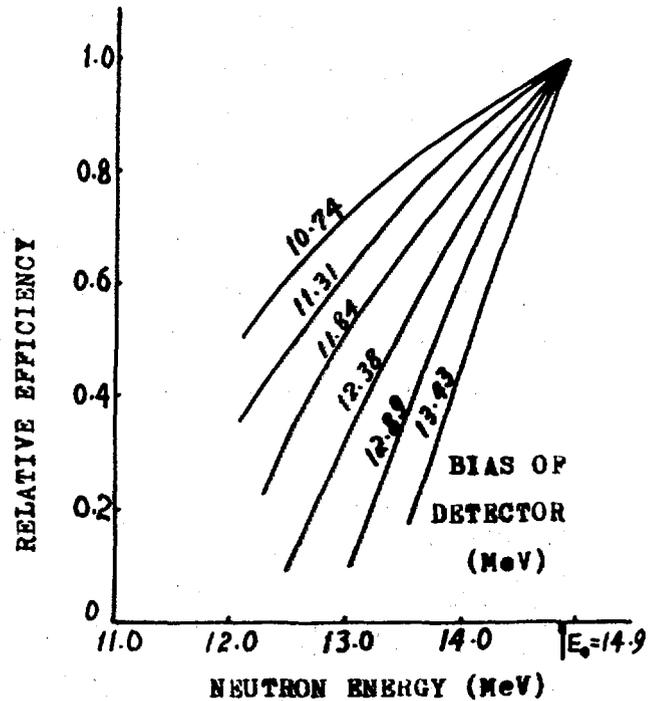
Fig. 2. Relative efficiency curve of a spherical plastic scintillator as a function of neutron energy for different biases
