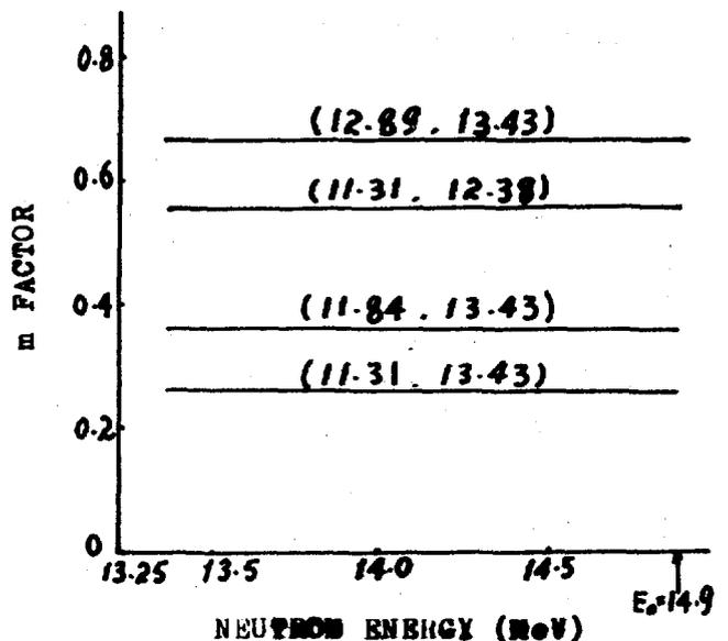
Fig. 3. Variation of the scale factor  $m$  with energy (by calculation)
