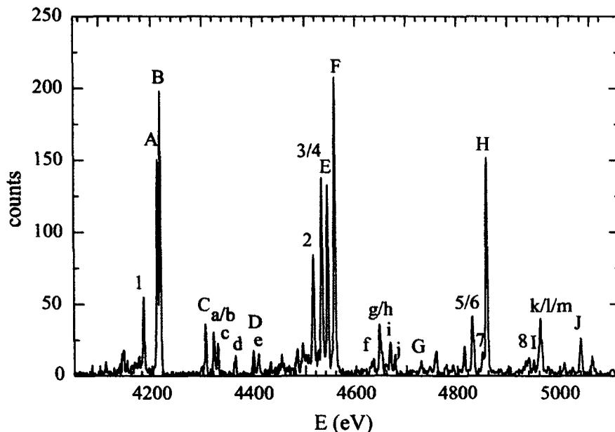
**Fig. 1** Crystal diffraction spectrum of L x-ray transitions in Xe<sup>43+...45+</sup>
