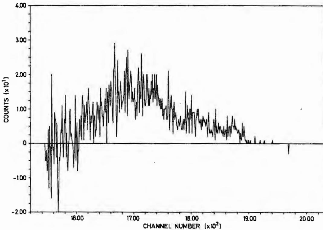
Fig.1.3 Experimental pulse height spectrum of scintillation detector observing charged particles from nickel foil.
