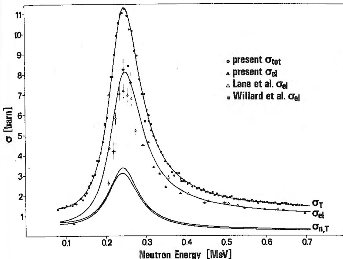
Fig. 3.1 The neutron total integrated elastic and (n,T) cross sections of  ${}^6\text{Li}$  are plotted versus the incident neutron energy. Curves are obtained from the fit.
