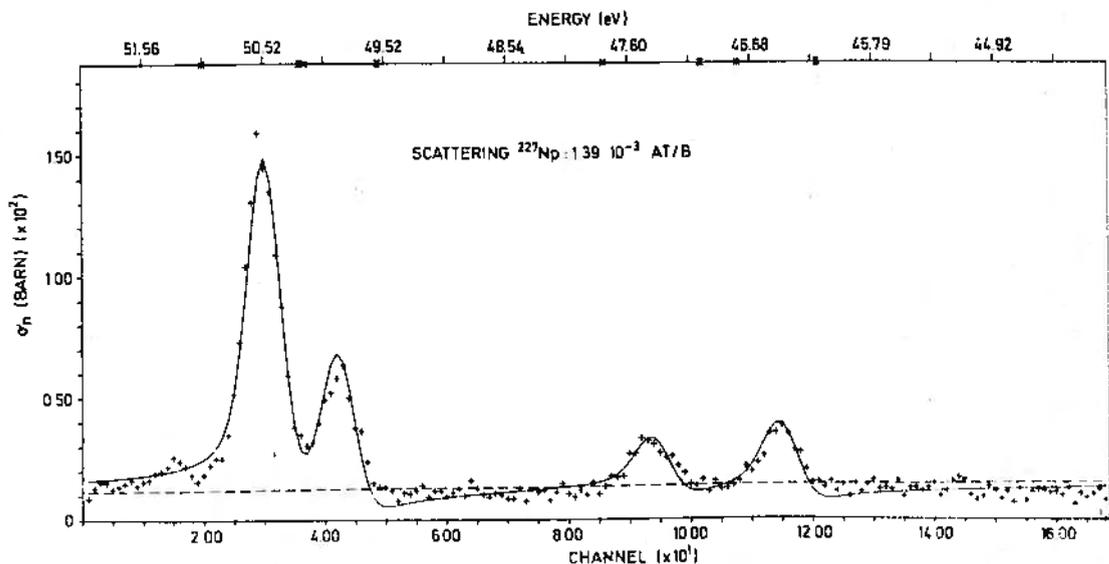
Fig 2.12 Scattering cross section of  $^{237}\text{Np}$  between 44.5 eV and 51.6 eV neutron energy. The full curve represents the cross section calculated from the adapted resonance parameters
