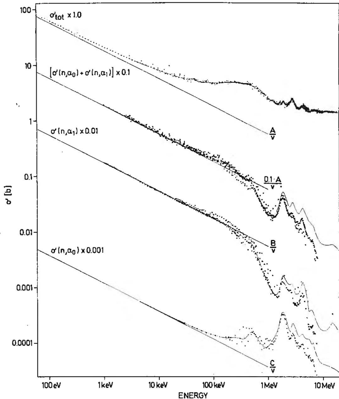
Fig. 3.3 Cross-sections:  $\sigma_{tot}$ ,  $\sigma(n, \alpha_0) + \sigma(n, \alpha_1)$ ,  $\sigma(n, \alpha_1)$  and  $\sigma(n, \alpha_0)$ . Continuous curves are ENDF/B IV 1975 evaluation.
