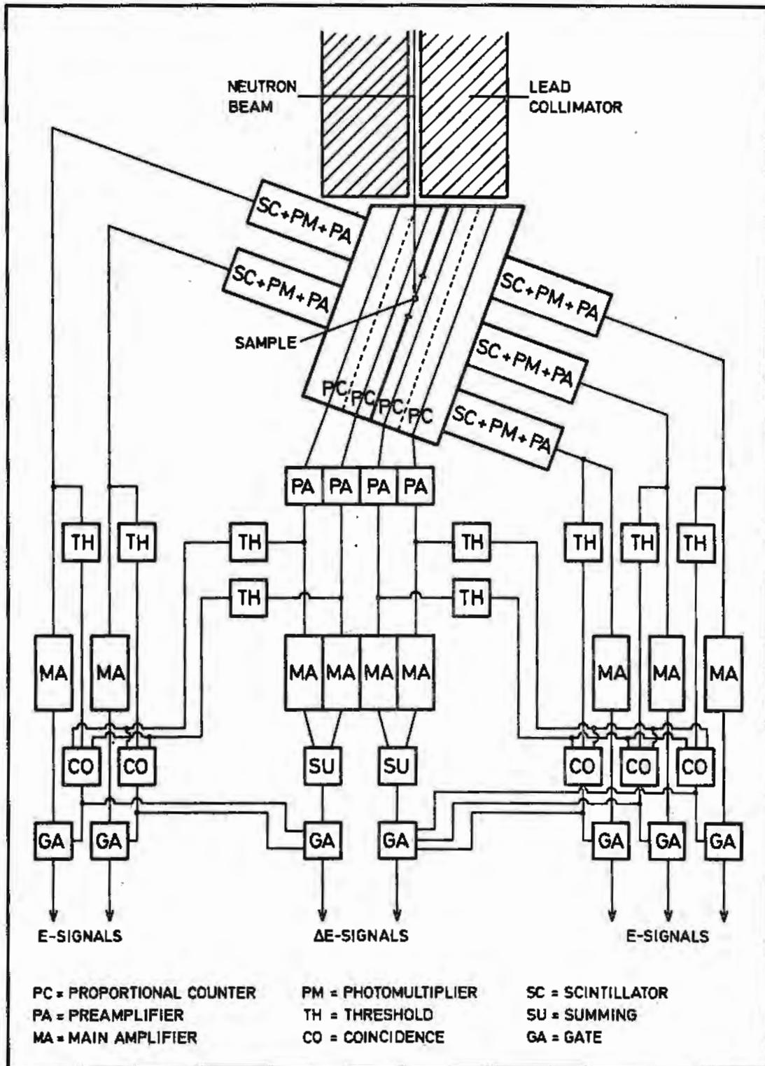
Fig.1.1 Experimental set-up for reaction chamber.
