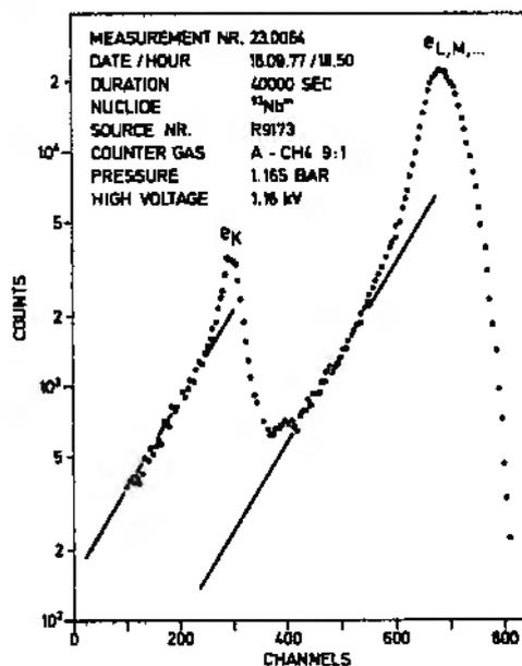
Fig.4.3 The conversion electron spectrum of  $^{93}\text{Nb}^m$  plotted in semi-log scale to correct for degradation in the low-energy tail
