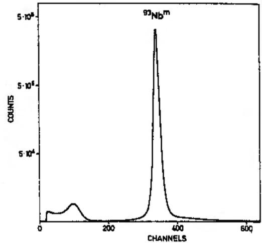
Fig. 4.1 Measurement of the disintegration rate of a  $^{93}\text{Nb}^m$  solution with the liquid scintillation technique.
