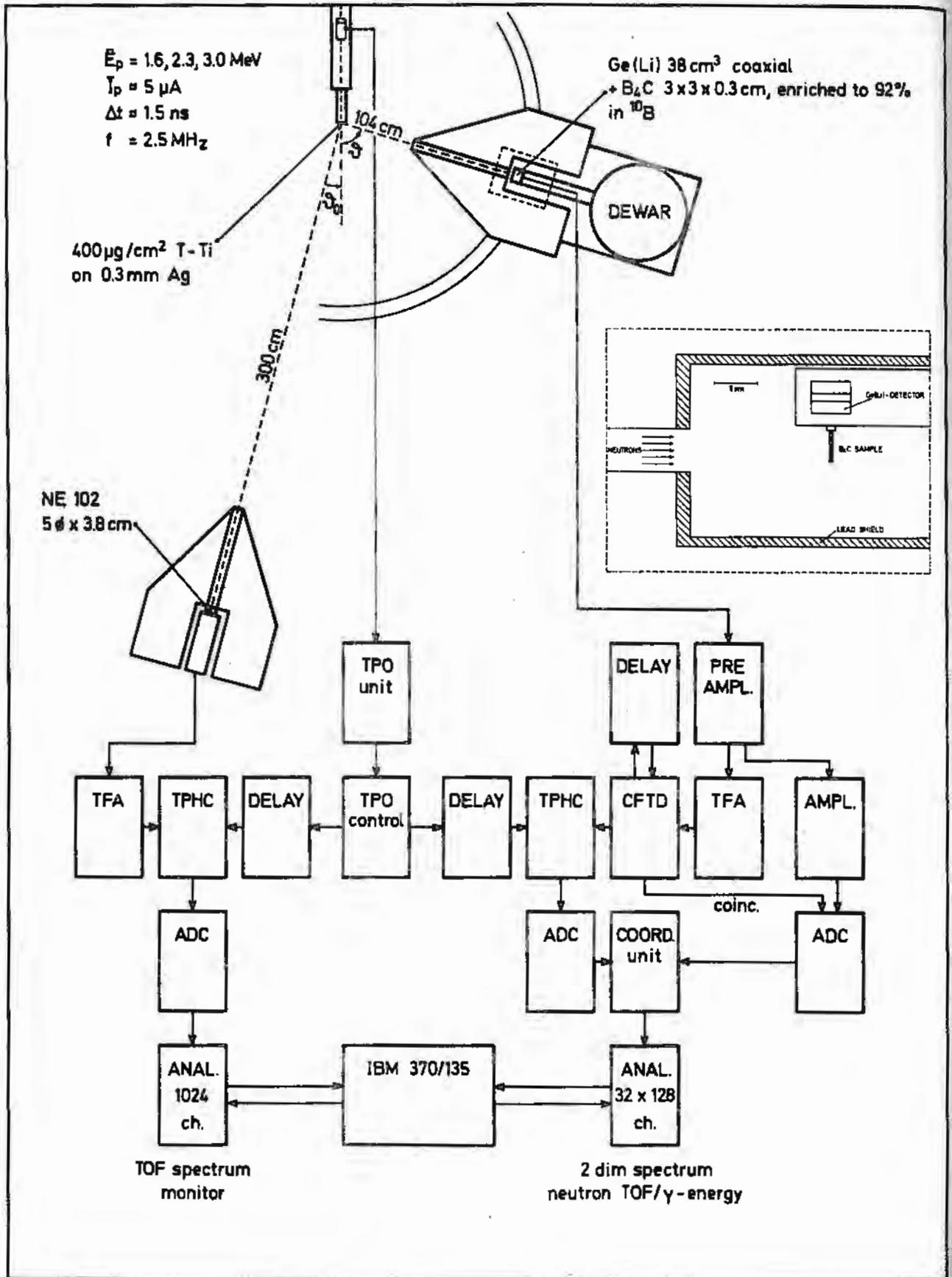
Fig. 3.6 Experimental arrangement for the measurement of the  $^{10}\text{B}(n, \alpha)^7\text{Li}$  cross section.
