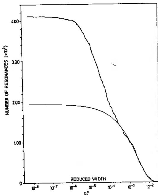
Fig. 2.11 Integral distribution of reduced neutron widths of  $^{238}\text{U}$  resonances.
