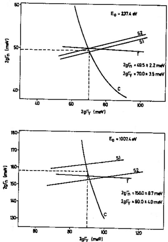
Fig.2.5 Examples of resonance parameter analysis for two resonances of  $^{129}\text{I}$ . The curves labelled C, T, S1 and S2 are from capture, transmission, self-indication (thin sample) and self-indication (thick sample) experiments respectively.
