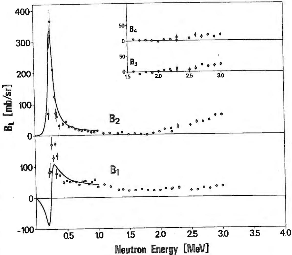
Fig. 3.2 Centre of mass legendre polynomial expansion coefficients of neutron elastic scattering angular distributions of  ${}^6\text{Li}$ . Solid lines are calculated curves.
