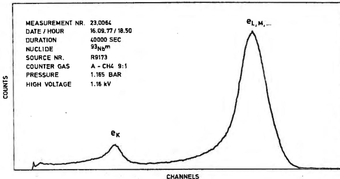
Fig.4.2 Spectrum of the K and LM+... conversion electrons of  $^{93}\text{Nb}^m$  measured with a proportional counter.
