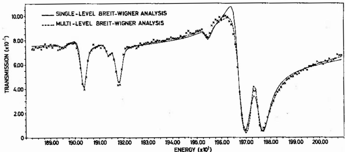
Fig.2.10 Comparison of single-level and multi-level Breit-Wigner analysis of neutron transmission through  $^{238}\text{U}$  in the neutron energy range 1880 eV to 2010 eV.
