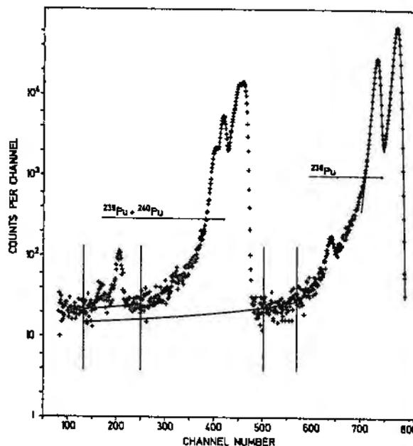
Fig. 4.4 Alpha ray spectrum of a Pu sample.
