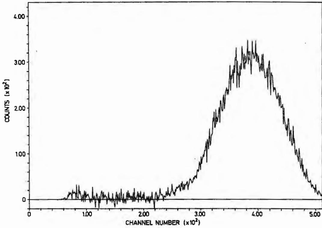
Fig.1.2 Experimental pulse height spectrum of scintillation detector observing recoil protons from polyethylen radiator foil.
